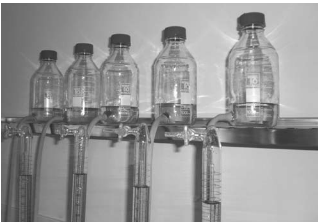
Fig. 3. Production of gas from various substrate samples
