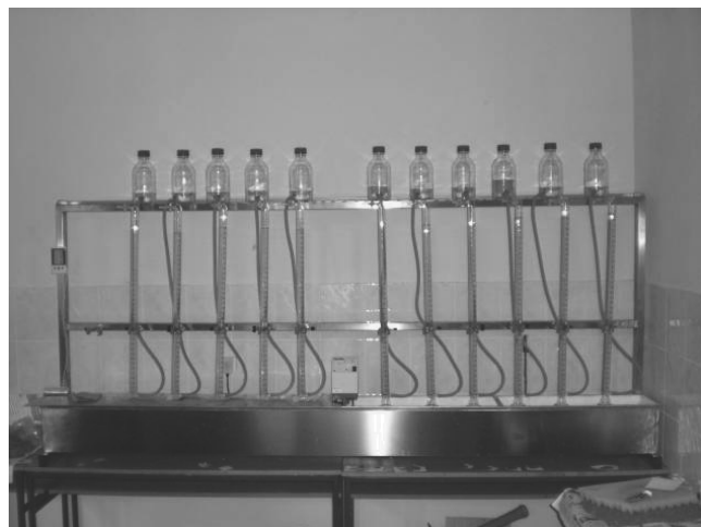
Fig. 5. Series of tests of biogas production
