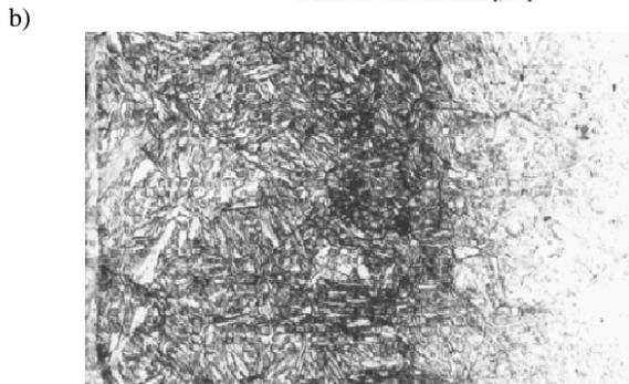
Fig. 23. The hardness profile – a), and microstructure of nitrided layer of X37CrMoV51 steel – b)
