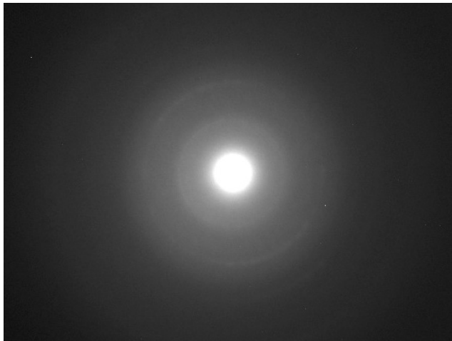
Fig. 3. Electron diffraction of thin DLC film
