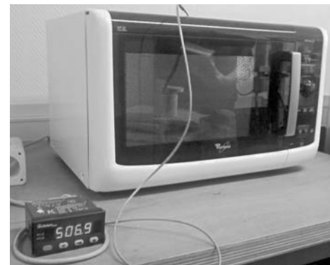
Fig. 2. Design of the safe box prepared for microwave sintering and using a house type microwave in laboratory conditions
