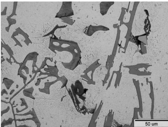
Fig. 5. a), b) Microstructure of ACAISi9Cu casting alloy
