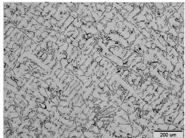
Fig. 7. Microstructure of ACAISi9Cu4 casting alloy
