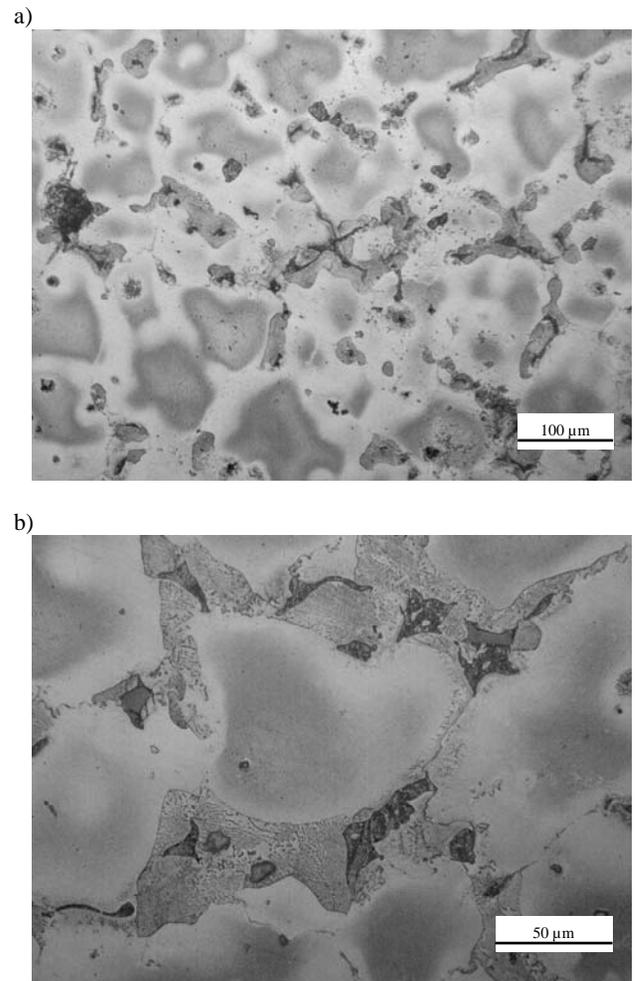
Fig. 2. a), b) Microstructure of MCMgAl6Zn1 magnesium alloys in as-cast state
