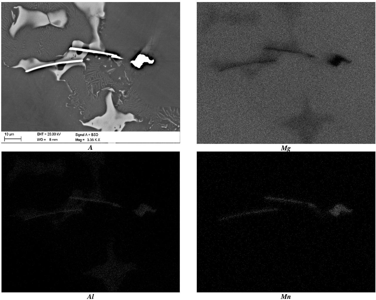
Fig. 4. The area analysis of chemical elements alloy MCMgAl6Zn1 in as-cast state: image of the secondary electrons (A) and maps of elements' distribution
