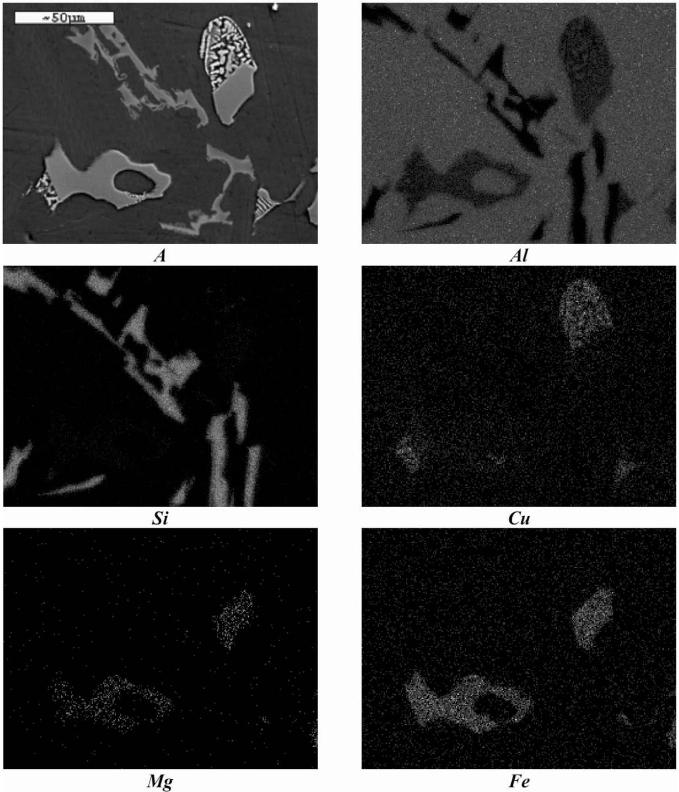
Fig. 8. The area analysis of chemical elements alloy ACA1Si9Cu4: image of secondary electrons (A) and maps of elements' distribution
