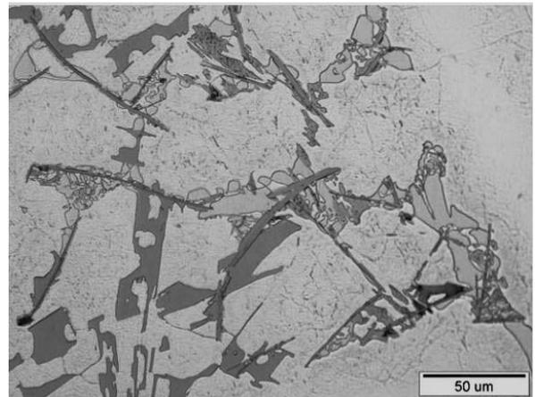
Fig. 6. Microstructure of ACAISi9Cu4 casting alloy
