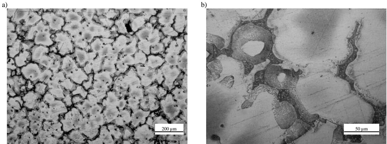
Fig. 3. a), b) Microstructure of MCMgAl9Zn1 magnesium alloys in as-cast state
