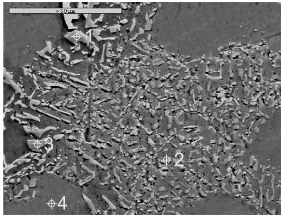
Fig. 9. Microstructure of ACAISi9Cu casting alloys
