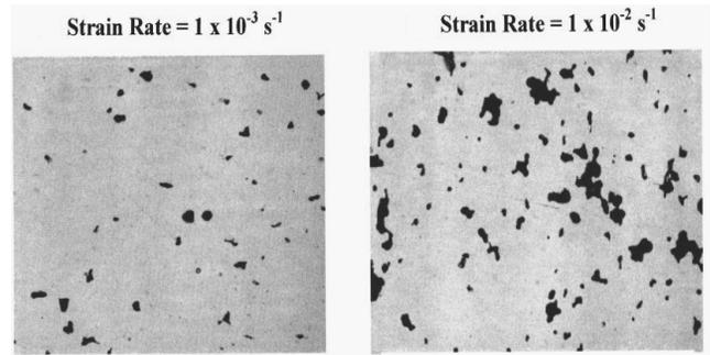
Fig. 5. Cavitation after Tensile Test on aluminium alloy specimens at fixed-temperature and different strain rate conditions
