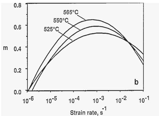
Fig. 3. Strain rate -  $m$  coefficient as the temperature change on experimental relation for Al5083 aluminium alloy
