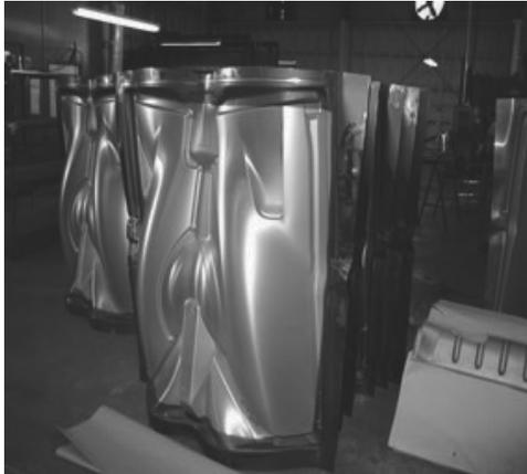
Fig. 1. Aerospace part realized with SPF
