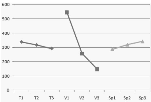
Fig. 14. Trend analysis of  $ft$  index over Temperature (T), Strain Rate (V) and Thickness (Sp)
