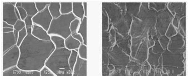
Fig. 2. Grains size change before and after SPF
