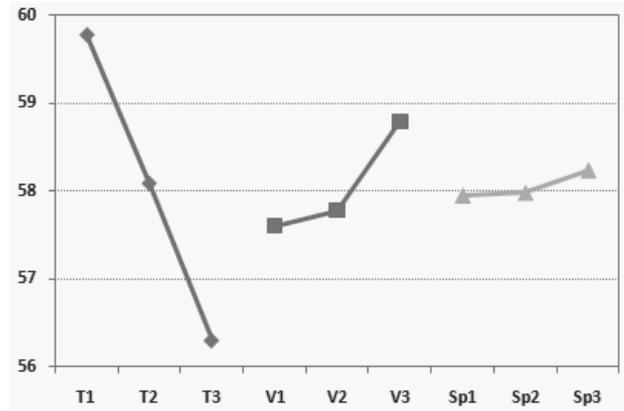
Fig. 9. Trend analysis of *mtp* index over Temperature (T), Strain Rate (V) and Thickness (Sp)
