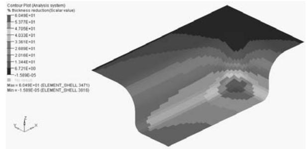
Fig. 7. Case T1Sp2V3: thickness reduction
