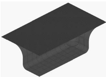
Fig. 6. FE model of a quarter of die and blank
