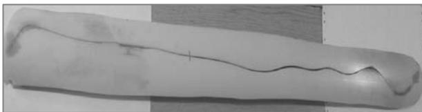
Fig. 6. Deformed fragment of the pipe: a) internal side of the wall of the tubular wire, b) the outside of the wall of the tubular wire
