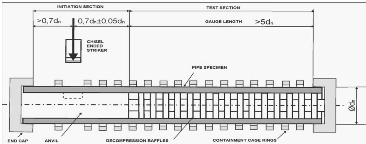
Fig. 2. Schematic view of the Small Scale Steady State (S4) test configuration [11]
