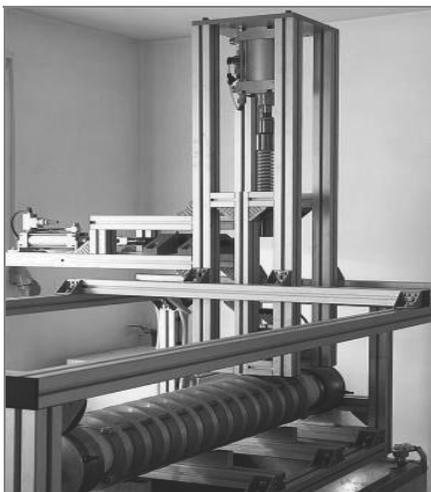
Fig. 3. Position to the Small Scale Steady State (S4) test in Oil and Gas Institute in Cracow
