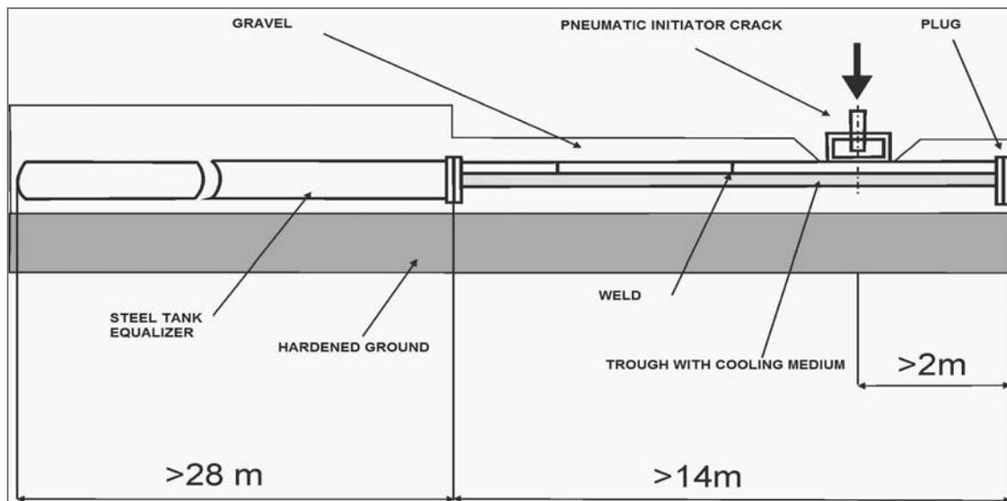
Fig. 1. Schematic view of the Full Scale Test configuration [11]
