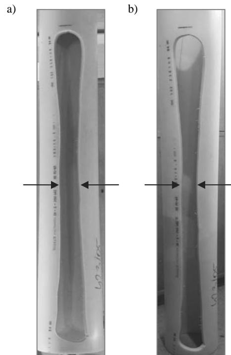
Fig. 8 . Deformed sample after the fragment has been cut; a) after 1 hour, b) after 2 weeks
