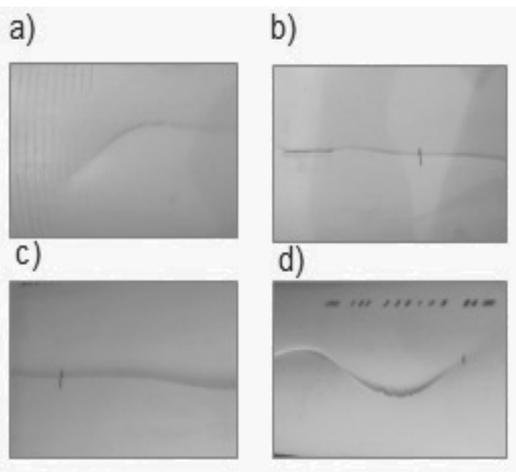
Fig. 7. Fragments of the sample depicting the course of the crack: a) beginning of the sample (closer side of the blade initiating the crack), b) fragment of it being struck by a blade, c) median part of the sample, d) end of the sample
