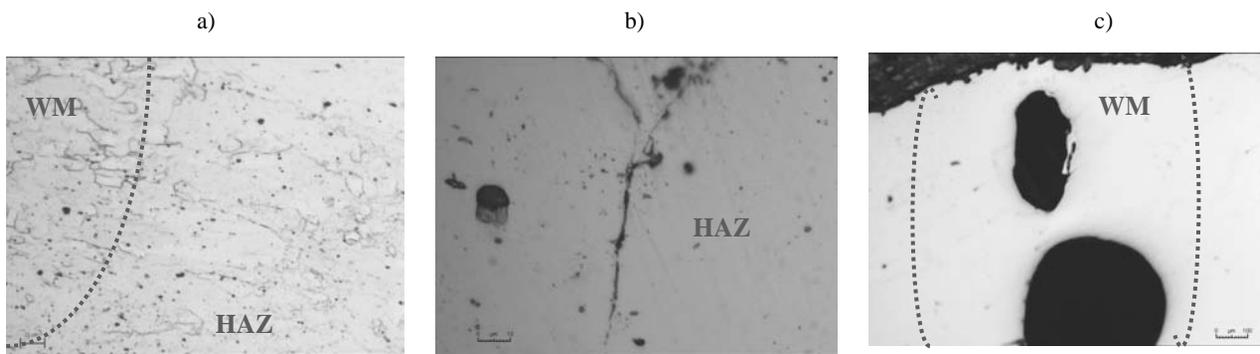
Fig. 5. Microstructure of the IF-NbB steel grade (LASER, weld bead and HAZ)
