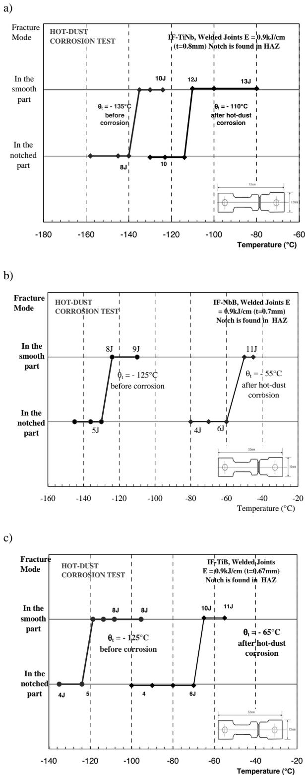
Fig. 8. Ductile-Brittle Transition Temperature (DBTT) of IFS-steel grades before and after hot/dust corrosion
