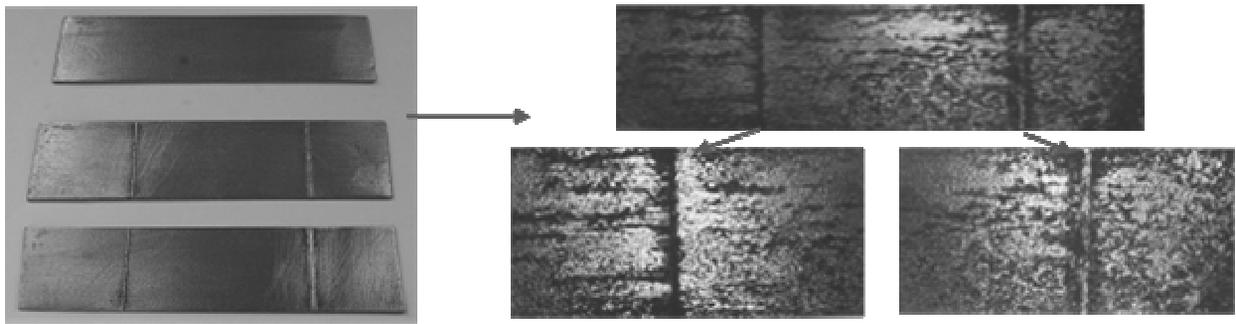
Fig. 4. IFS steel samples before and after the corrosion test
