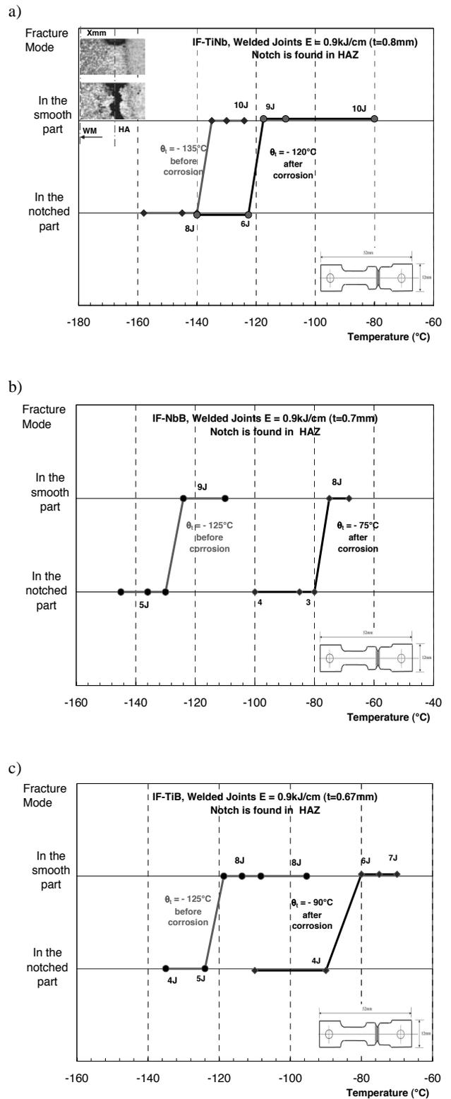
Fig. 7. Ductile-Brittle Transition Temperature (DBTT) of IFS-steel grades before and after wet/humidity corrosion
