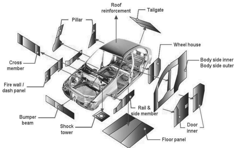
Fig. 1. General application of thin sheet steel as Tailored Welded Blanks (TWBs) in car industry [9]
