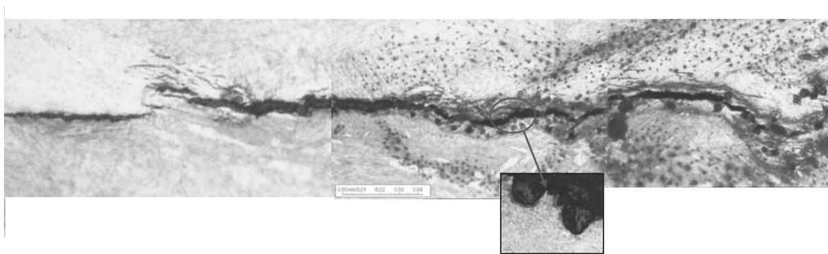
Fig. 6. Damage in the HAZ of the IF-NbB steel grade kept under the stress during the corrosion (RSW)
