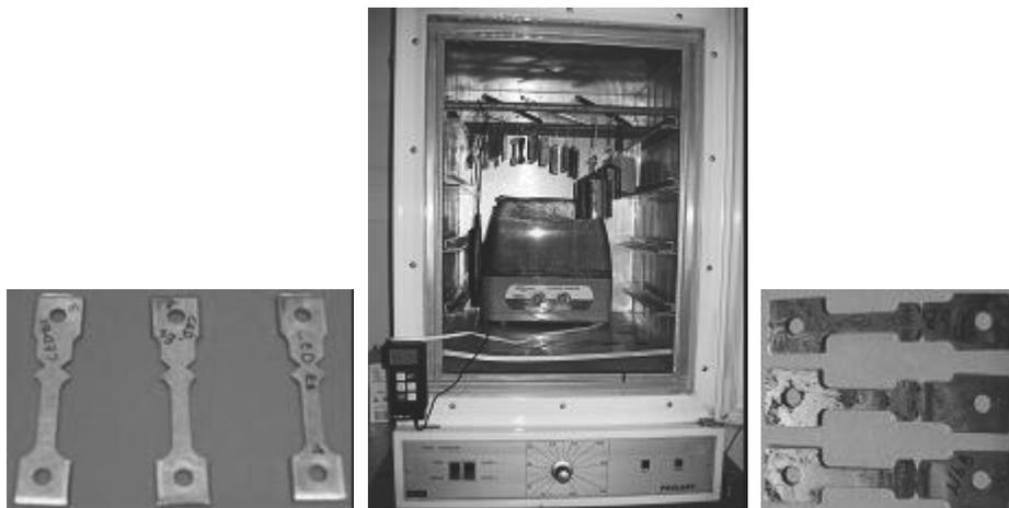
Fig. 3. Laboratory set up of corrosion (oven + specimen setting + hygrometer, etc.); Impact tensile-crash test specimens before and after the corrosion exposing cycle
