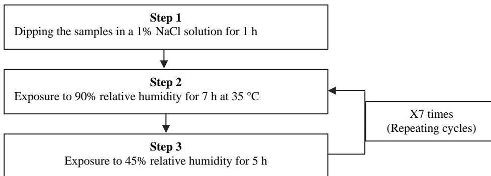
Fig. 2. Experimental procedure of (VOLVO) corrosion test
