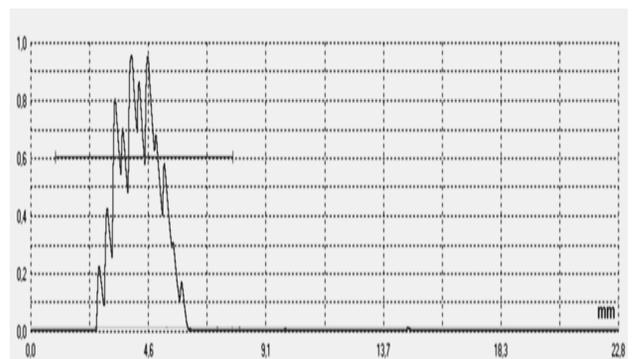
Fig. 6. Pulse image obtained from the 10mm diameter defect 3.25mm under the surface. Ultrasonic head was at the central position above the defect. (Amplification - 72.40 dB; Undercutting - 49, 46 %)
