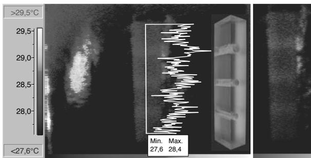
Fig. 13. The thermal image of polymethacrylate (methylate) specimen recorded one hundred fifty seconds from the end of pre-heating process
