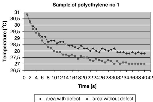
Fig. 9. The dependence of temperature on cooling time for areas with and without defect
