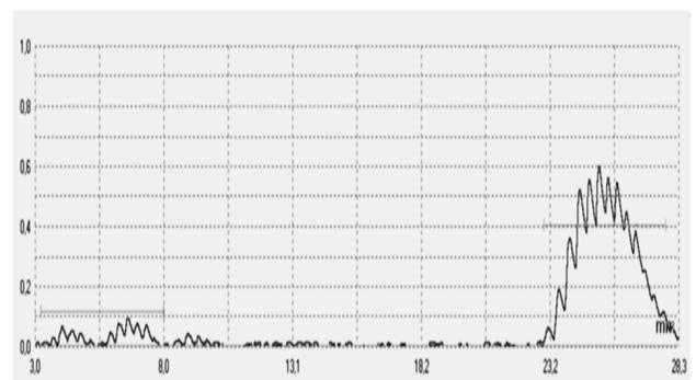
Fig. 16. Image of pulse reflected from the bottom of the laminate sample. (Amplification - 72.40 dB; Undercutting - 10, 12 %)
