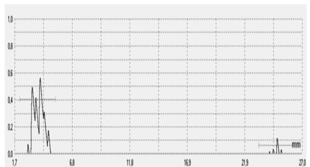
Fig. 11. Pulse image from the 10mm diameter defect at a depth of 3, 24 mm. Ultrasonic head was placed at the central position above the defect. (Amplification - 72.40 dB; Undercutting -72, 00 %)
