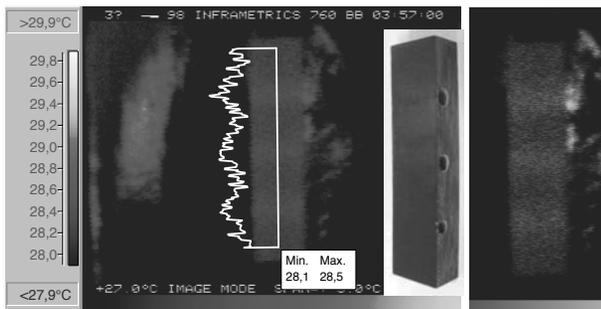
Fig. 18. The thermal image of laminate surface recorded one hundred and fifty seconds from the end of pre-heating process
