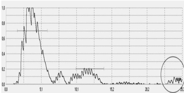
Fig. 17. Image of pulse reflected from the 4mm diameter defect being 2, 58 mm deep and reflected from the bottom of the laminate sample (in the circle). (Amplification - 72.40 dB; Undercutting - 10, 12 %)
