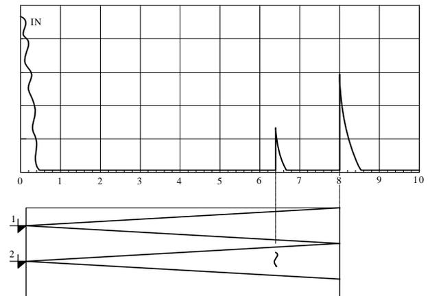
Fig. 1. Idea of the ultrasound pulse-echo testing method. The top image shows the flaw detector's screen. IN – trigger pulse. The bottom image shows the ultrasound wave passing through the material [19].
