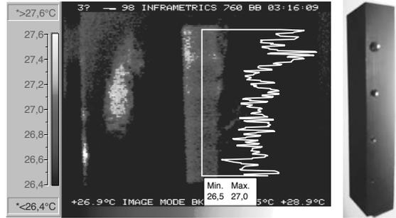
Fig. 10. The thermal image of polyethylene specimen registered sixty seconds after the end of pre-heating process
