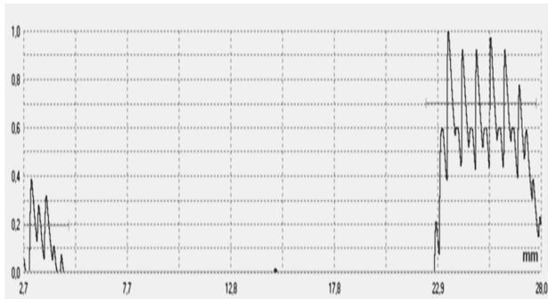
Fig. 12. Pulse image from the 2mm diameter defect at 2,99 mm deep. Ultrasonic head was placed at the central position above the defect. (Amplification - 72.40 dB; Undercutting -72, 00 %)
