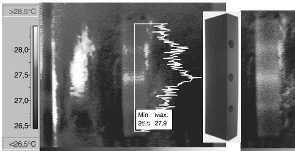
Fig. 8. The thermal image of polyethylene specimen registered ninety seconds after the end of pre-heating process
