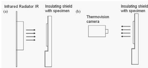
Fig. 4. Scheme of thermovision research stand: a) specimen pre-heating process, b) observing specimen's surface by a thermovision camera
