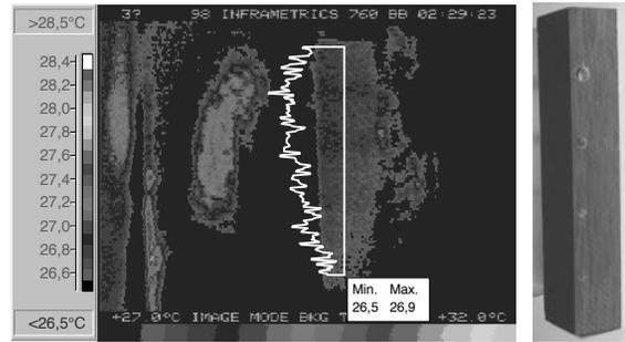
Fig. 20. The thermal image of laminate recorded sixty seconds from the end of pre-heating process
