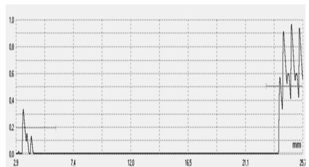
Fig. 7. Pulse images obtained from the 2mm diameter defect at 3.44 mm depth. Ultrasonic head was at the central position above the defect. (Amplification - 72.40 dB; Undercutting - 72, 17 %)
