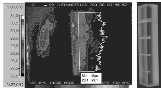
Fig. 15. The thermal image of polymethacrylate (methylate) recorded sixty seconds from the end of pre-heating process
