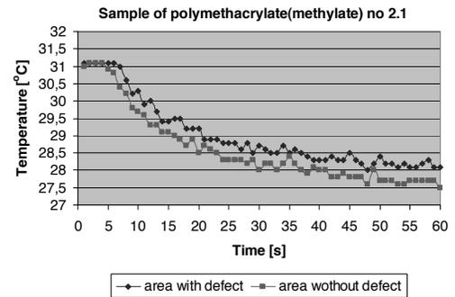
Fig. 14. The dependence of temperature on cooling time for the areas with and without defect
