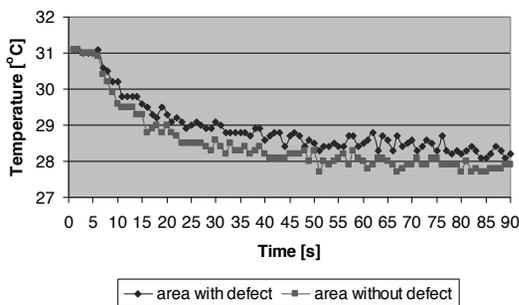
Fig. 19. The dependence of temperature on cooling time for the areas with and without defect
