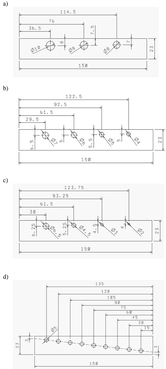
Fig. 3. Specimens and defects geometry: a) specimen with holes  $\Phi 10$ mm,  $\Phi 9$ mm and  $\Phi 8$ mm, b) specimen with holes  $\Phi 4 - \Phi 7$ mm, c) specimen with holes  $\Phi 2$ mm,  $\Phi 3$ mm,  $\Phi 4.5$ mm and  $\Phi 6.5$ mm, d) specimen with holes placed at different distances to surface
