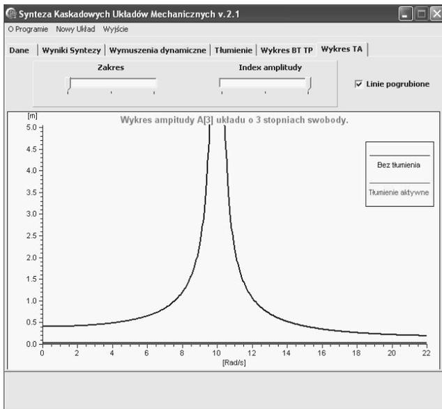
Fig. 19. Diagram of  $A_3$  amplitude and maximum displacement of system at  $\omega = 10 \frac{\text{rad}}{\text{s}}$
