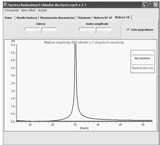
Fig. 17. Diagram of  $A_1$  amplitude and maximum displacement of system at  $\omega = 35 \frac{rad}{s}$
