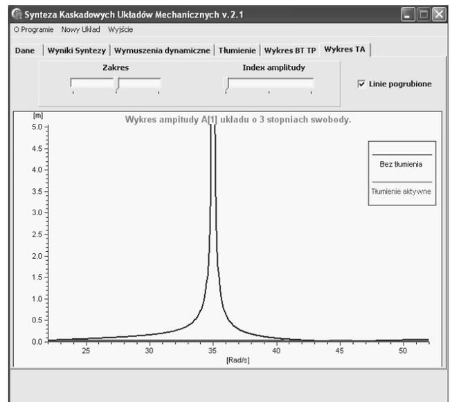
Fig. 14. Diagram of  $A_1$  amplitude and maximum displacement of system at  $\omega = 35 \frac{rad}{s}$
