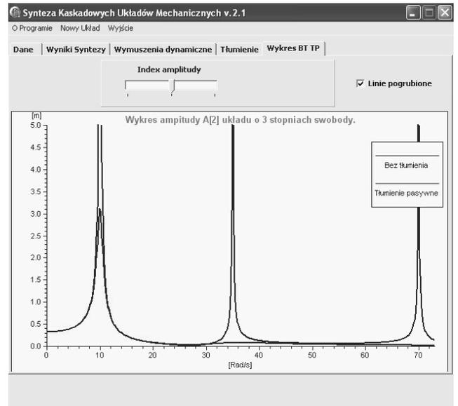
Fig. 10. Diagram of  $A_2$  amplitude and maximum displacement
