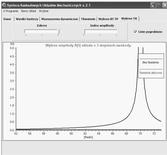
Fig. 15. Diagram of  $A_1$  amplitude and maximum displacement of system at  $\omega = 70 \frac{rad}{s}$
