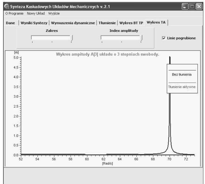
Fig. 21. Diagram of  $A_3$  amplitude and maximum displacement of system at  $\omega = 70 \frac{\text{rad}}{\text{s}}$
