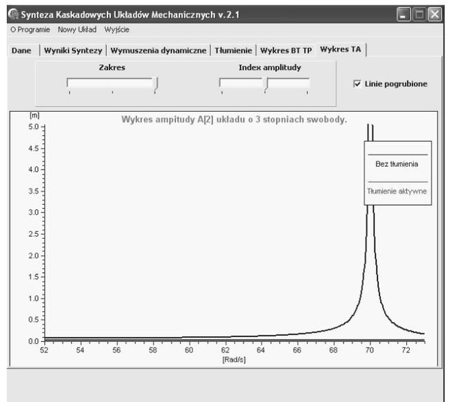
Fig. 18. Diagram of  $A_2$  amplitude and maximum displacement of system at  $\omega = 70 \frac{rad}{s}$
