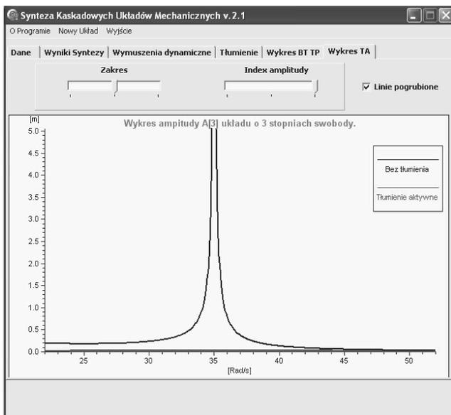
Fig. 20. Diagram of  $A_3$  amplitude and maximum displacement of system at  $\omega = 35 \frac{\text{rad}}{\text{s}}$
