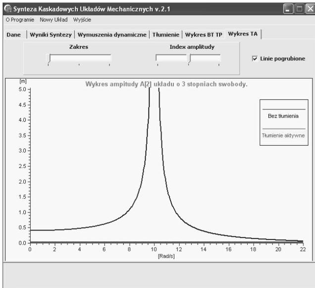
Fig. 16. Diagram of  $A_2$  amplitude and maximum displacement of system at  $\omega = 10 \frac{rad}{s}$
