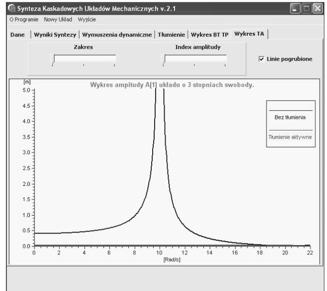
Fig. 13. Diagram of  $A_1$  amplitude and maximum displacement of system at  $\omega = 10 \frac{rad}{s}$
