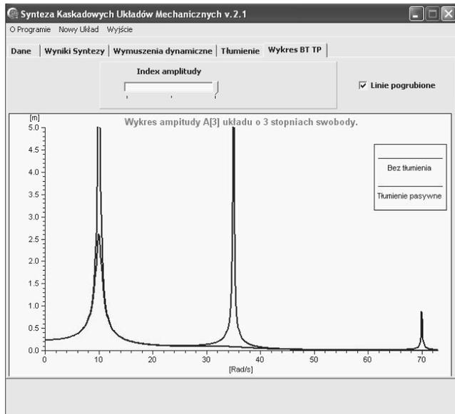
Fig. 11. Diagram of  $A_3$  amplitude and maximum displacement
