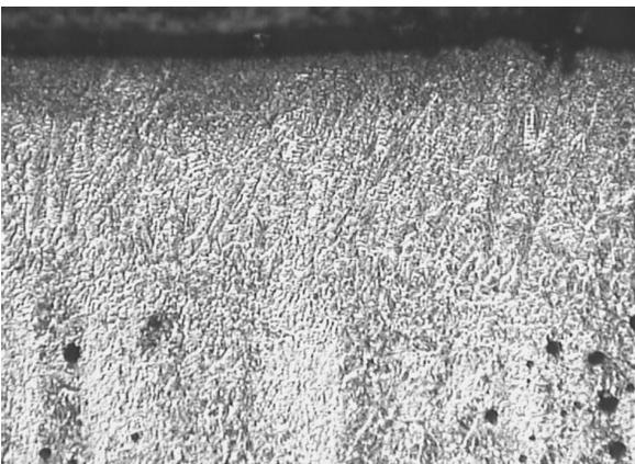
Fig. 10. Structure of the surface layer after remelting with  $\text{Al}_2\text{O}_3$  powder using 1.2 kW laser power
