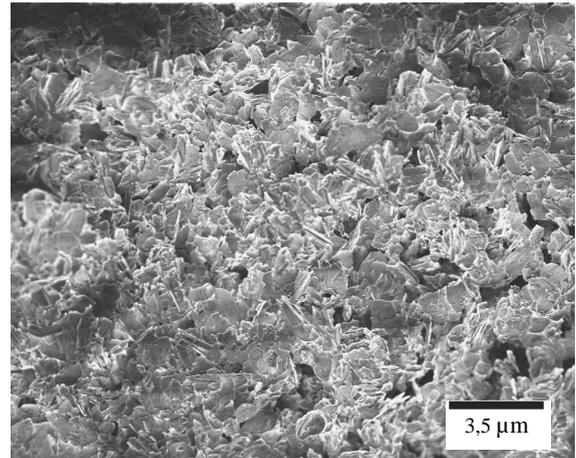
Fig. 4.  $ZrO_2$  powder used for alloying
