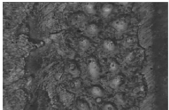
Fig. 7. Shape of the laser tray of the 32CrMoV12-28 steel remelted with ZrO<sub>2</sub> powder, laser power 1.2 kW
