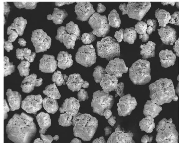
Fig. 5.  $Al_2O_3$  powder used for alloying
