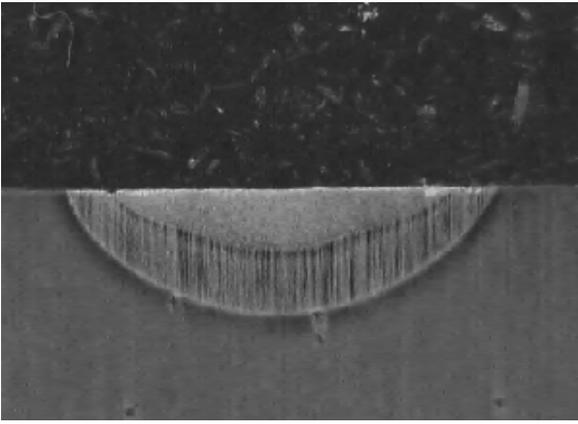
Fig. 8. Shape and thickness of cross-section of the laser remelted samples with  $\text{Al}_2\text{O}_3$  laser by power of 2.3 kW
