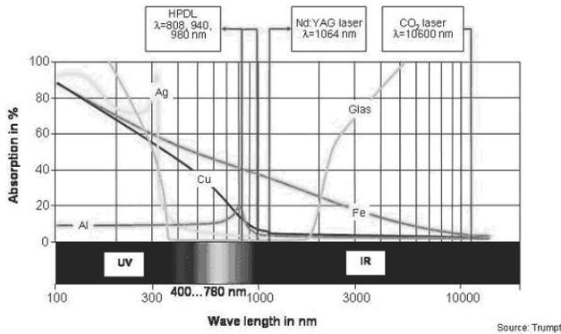
Fig. 1. Wave length range of the HPDL in comparison to Nd:Yag and CO<sub>2</sub> laser [Trumpf]
