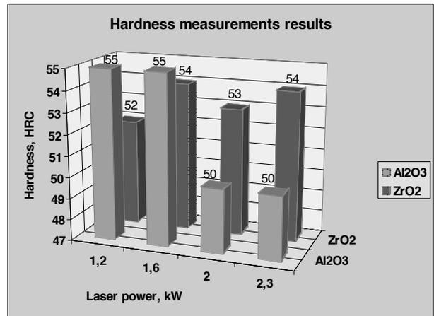
Fig. 15. Hardness measurements results of the Al<sub>2</sub>O<sub>3</sub> and ZrO<sub>2</sub> alloyed steel
