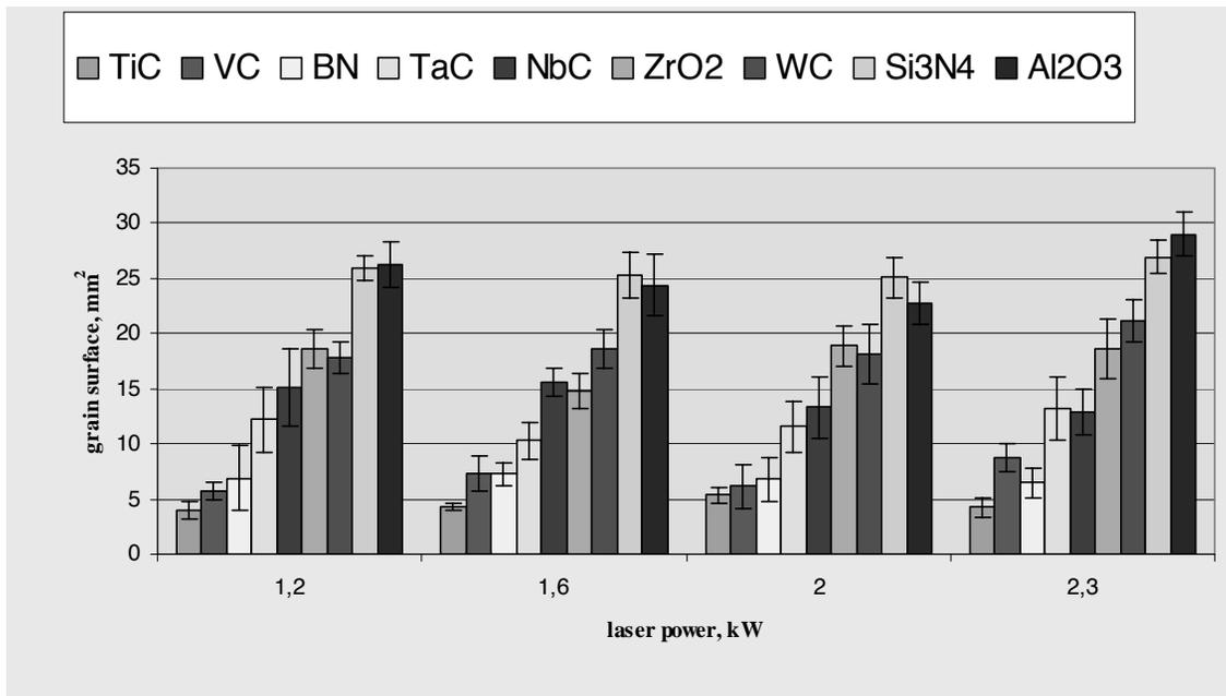
Fig. 16. Average grain surface area of the remelted zone SP of the 32CrMoV12-28 steel alloyed with ceramic powders wit laser power in the range of 1.2 to 2.3 kW
