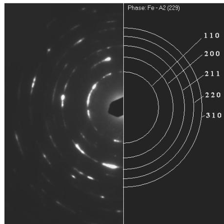
Fig. 11. TEM microstructure, a) bright field image, b) dark field image, c) diffraction pattern and its solution of the area in Fig. 13a
