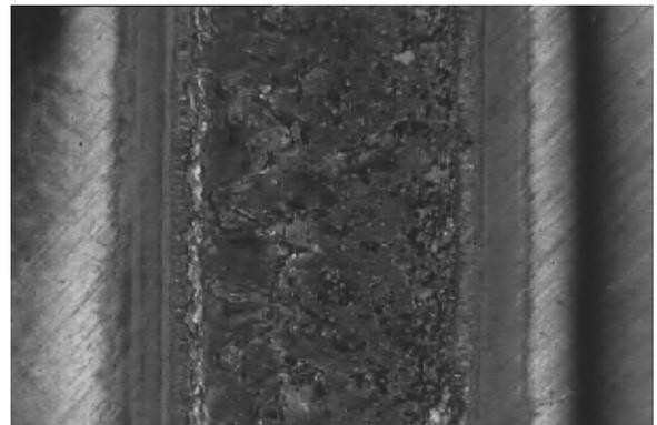
Fig. 6. Shape of the laser tray of the 32CrMoV12-28 steel remelted with Al<sub>2</sub>O<sub>3</sub> powder, laser power 2.3kW
