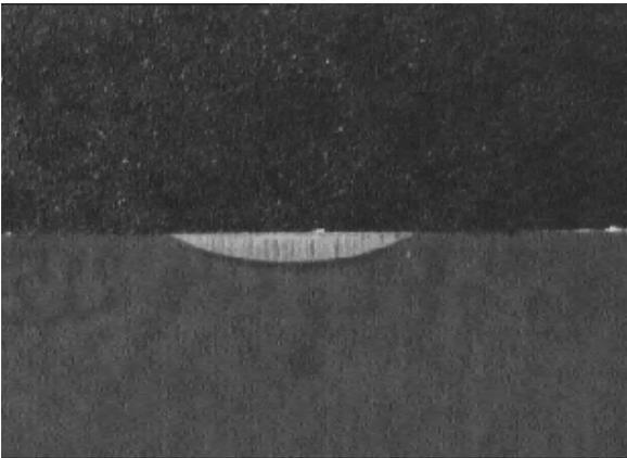
Fig. 9. Shape and thickness of cross-section of the laser remelted samples with  $\text{ZrO}_2$  laser by power of 1.2 kW
