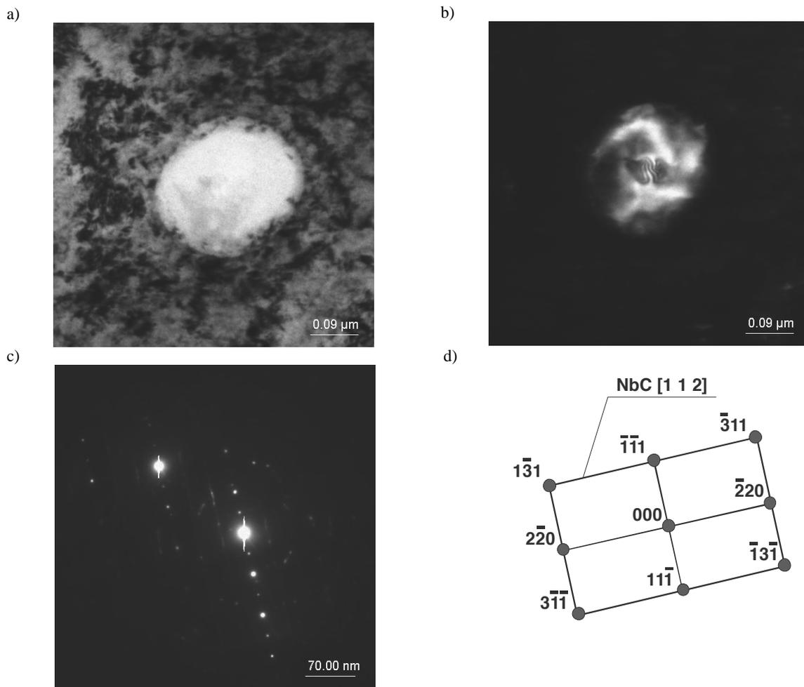
Fig. 12. TEM microstructure, a) bright field image, b) dark field image, c) diffraction pattern of the particle in Fig. 2a, solution of the diffraction pattern in Fig. 2c, high resolution image
