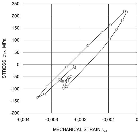
Fig. 15. Stress-strain characteristic in the selected point of T-pipe in the period of time: 6540 s - 8220 s
