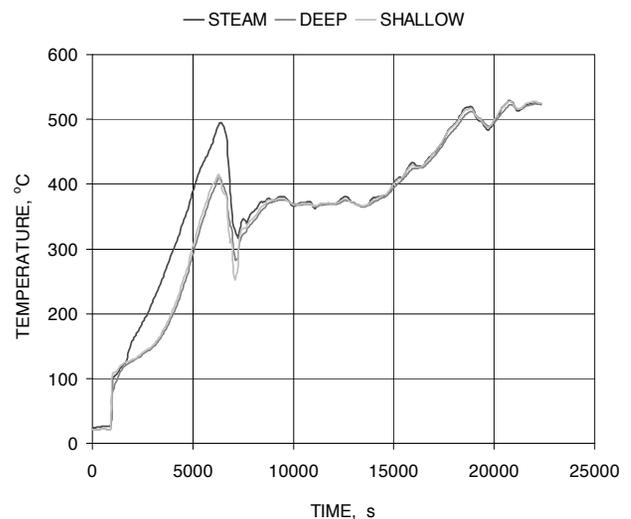
Fig. 2. Measurement results of steam temperature close to the boiler and of metal temperature in selected points of the T-pipe
