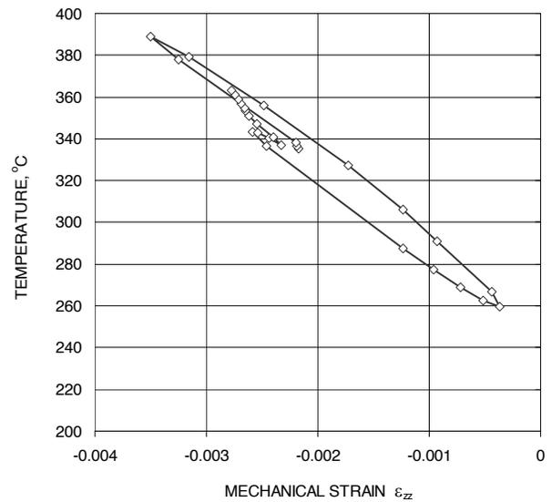
Fig. 16. Mechanical strain - temperature characteristic in the selected point of T-pipe in the period of time: 6540 s - 8220 s
