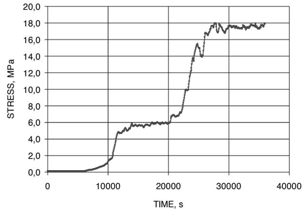
Fig. 7. Graph of pressure changes as a function of time during the boiler start-up
