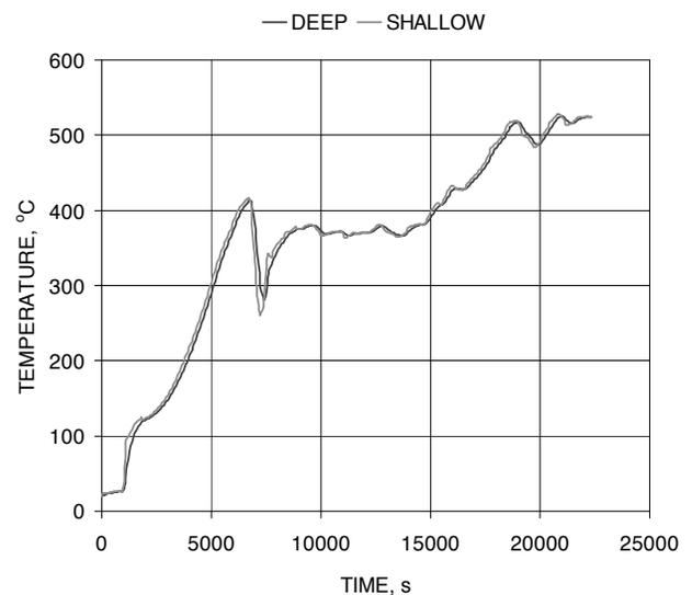
Fig. 4. Results of checking the correctness of the T-pipe model functioning: a diagram illustrating changes in time temperature, determined, using a computer model, in the same places (deep and shallow) as sensors
