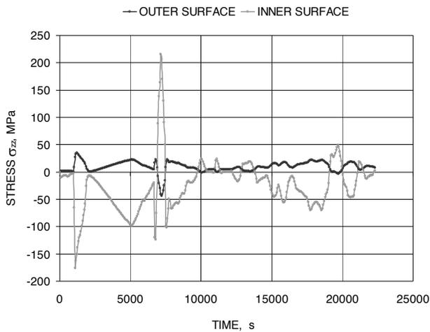
Fig. 14. Diagrams of changes over time of stresses  $\sigma_{zz}$  in the T-pipe in selected points of its inner and outer surfaces - the T-pipe with thick wall (Figs. 9, 10)
