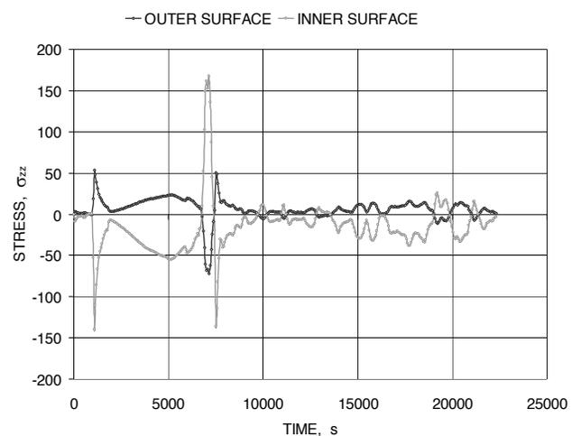
Fig. 13. Diagrams of changes over time of stresses  $\sigma_{zz}$  in the T-pipe in selected points of its inner and outer surfaces - the T-pipe with thin wall (Figs. 1, 6, 8)
