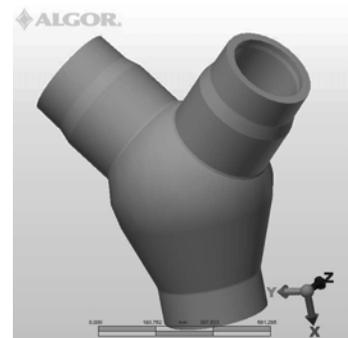
Fig. 1. Model of the main steam pipeline T-pipe
