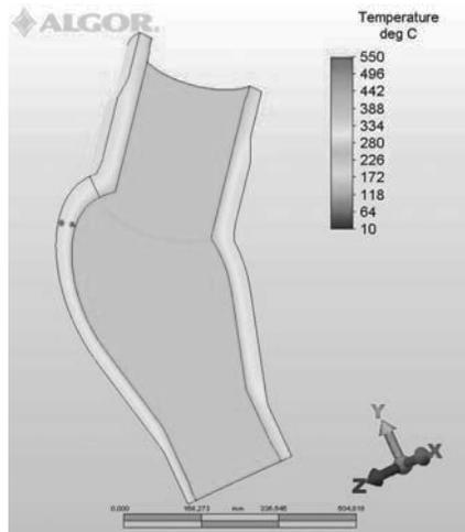
Fig. 6. Temperature distributions in the thin T-pipe with the lower value of thickness in selected instant of time:  $t=7200$  s
