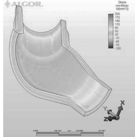
Fig. 8. Distributions of equivalent stresses in the T-pipe with the lower value of thickness in a moment of time:  $t=7200$  s from the start-up beginning
