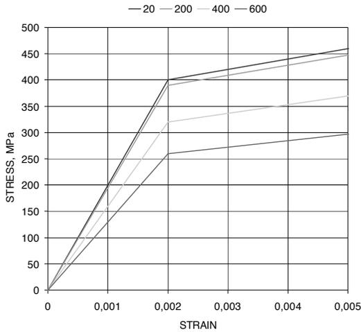
Fig. 5. Stress-strain characteristics of thermo-elastic-plastic model of material
