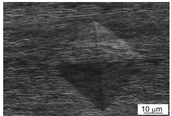
Fig. 13. Scanning microscopy image corresponding to deformation \varphi = 8.4 , by 20 CEC cycles and hydrostatic extrusion ( \varphi = 1.8 )
