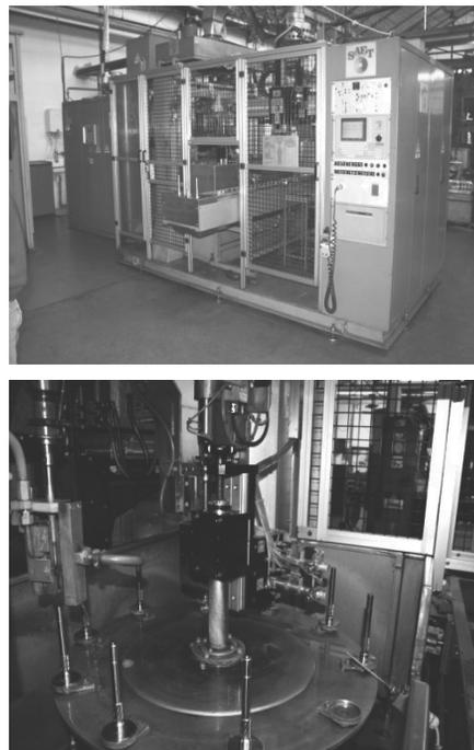
Fig. 2. The spin case-hardening device 3KTC (above). Inductor and manipulation system detail (below)
