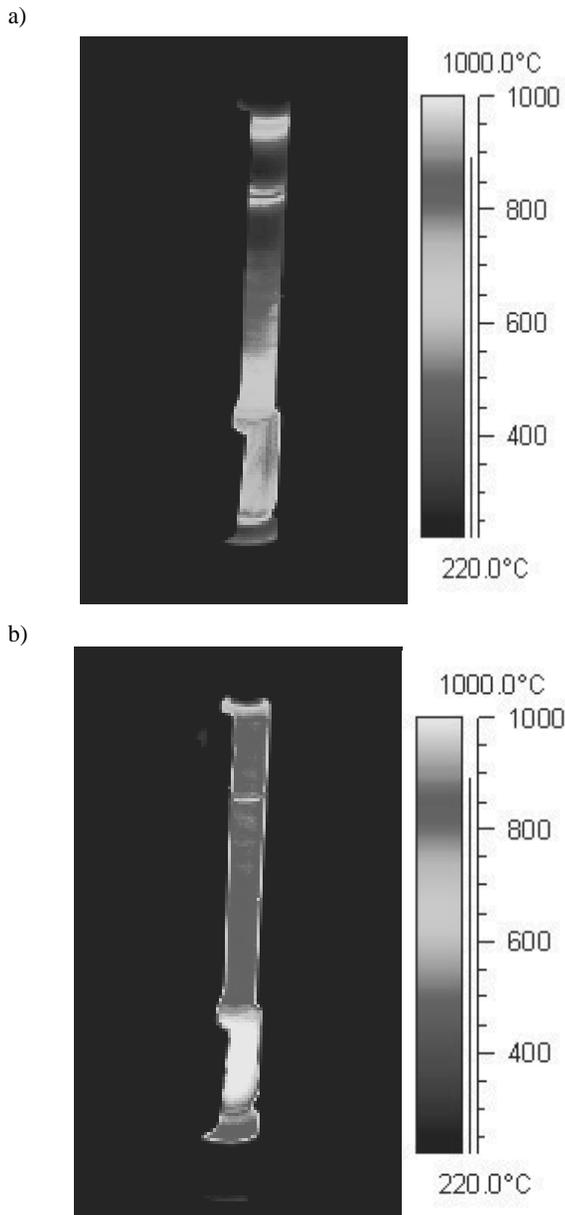
Fig. 5. Thermograph records: a) At the beginning of induction heating (0.5 sec). b) At the end of induction heating (2.5 sec)
