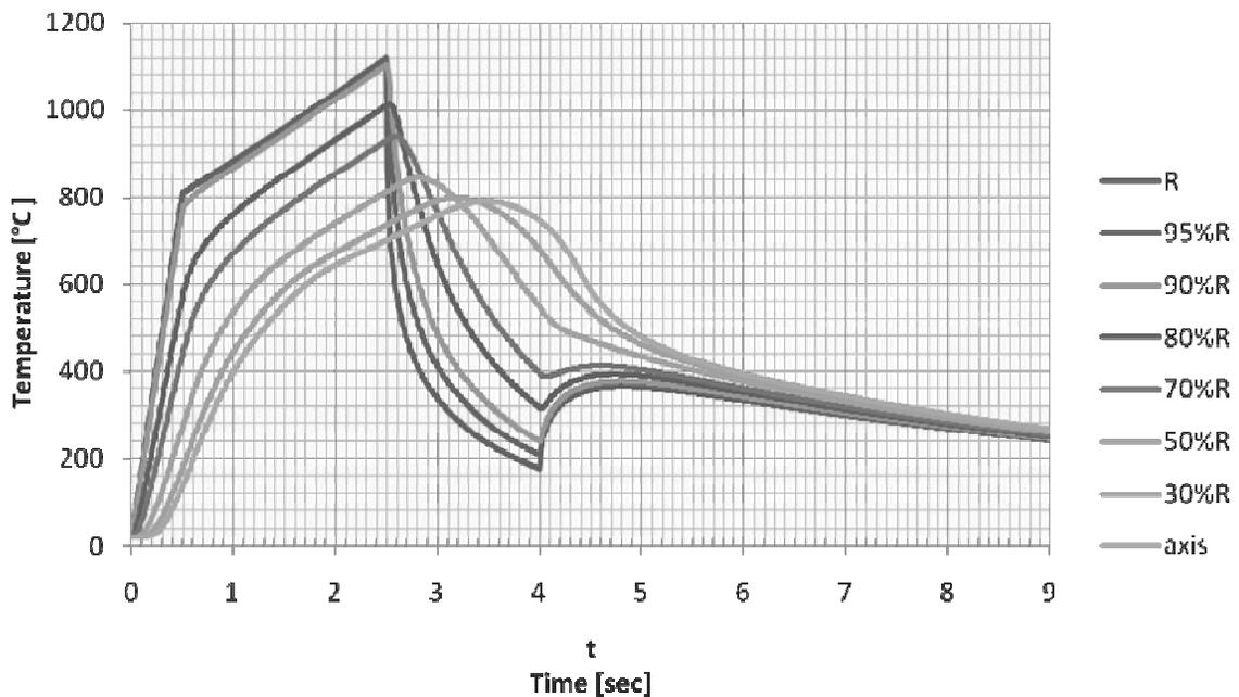
Fig. 6. Calculated temperature field in planetary shaft during induction hardening process ( $h_{tc} = 35000 \text{ W/m}^2\text{K}$ )
