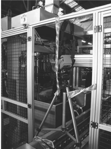
Fig. 3. Thermographic camera ThermoCAM PM675
