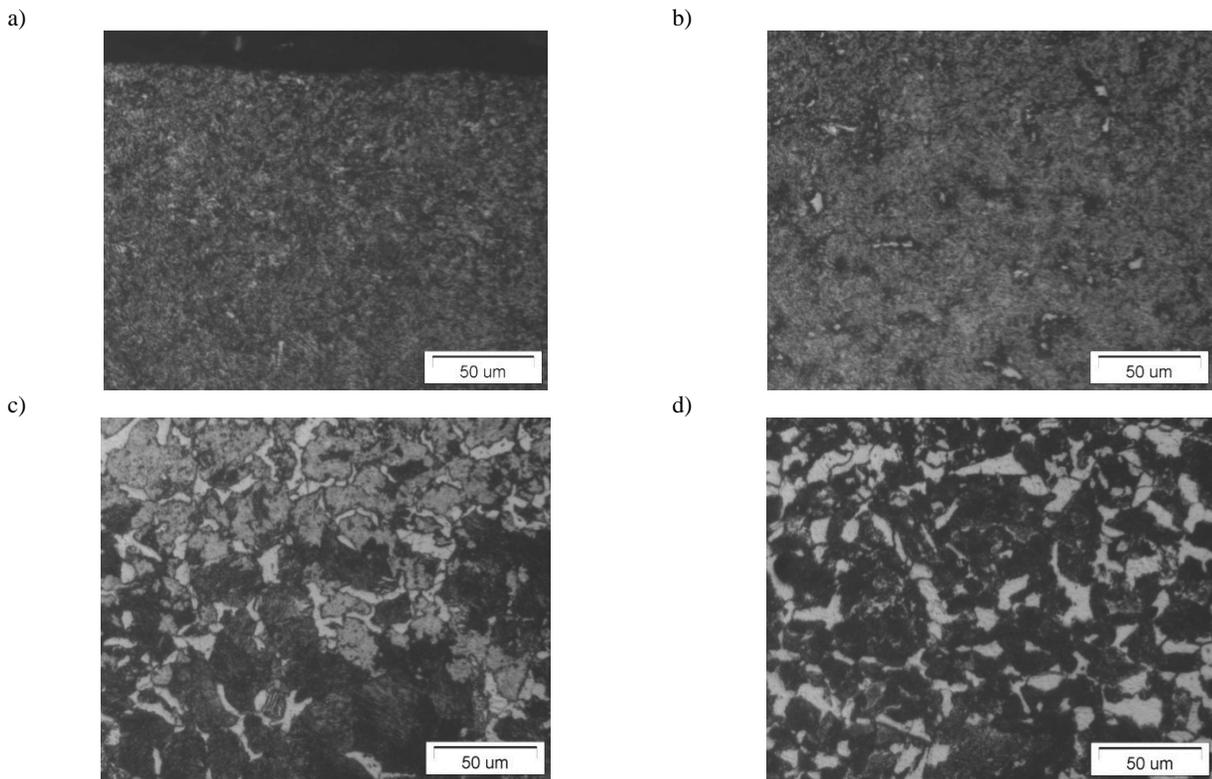
Fig. 9. Steel microstructures at different depths under the surface: a) surface; b) 0.7 mm; c) 1.4 mm; d) 2.1 mm
