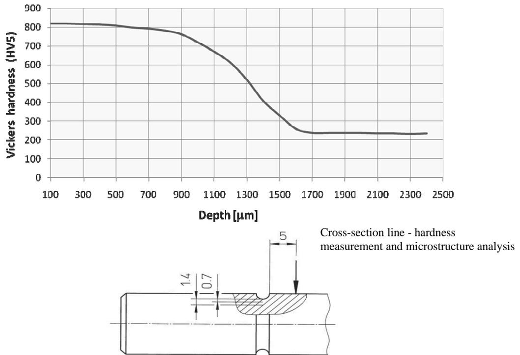
Fig. 8. Hardness course measured over the hardened case of the planetary shaft (above) and cross section line (below)
