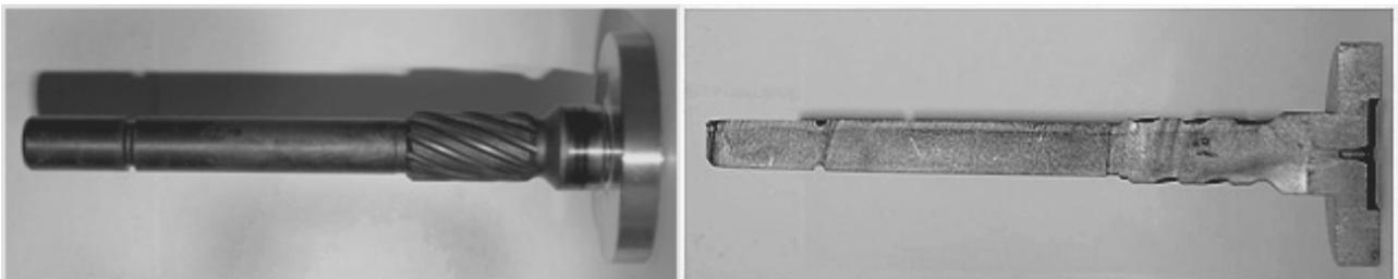
Fig. 7. Heat treated shaft (left). Longitudinal cross-section of the planetary shaft (right). Cutting was made with water jet cutting machine. Thickness of hardened case is approximately 1.4 mm
