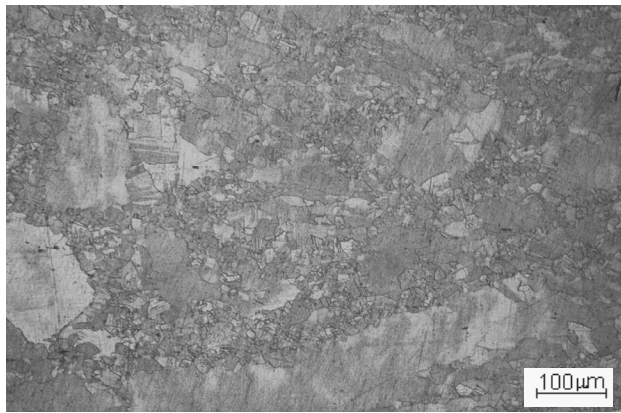
Fig. 17. The microstructure of brass CuZn30 after cold-rolling and recrystallization. Differentiated sizes of the \alpha grains in the solution ( z = 15.8\% , t_r = 400^\circ\text{C} )
