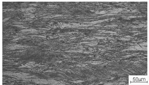
Fig. 15. The microstructure of brass CuZn30 after cold-rolling. Elongated \alpha grains in the solution with parallel slip bands ( z = 42.5\% ).
