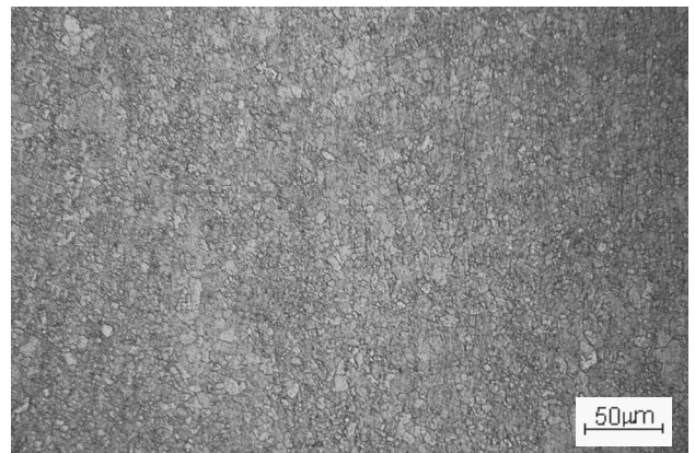
Fig. 21. Small recrystallized grains in the solution ( z = 56.2\% , t_r = 400^\circ\text{C} )
