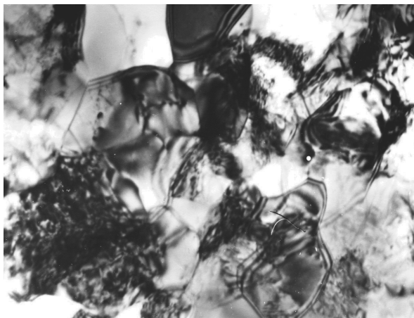
Fig. 16. Substructure of the sample after 4 ECAP passes
