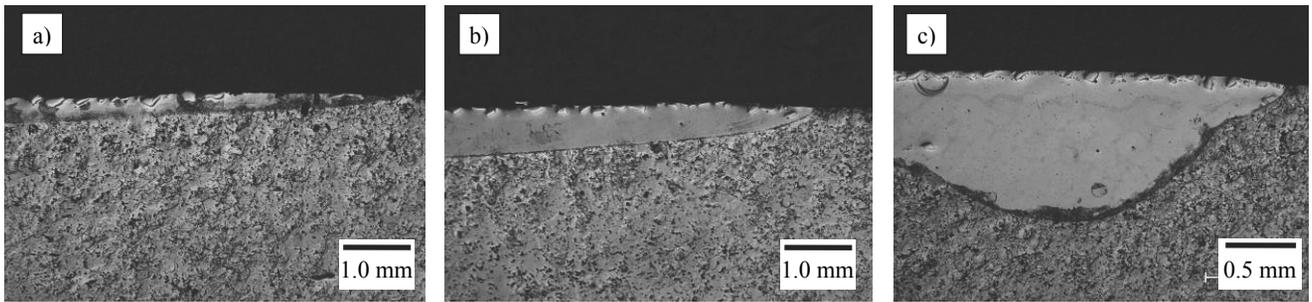
Fig. 4. The cross section of chromium laser alloyed 316L sintered stainless steel at increasing from a) to c) the laser beam power and powder feed rate, respectively: a) 0.7kW and 1.5g/min, b) 1.4kW and 2.0g/min and c) 2.0kW and 4.5g/min
