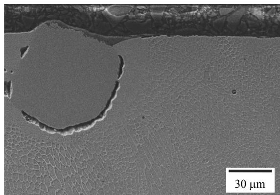
Fig. 16. The chromium powder particle embedded on the surface of 316L stainless steel alloyed at laser beam power of 1.4kW and powder feed rate of 1.0g/min
