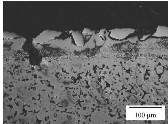
Fig. 8. The edge zone of 316L laser alloyed with Cr at laser beam power 1.4kW and powder feed rate of 2.0g/min
