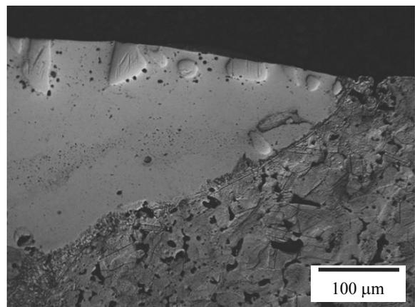
Fig. 10. The edge zone of 316L laser alloyed with Cr at laser beam power 2.0kW and powder feed rate of 4.5g/min
