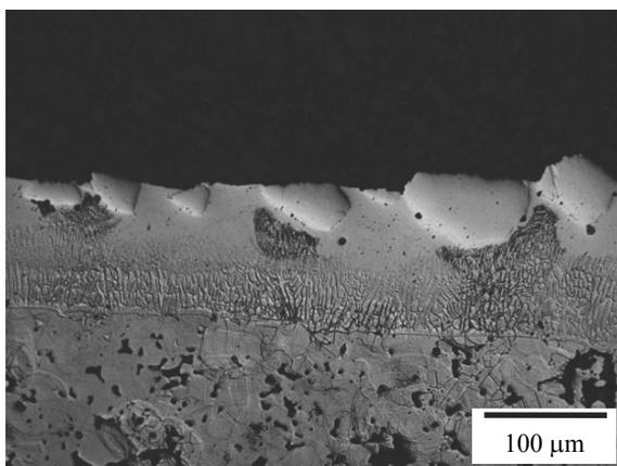
Fig. 7. The edge zone of 316L laser alloyed with Cr at laser beam power 0.7kW and powder feed rate of 1.5g/min
