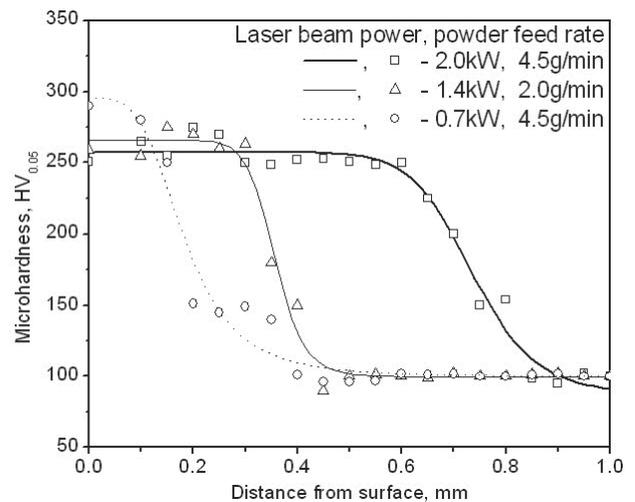
Fig. 13. Microhardness depth profile of sintered 316L after laser alloying with Cr at different laser conditions of laser beam power powder feed rate
