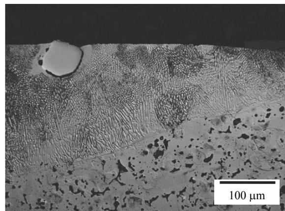
Fig. 9. The edge zone of 316L laser alloyed with Cr at laser beam power 1.4kW and powder feed rate of 1.0g/min
