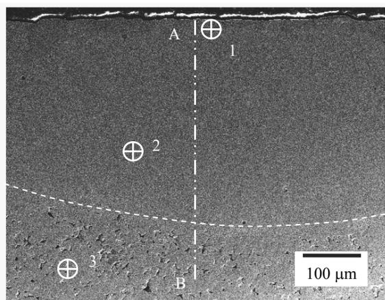
Fig. 14. The cross-section of laser surface alloyed 316L at 1.4kW of laser beam power and powder feed rate 2.0g/min. The dashed line represents the interface between remelted zone and base metal
