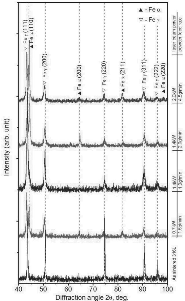
Fig. 6. The x-ray diffraction patterns of laser surface alloyed and as sintered stainless steel 316L
