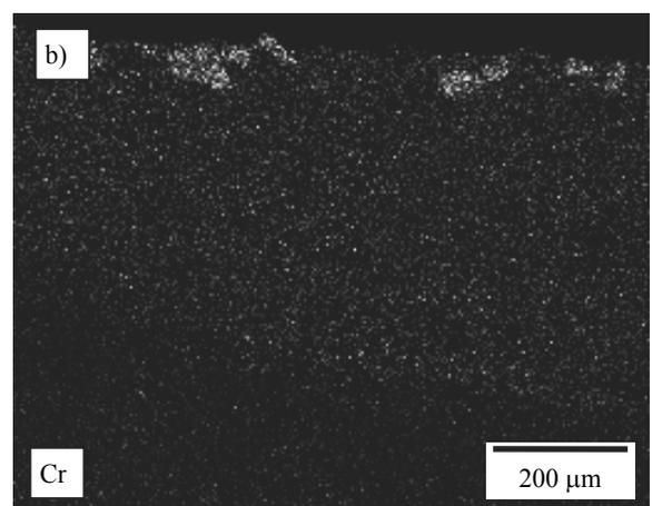
Fig. 17. The image of laser alloyed 316L at laser beam power of 1.4kW and powder feed rate of 2.0g/min, a) SE-image of cross section and b) the map of chromium distribution
