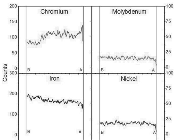
Fig. 15. The liner distribution of chemical composition along dash-dot line according to Fig. 14 on the cross section of Cr alloyed surface of 316L
