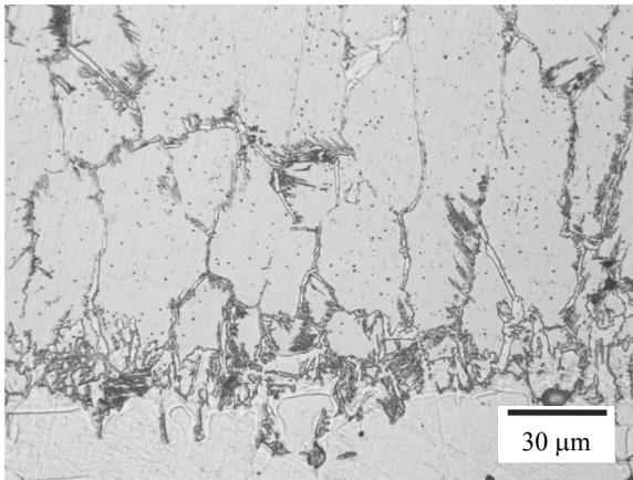
Fig. 11. The interface between alloyed zone (top), transient and base metal of 316L laser alloyed with Cr at laser beam power 2.0kW and powder feed rate of 4.5g/min
