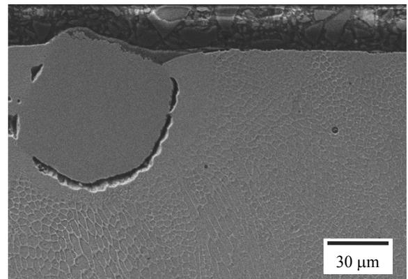
Fig. 16. The chromium powder particle embedded on the surface of 316L stainless steel alloyed at laser beam power of 1.4kW and powder feed rate of 1.0g/min
