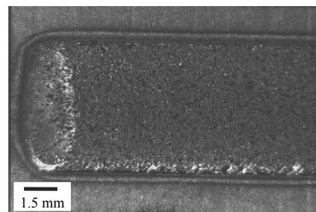
Fig. 3. The surface view of sintered 316L after laser alloying with Cr at laser beam power of 1.4kW and powder feed rate of 2.0g/min
