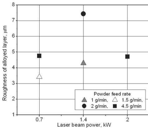
Fig. 5. The surface roughness of 316L sintered stainless steel after laser surface alloying
