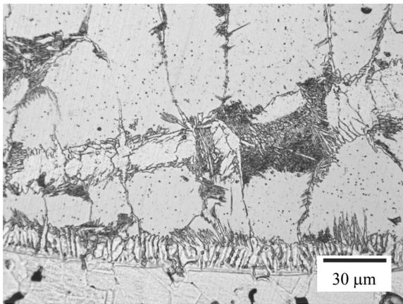
Fig. 12. The central zone of 316L laser alloyed with Cr at laser beam power 2.0kW and powder feed rate of 4.5g/min
