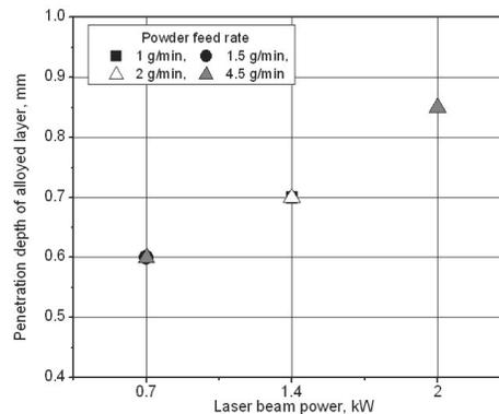
Fig. 2. The penetration depth of Cr alloyed surface layer of the 316L sintered austenitic stainless steel
