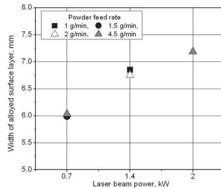
Fig. 1. The width of Cr alloyed surface layer of the sintered austenitic stainless steel 316L
