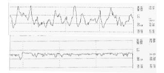
Fig. 5. Surface profile (before and after burnishing)
