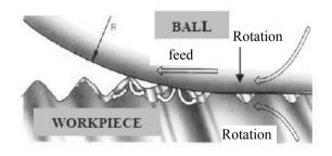
Fig. 1. Scheme of roller burnishing process [4]
