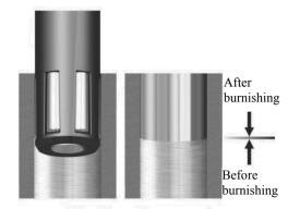
Fig. 2. Surface before and after roller burnishing [16]
