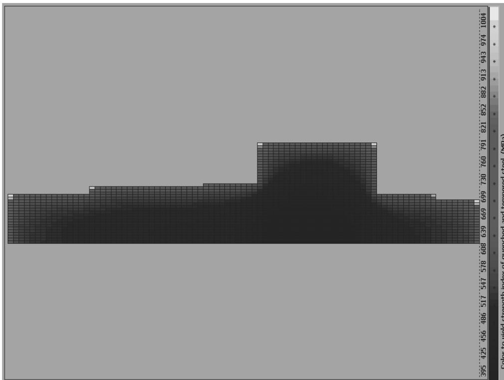
Fig. 4. Yield strength distribution in the quenched and tempered steel shaft
