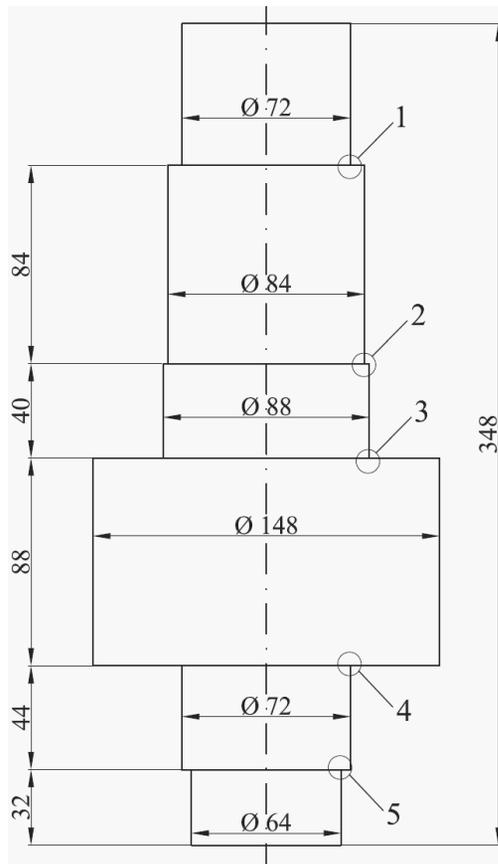
Fig. 1. Geometry of steel shaft
