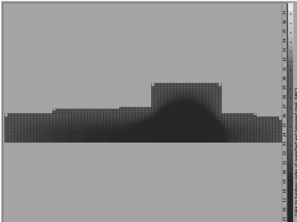
Fig. 3. Hardness distribution in the quenched and tempered steel shaft
