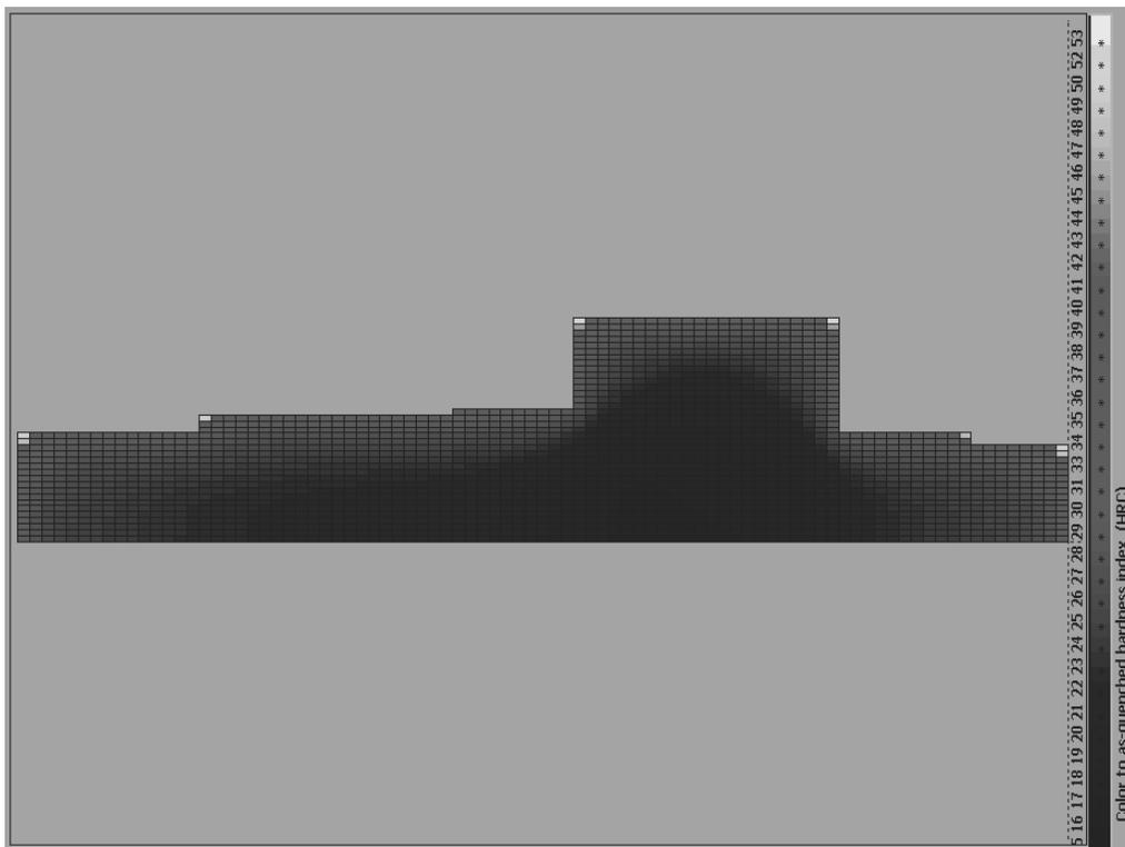
Fig. 2. Distributions of as-quenched hardness
