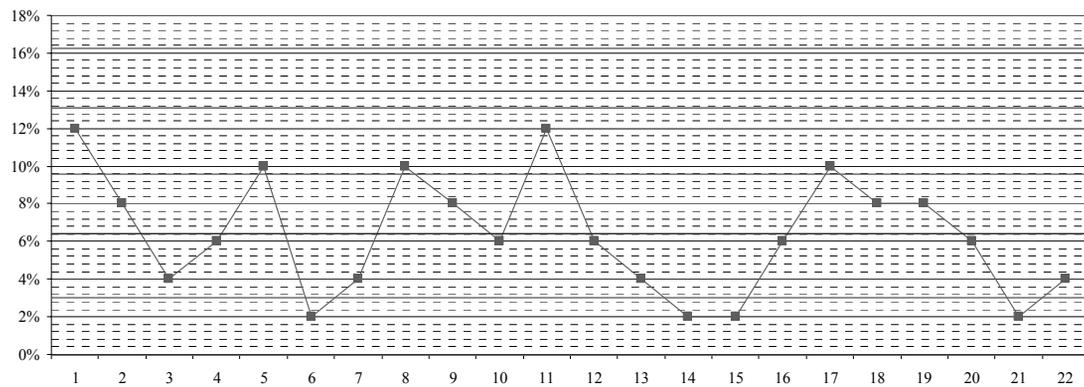
Fig. 3. p - chart - after the corrective actions were taken; x-axis- working days during one month
