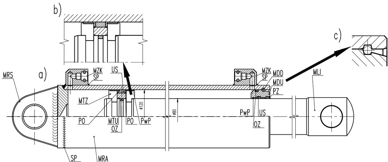
Fig. 4. Hydraulic actuator design generated with use of modular system program [5, 8]
