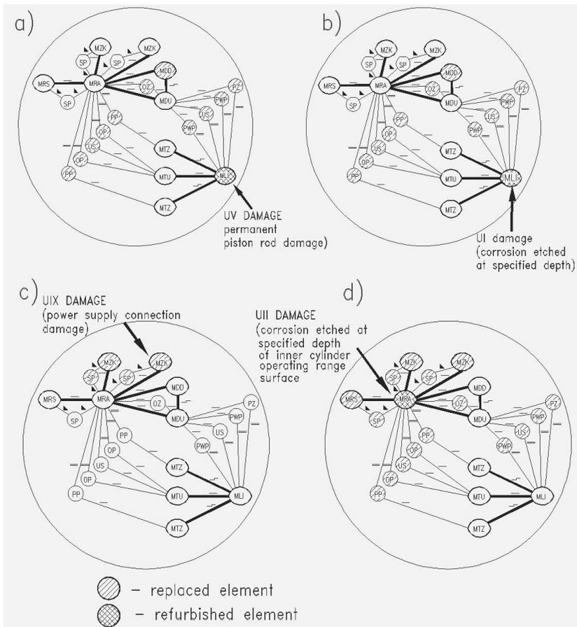
Fig. 8. Relations between damage type and element replacement or refurbishing model
