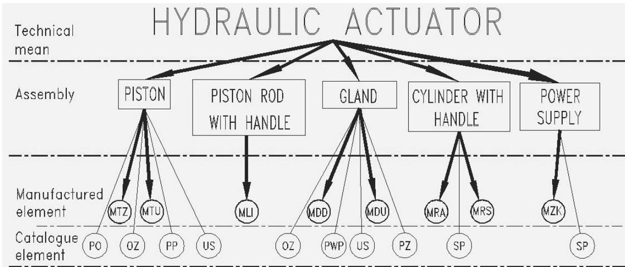
Fig. 6. Legacy of hydraulic actuator system structure based on technical drawing presented in Fig. 4a
