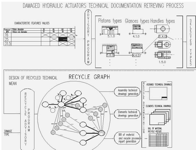
Fig. 9. Technical means recycle advisory program schema
