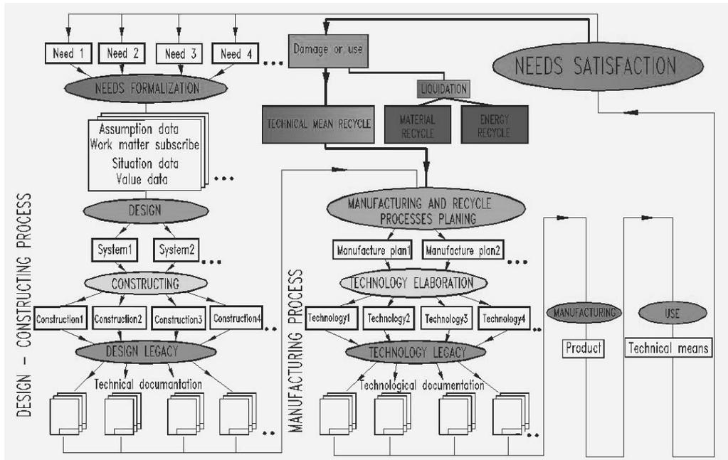
Fig. 3. Overall design process combined with manufacturing and recycle processes
