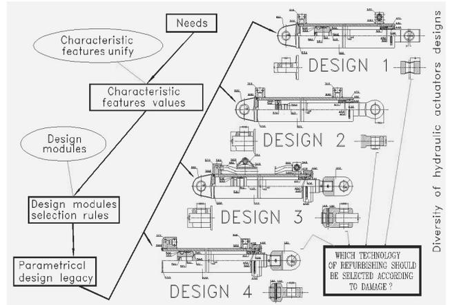
Fig. 2. Model of hydraulic actuators designs based generation with use of design modular system
