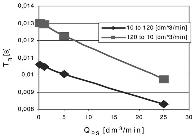
Fig. 12. Pressure setting times  $T_R$  for flow rate step
