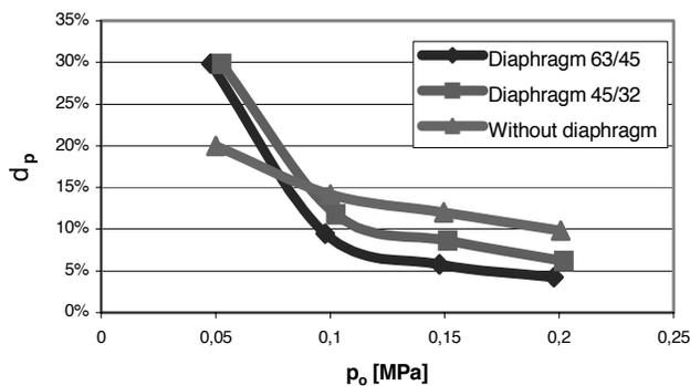
Fig. 8. Influence of the diaphragm dimensions and the pressure setting on the inequality factor of the pressure  $\delta_p$
