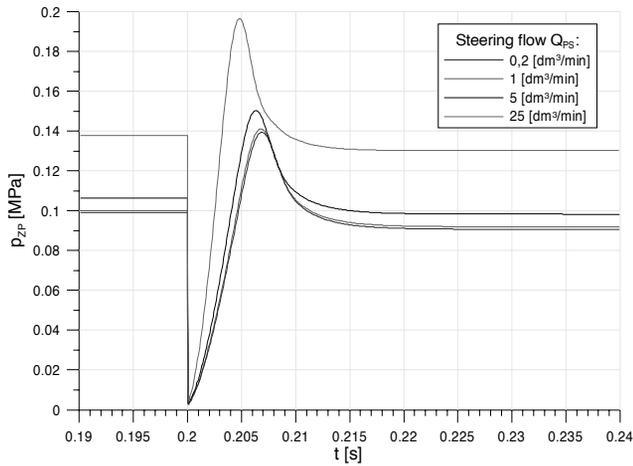
Fig. 11. Pressure response for flow rate step from 120 to 10 dm<sup>3</sup>/min
