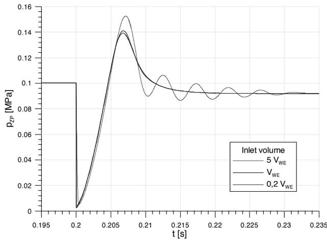
Fig. 16. The valve response on flow step 120 to 10 dm<sup>3</sup>/min for different inlet volumes
