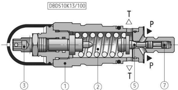
Fig. 2. Typical direct operated pressure relief valve [2]
