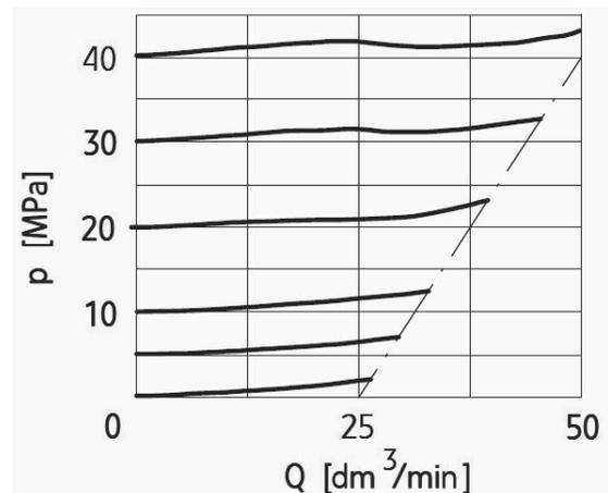
Fig. 3. Performance curves of the direct operated pressure relief valves type DBD 6 [2]
