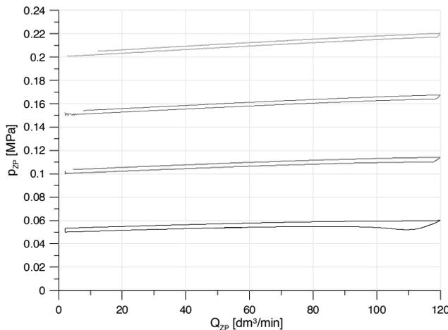
Fig. 7. Characteristic curves of the low pressure relief valve without diaphragm
