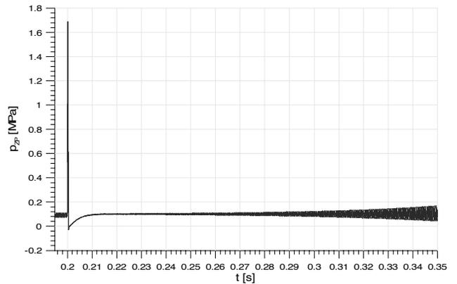
Fig. 14. The valve response on flow step 10 to 120 dm<sup>3</sup>/min for  $V_{ST} = 3.73 \cdot 10^{-6} \text{ m}^3$
