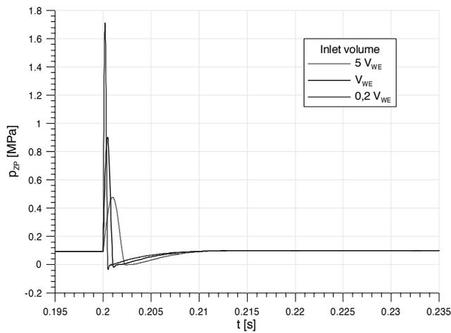
Fig. 15. The valve response on flow step 10 to 120 dm<sup>3</sup>/min for different inlet volumes
