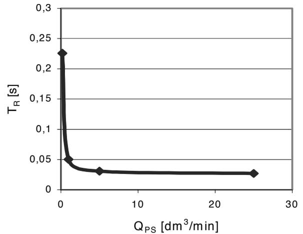
Fig. 21. Pressure setting times  $T_R$  for current step
