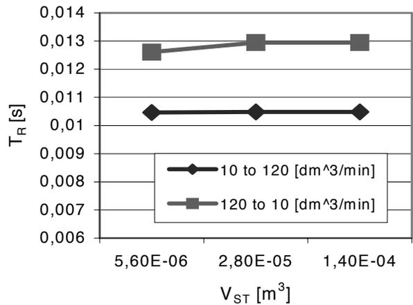
Fig. 13. The influence of auxiliary system volume on the pressure setting times
