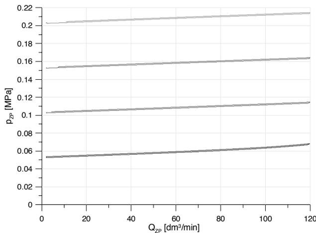
Fig. 6. Characteristic curves of the low pressure relief valve with Ø45/32 diaphragm
