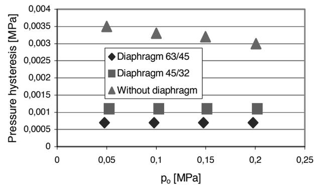
Fig. 9. Influence of the diaphragm dimensions and the pressure setting on the pressure hysteresis
