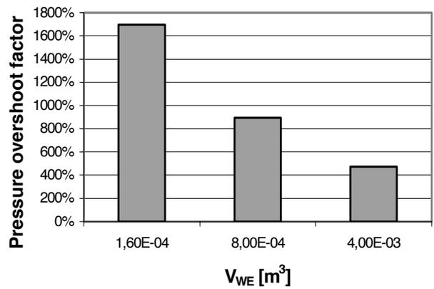
Fig. 18. The influence of inlet volume V<sub>WE</sub> on the peak pressures for flow step
