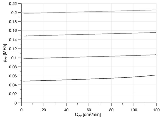
Fig. 5. Characteristic curves of the low pressure relief valve with Ø63/45 diaphragm
