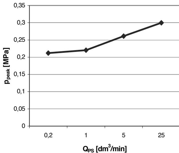
Fig. 22. The peak pressures produced by current step for different inlet volumes
