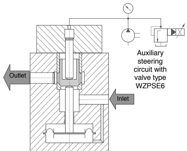
Fig. 19. Proportionally operated low pressure relief valve
