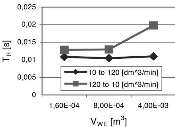
Fig. 17. The influence of inlet volume V<sub>WE</sub> on the pressure setting times T<sub>R</sub> for flow step
