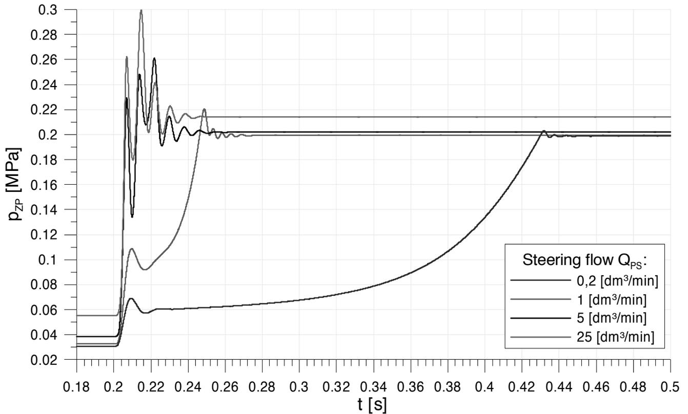
Fig. 20. Pressure response for current step from 0 to rated current at 0.2 s
