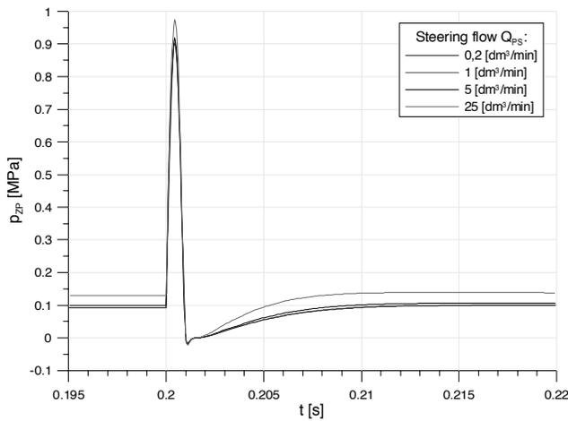
Fig. 10. Pressure response for flow rate step from 10 to 120 dm<sup>3</sup>/min
