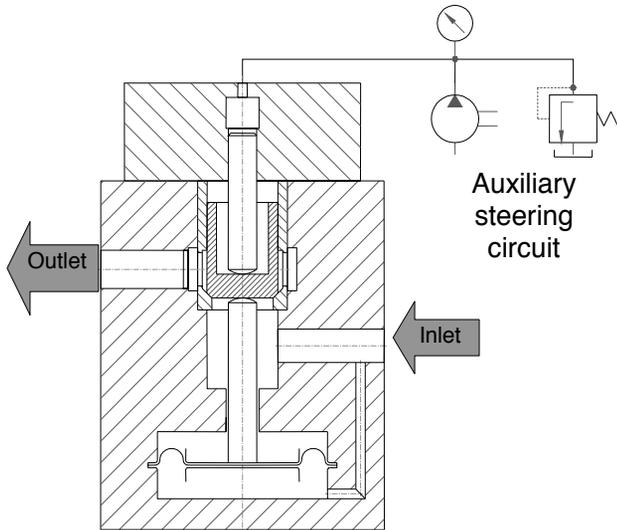
Fig. 1. Low pressure relief valve conception
