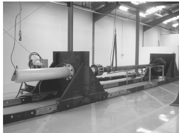
Fig. 2. Solid expandable tubular test setup: a) CAD image of the test setup, b) test setup with expandable tubular ready for test
