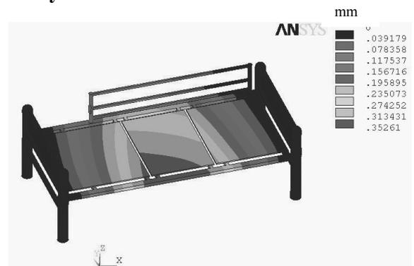
Fig. 11. Displacement distribution in bed frame, transverse stability
