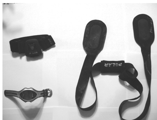
Fig. 1. Complete training system with T56H transmitter, G3 GPS sensor with battery and RS800CX receiver
