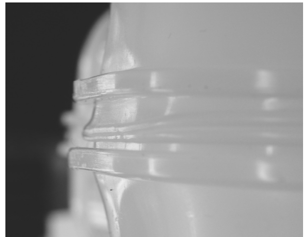
Fig. 11. View of weld's beads where the polymer was overheated
