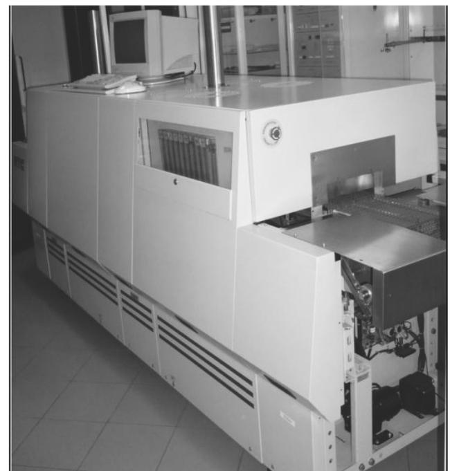
Fig. 7. LA-310 RTC type IR furnace at IMMS PAS
