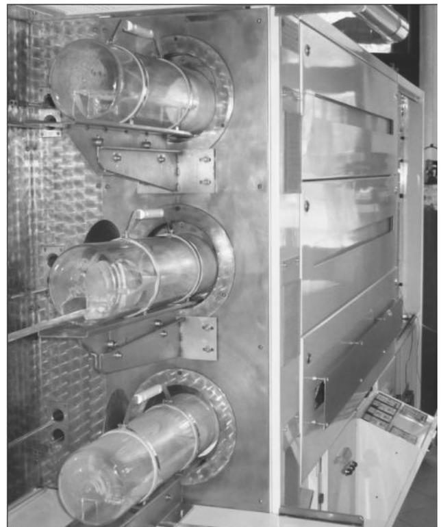
Fig. 5. PIE, SD-3/158M type diffusion furnace in IMMS PAS
