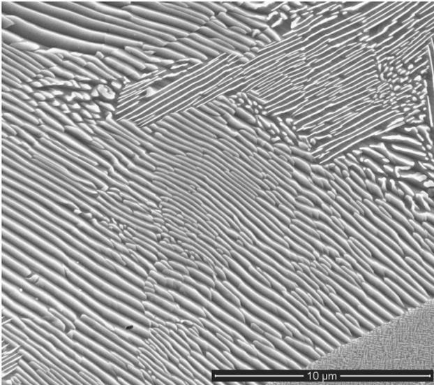
Fig. 8. Microstructure of CuTi4 alloy after supersaturation and ageing (500°C/1h). Conspicuous lamellar precipitates
