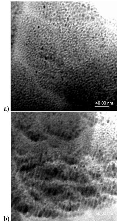
Fig. 24. Microstructure of supersaturated, cold deformed (50% reduction) and aged (550°C/1 min.) CuTi4 alloy; image in bright field; conspicuous areas of discrete precipitation a), and area of continuous precipitation b)
