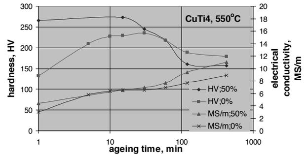
Fig. 19. Changes of hardness and electrical conductivity after supersaturation and ageing, and after supersaturation, cold deformation (50%) or ageing of CuTi4 alloy for ageing temperature of 550°C
