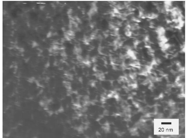
Fig. 10. Microstructure of CuTi4 alloy after supersaturation and ageing (500°C/10 min.). Conspicuous small precipitates of second phase
