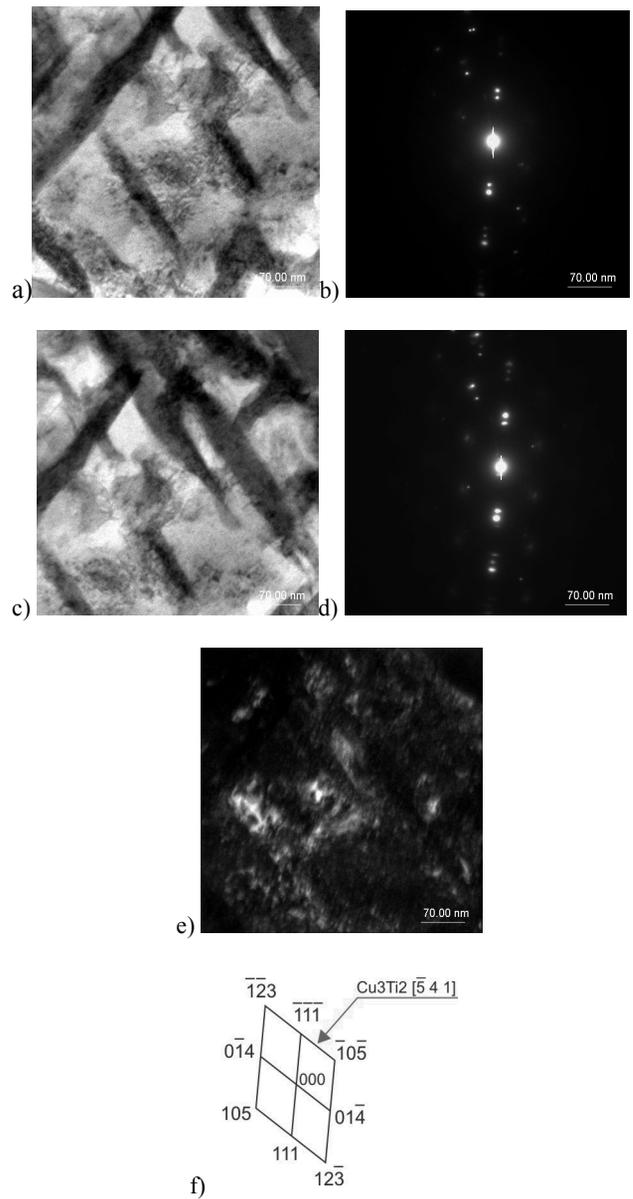
Fig. 22. Microstructure of supersaturated, cold deformed (50% reduction) and aged (550°C/1 min.) CuTi4 alloy. Cu<sub>3</sub>Ti<sub>2</sub> precipitate
