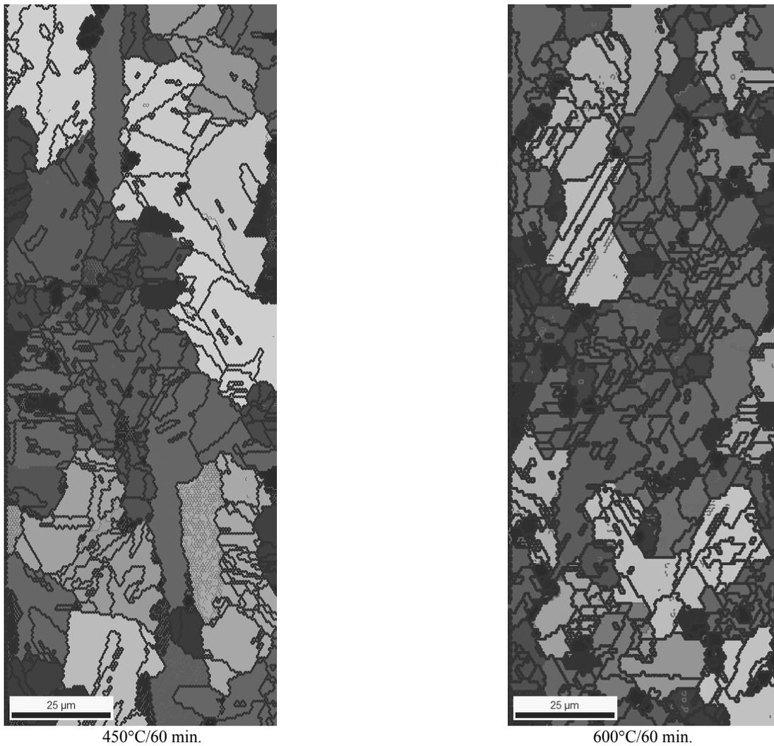
Fig. 27. Grain size distribution in CuTi4 alloy supersaturated, cold deformed with 50% reduction and aged at the temperature of 450°C for 60 minutes and at a temperature of 600°C for 60 minutes
