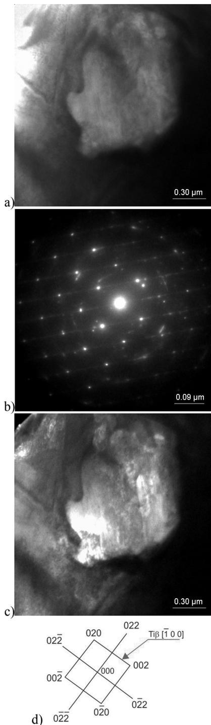
Fig. 21. Microstructure of supersaturated, cold deformed (50% reduction) and aged (550°C/1 min.) CuTi4 alloy. Original, undissolved Ti particle
