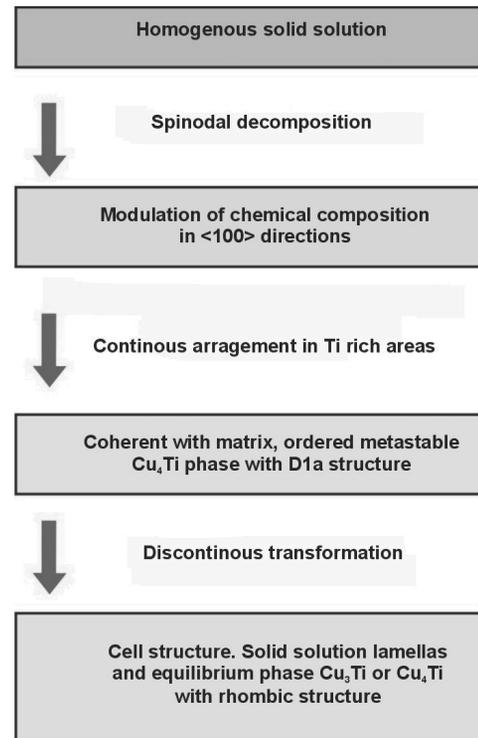
Fig. 34. Phase transitions in Cu-Ti alloys [9]
