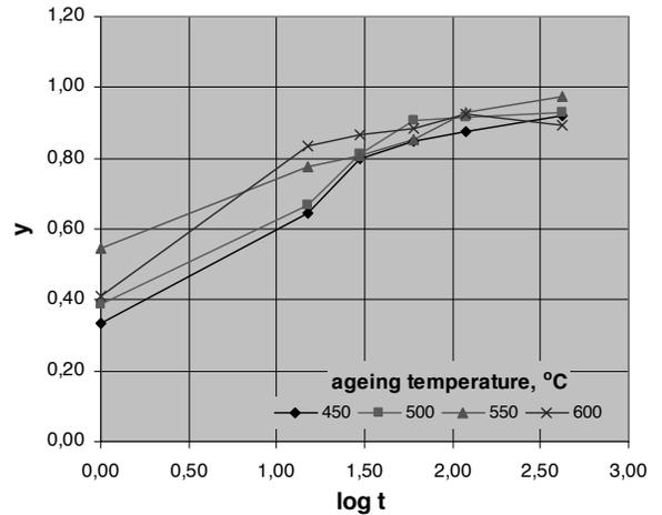
Fig. 15. Changes in extent of reaction y vs. temperature and ageing time of supersaturated and cold deformed (50% reduction) CuTi4 alloy
