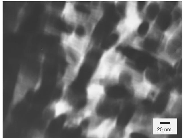
Fig. 11. Microstructure of CuTi4 alloy after supersaturation and ageing (500°C/0.5 h). Conspicuous growth of precipitates
