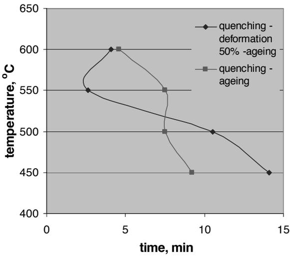
Fig. 31. TTT diagram for CuTi4 alloy after supersaturation and ageing, and after supersaturation, cold deformation (50% reduction) and for the extent of reaction  $y = 0.6321$
