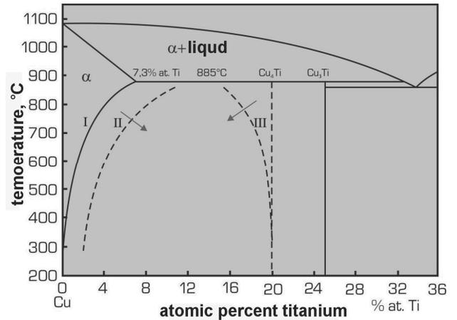
Fig. 32. Part of Cu-Ti equilibrium phase diagram; area I phase  $\alpha$  solid solution Ti in Cu; area II spinodal transformation curve; calculated with thermodynamical properties corrected by changeable solubility of  $\text{Cu}_4\text{Ti}$ ; area III presence of metastable  $\text{Cu}_4\text{Ti}$  phase and hypothetical change of its solubility (III) [5]
