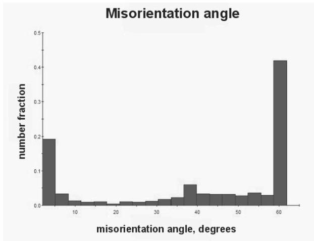
Fig. 28. Grain boundary misorientation angle distribution in CuTi4 alloy supersaturated, cold deformed with 50% reduction and aged at a temperature of 450°C for 60 minutes
