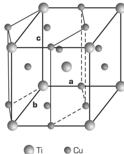
Fig. 35. Reciprocal orientation of unit cells of phase  $\beta'$  (hexagonal) and phase  $\beta$  (orthorhombic) [9]
