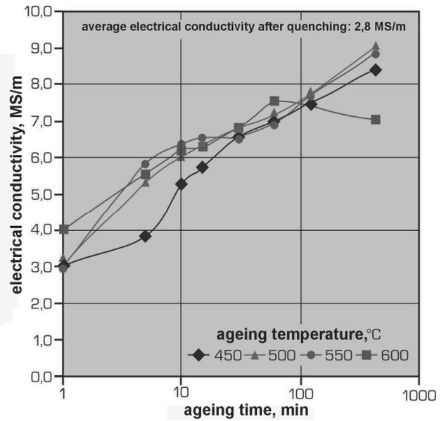
Fig. 6. Electrical conductivity  $\gamma$  of supersaturated CuTi4 alloy vs. temperature and ageing time
