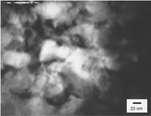
Fig. 12. Microstructure of CuTi4 alloy after supersaturation and ageing (550 C/7h) Conspicuous part of dissolved precipitates
