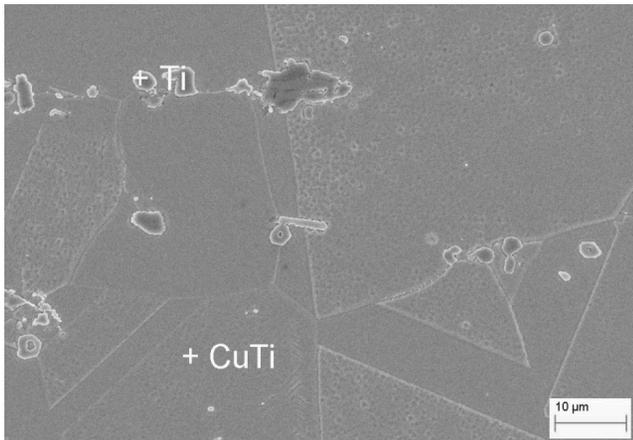
Fig. 4. Microstructure of CuTi4 alloy after supersaturation, + zones of chemical microanalysis (EDS)
