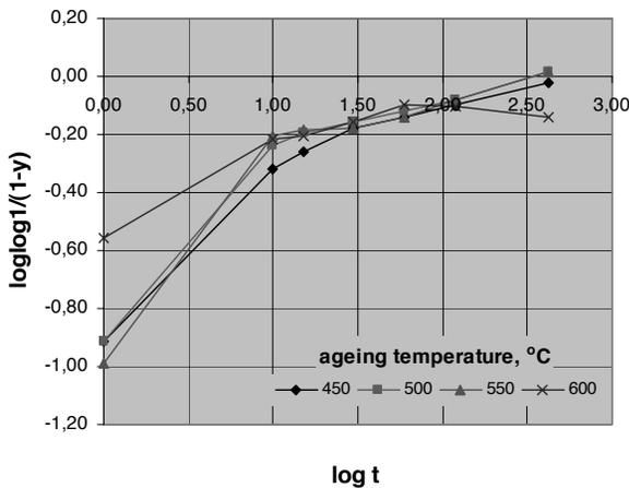
Fig. 14. Dependency between loglog 1/(1-y) and log t of supersaturated CuTi4 alloy in various ageing temperatures
