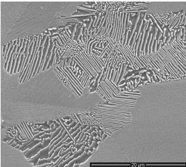
Fig. 9. Microstructure of CuTi4 alloy after supersaturation and ageing (500°C/1h) Conspicuous areas of continuous and discrete precipitation
