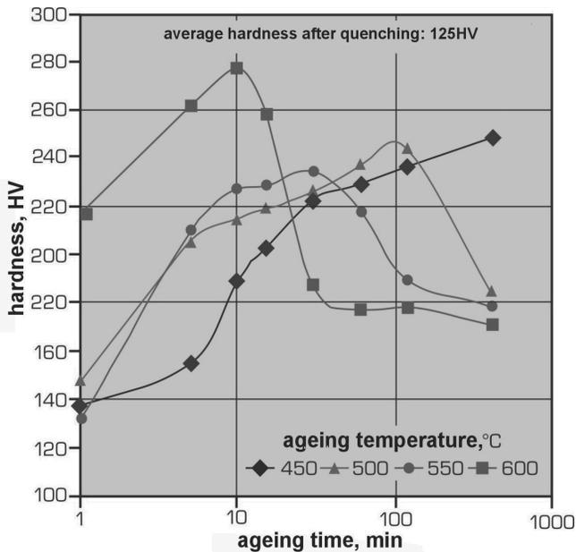
Fig. 5. Hardness of supersaturated CuTi4 alloy vs. temperature and ageing time
