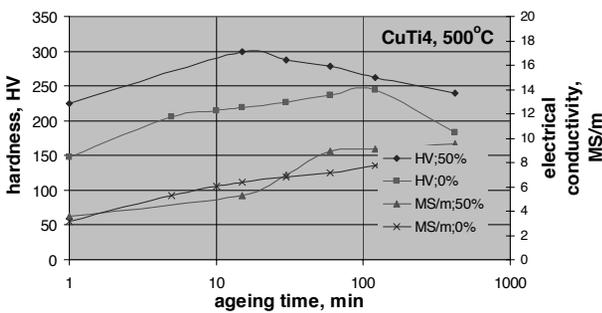
Fig. 18. Changes of hardness and electrical conductivity after supersaturation and ageing, and after supersaturation, cold deformation (50%) and ageing of CuTi4 alloy for ageing temperature of 500°C
