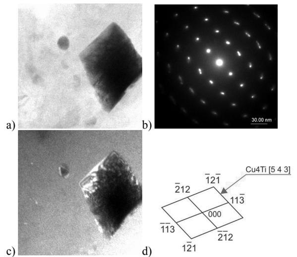
Fig. 25. Microstructure of supersaturated, cold deformed (50% reduction) and aged (550°C/1 min.) CuTi4 alloy
