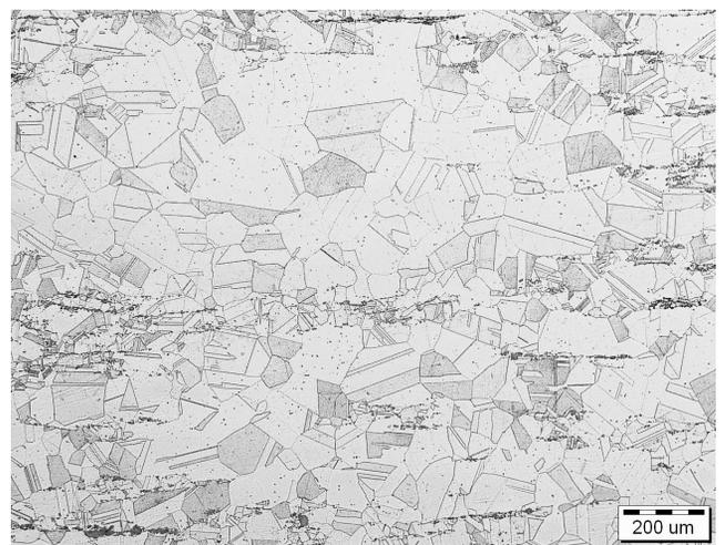
Fig. 3. Microstructure of CuTi4 alloy after supersaturation (900°C/1h/water)
