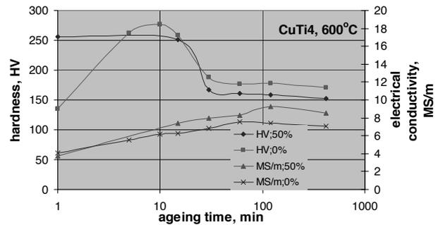
Fig. 20. Changes of hardness and electrical conductivity after supersaturation and ageing, and after supersaturation, cold deformation (50%) or ageing of CuTi4 alloy for ageing temperature of 600°C
