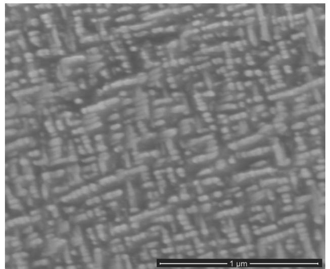
Fig. 7. Microstructure of CuTi4 alloy after supersaturation and ageing (500°C/1h)
