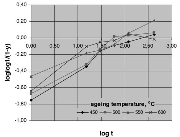
Fig. 16. Dependency between loglog 1/(1-y) and log t of supersaturated and cold deformed (50% reduction) CuTi4 alloy in various ageing temperatures
