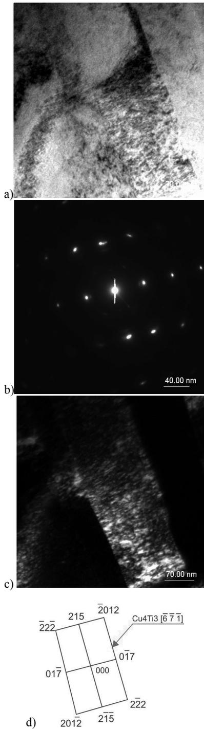
Fig. 23. Microstructure of supersaturated, cold deformed (50% reduction) and aged (550°C/1 min.) CuTi4 alloy
