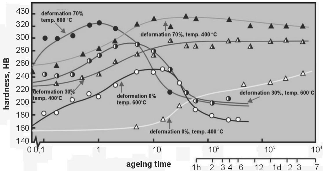
Fig. 33. Hardness of CuTi4.29 alloy after supersaturation versus ageing temperature, cold deformation and ageing time [5]
