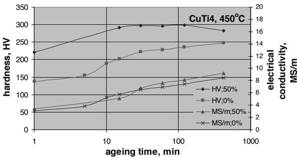
Fig. 17. Changes of hardness and electrical conductivity after supersaturation and ageing, and after supersaturation, cold deformation (50%) of ageing of CuTi4 alloy for ageing temperature of 450°C
