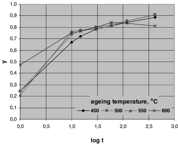
Fig. 13. Changes in extent of reaction y vs. temperature and ageing time of supersaturated CuTi4 alloy
