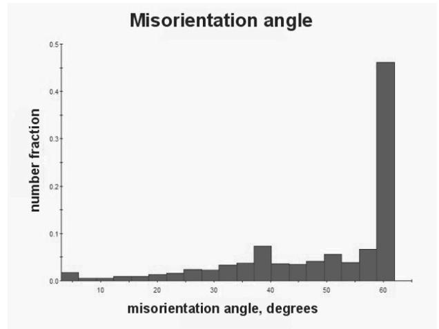
Fig. 29. Grain boundary misorientation angle distribution in CuTi4 alloy supersaturated, cold deformed with 50% reduction and aged at a temperature of 600°C for 60 minutes
