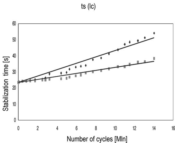
Fig. 8. Dependence of temperature time stabilization versus the number of fatigue cycles for measuring points 2, 3 and 1, 4
