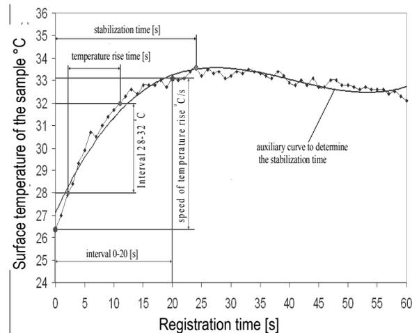
Fig. 4. The course of temperature changes during thermographic measurement
