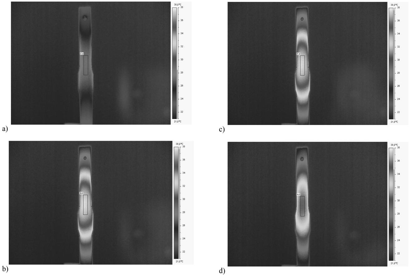
Fig. 6. The series of images of successive phases of the thermal process, taking place on the sample surface: measurement start (a), maximum temperature (b), the initial phase of descent (c), the end of measurement (d)
