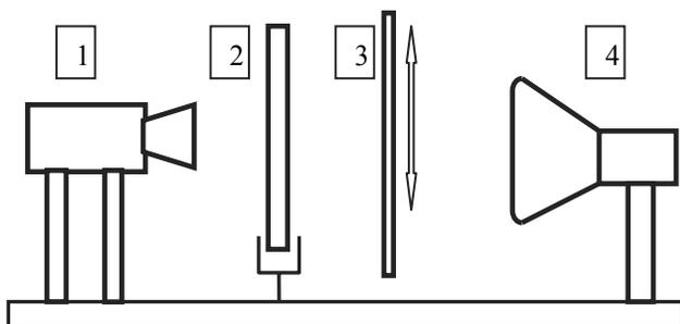
Fig. 3. Schematic draw of thermovision research stand. 1 - thermovision camera, 2 - sample, 3 - removable shield, 4 - infrared radiator
