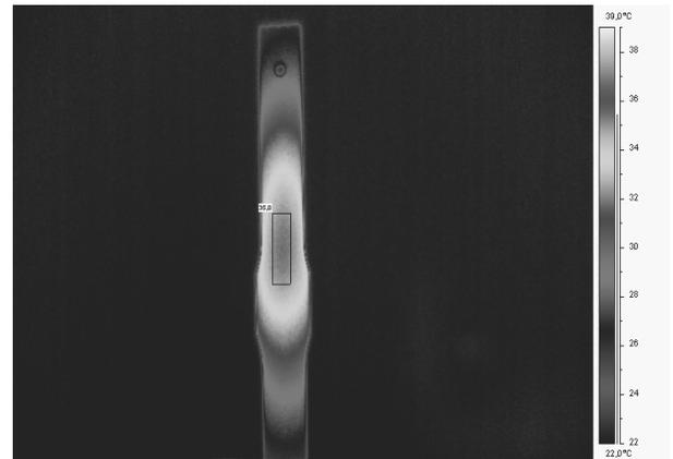
Fig. 5. Example thermogram for the samples subjected to fatigue tests at 10 million cycles (the temperature was read from inside the selected rectangular area)
