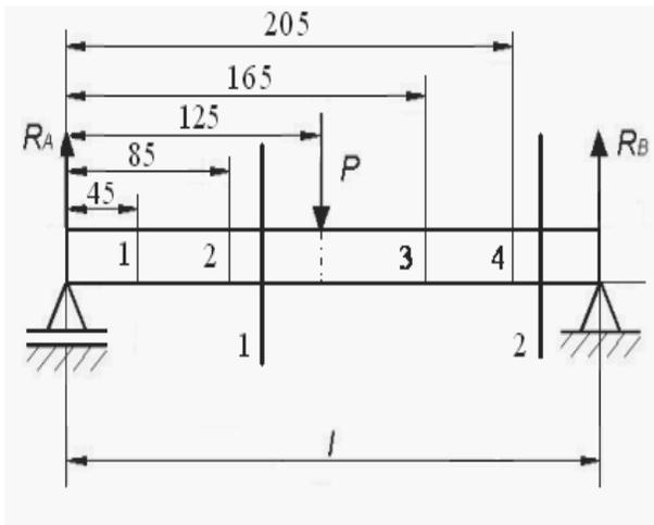
Fig. 2. Diagram of the distribution of forces and reactions acting during deformation of the sample in the fatigue machine and the distribution of measurement points: 1, 2, 3 and 4
