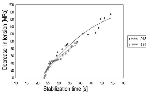
Fig. 9. The dependence of stress drop on the temperature stabilization time for measuring points 2, 3 and 1, 4
