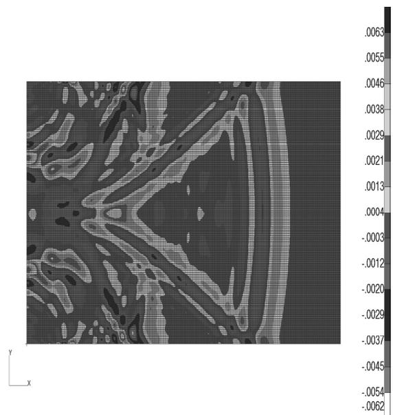
Fig. 5. Displacements map along x-axis of the composite after a period of  $4.5 \cdot 10^{-3}$  ms
