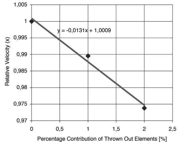
Fig. 9. Dependence of wave velocity on the degree of model fatigue degradation of the material
