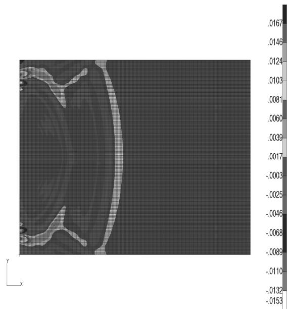
Fig. 4. Displacements map along x-axis of the composite after a period of  $2.5 \cdot 10^{-3}$  ms
