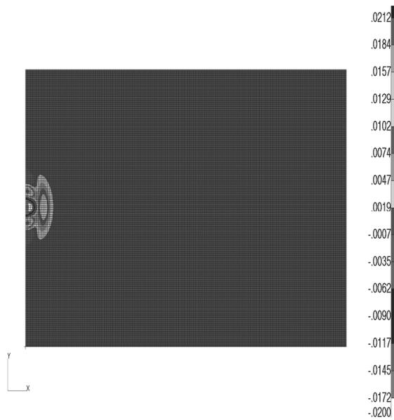
Fig. 2. Displacements map along x-axis of the composite after a period of  $5.0 \cdot 10^{-4}$  ms
