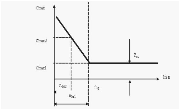
Fig.1. Simplified Wöhler diagram for tension and compression;  $Z_{rc}$  - fatigue limit of tensile and compressive strength,  $n_g$  - limit the number of cycles
