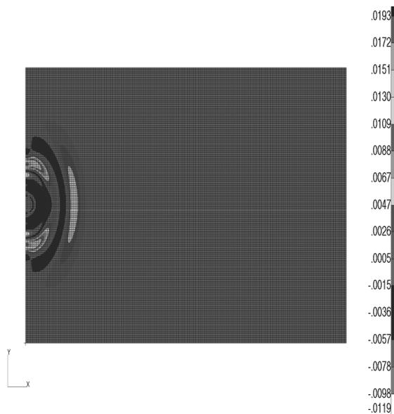
Fig. 3. Displacements map along x-axis of the composite after a period of  $1.0 \cdot 10^{-3}$  ms
