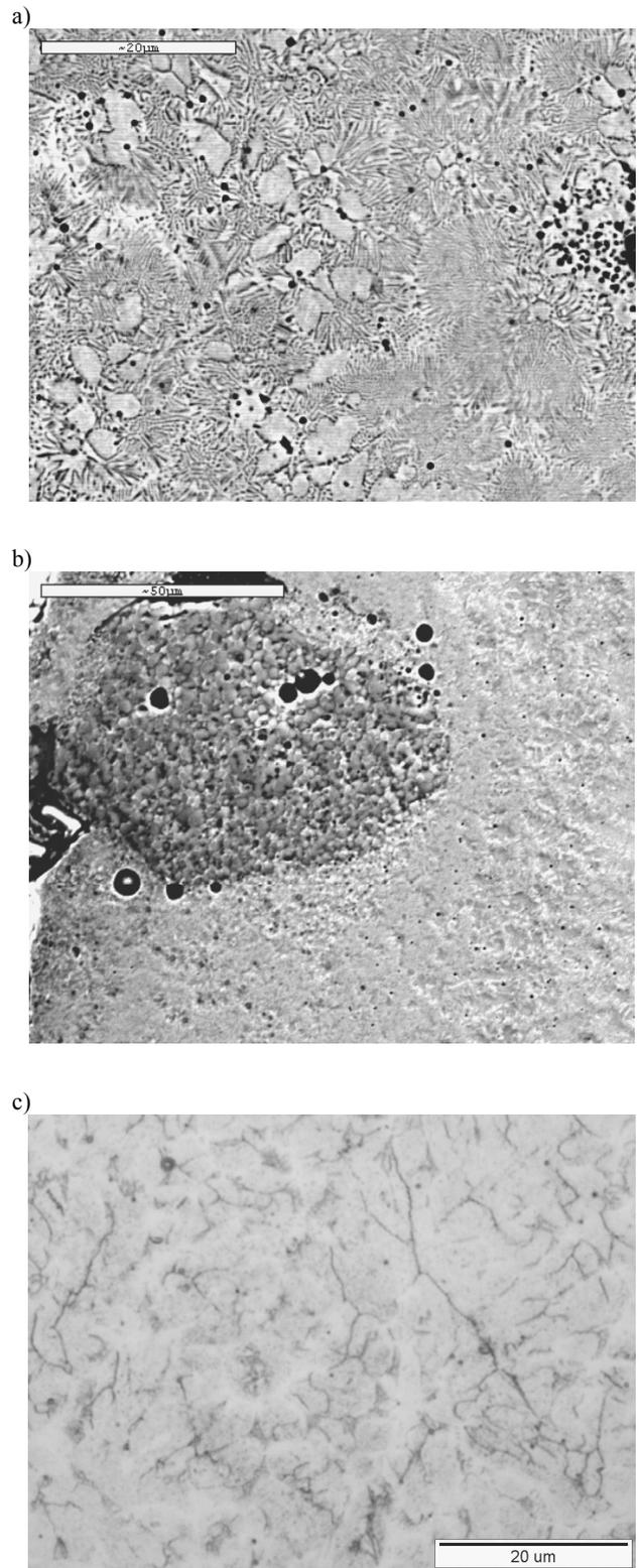
Fig. 5. Surface layer of the steel X40CrMoV5-1 after alloying with VC powder, laser power a) 1.6 kW, b) 1.2 kW, c) 2.3 kW
