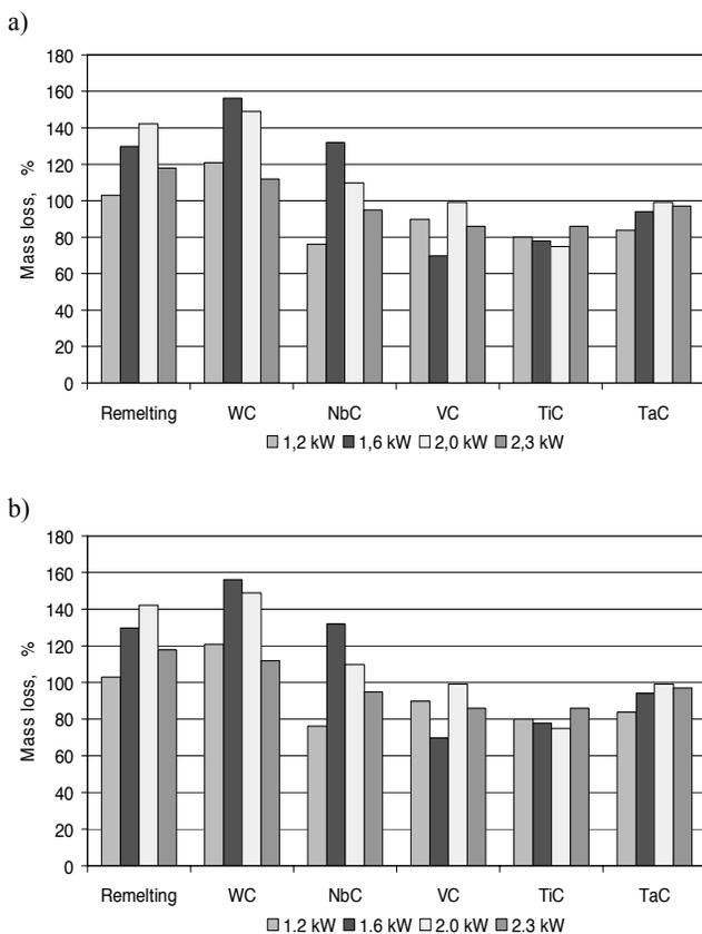
Fig. 6. Mass loss in comparison to the applied ceramic powder in the surface layer of the a) X40CrMoV5-1, b) 32CrMoV12-28
