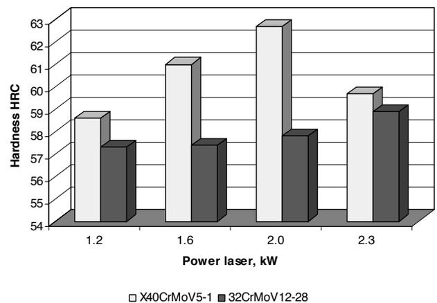
Fig. 7. Average hardness changes of the surface layer of the: a) X40CrMoV5-1, b) 32CrMoV12-28 steels alloyed with VC carbides with 1.2-2.3 kW laser power
