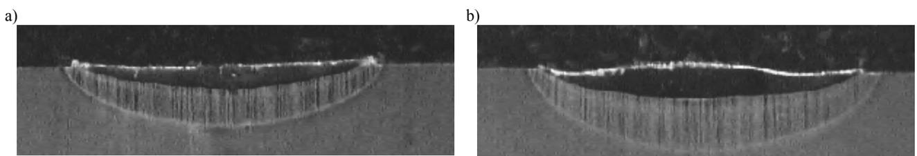
Fig. 3. Remelted and heat affected zone in the surface layer of the 32CrMoV12-28 hot work tool steel alloyed with VC, scanning rate 0.5 m/min., a) power range 1.2 kW, b) power range 2.0 kW, mag. 50x
