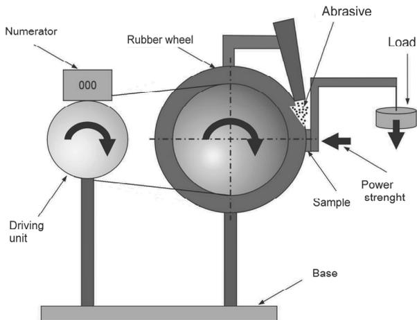
Fig. 4. Experimental stand for the abrasive wear investigations in a metal - ceramic system according to the ASTM G65
