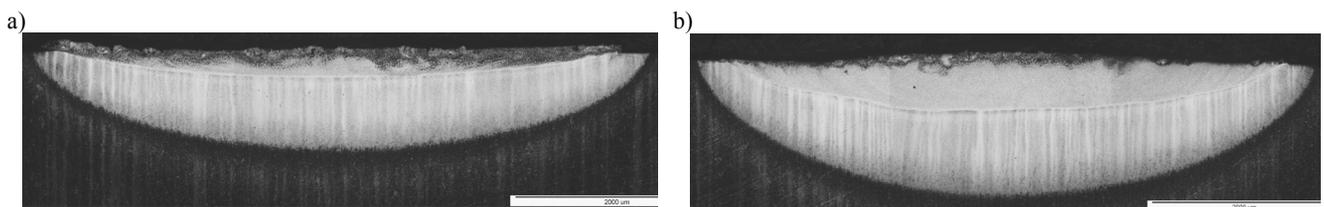
Fig. 2. Remelted and heat affected zone in the surface layer of the X40CrMoV5-1 hot work tool steel alloyed with VC, scanning rate 0.5 m/min., a) power range 1.2 kW, b) power range 2.0 kW, mag. 50x
