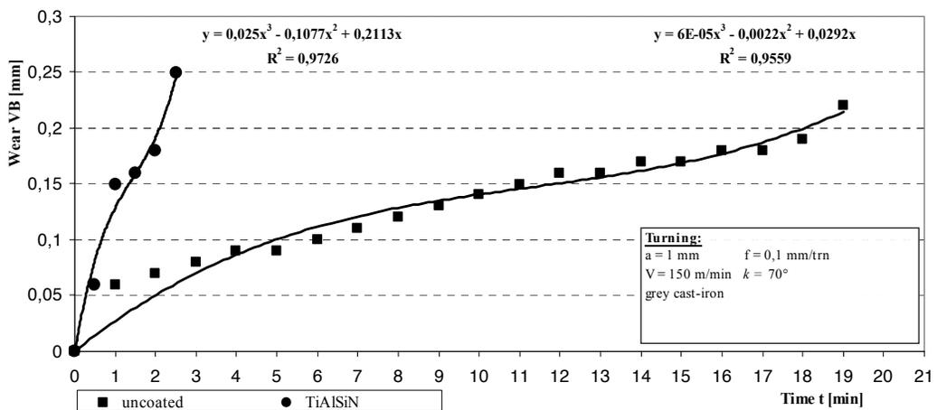
Fig. 10. Comparison of the approximated values of the VB wear of the cermet sample: uncoated and coated with the (Ti,Al,Si)N coating, depending on machining time
