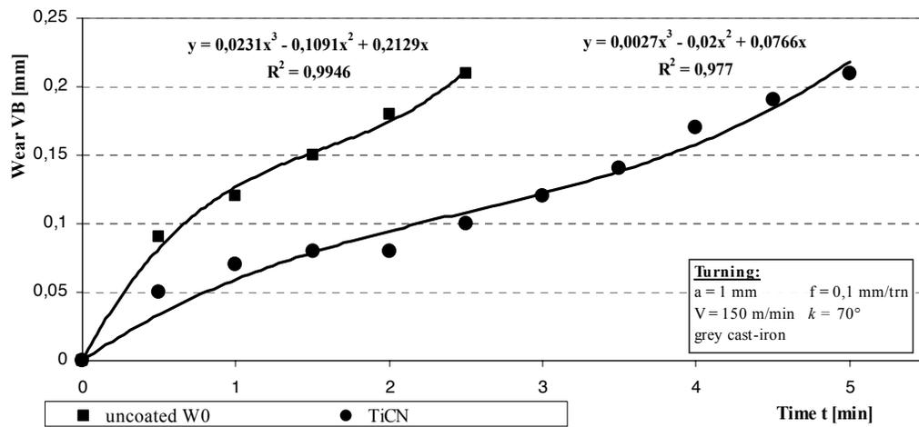
Fig. 6. Comparison of the approximated values of the VB wear of the cemented carbides sample: uncoated and coated with the Ti(C,N) coating, depending on machining time
