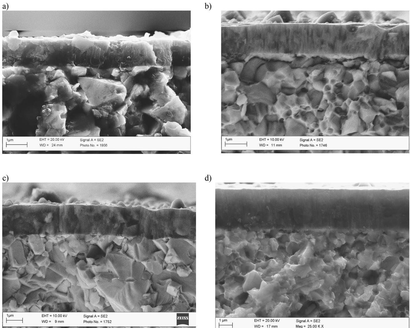
Fig. 1. Structure of the: a) Ti(C, N) coating deposited onto the cemented carbide substrate b) Ti(C, N) coating deposited onto the cermet substrate, c) (Ti,Al)N coating deposited onto the cemented carbides substrate, d) (Ti,Al,Si)N coating deposited onto the cermet substrate
