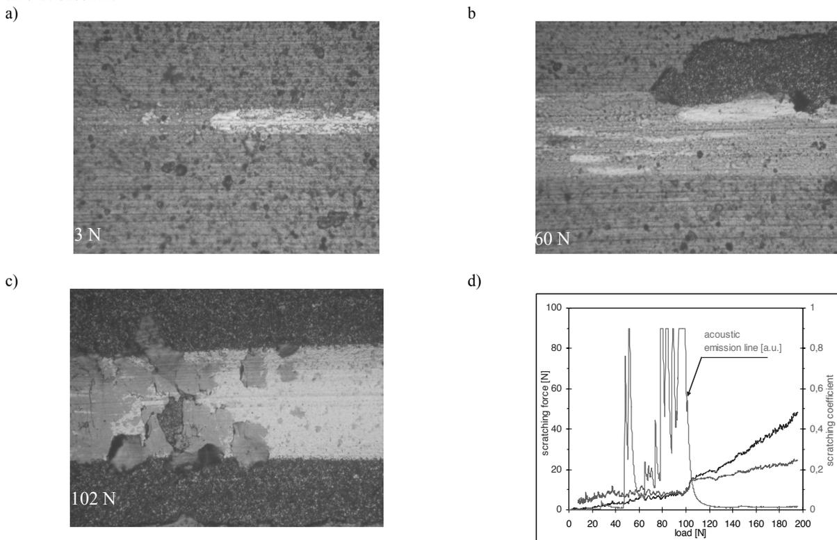
Fig. 4. a), b), c): Indenter trace with the optical  $L_c$  load, d) scratch test results of the (Ti,Al,Si)N coating surface deposited on cermet substrate
