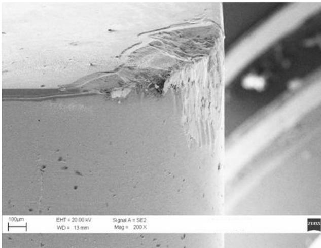
Fig. 11. Character of wear of cermet sample with (Ti,Al)N coating, investigated with SEM after cutting test
