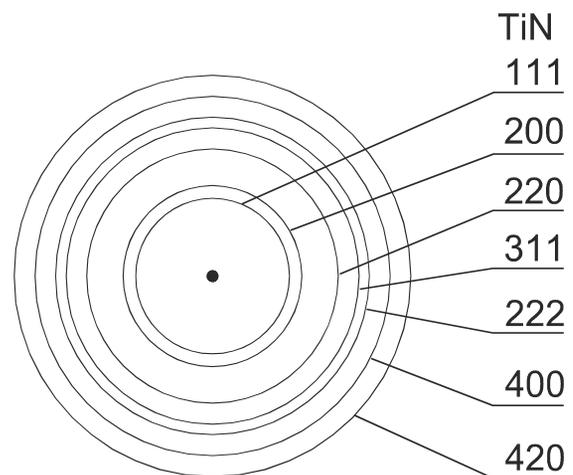
Fig.2. a) Structure of the thin foil from the (Ti,Al,Si)N coating deposited on cermet substrate, b) diffraction pattern for the area as from figure a, c) solution of the diffraction pattern from figure b.
