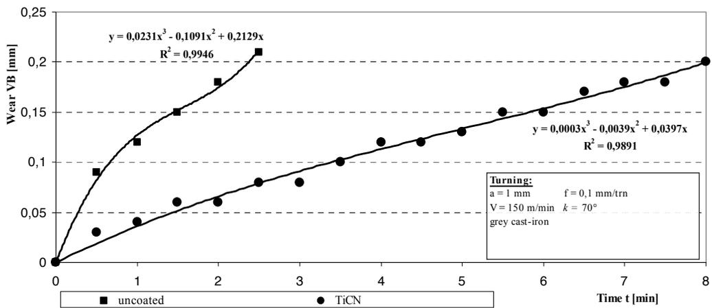
Fig. 9. Comparison of the approximated values of the VB wear of the cermet sample: uncoated and coated with the Ti(C,N) coating, depending on machining time
