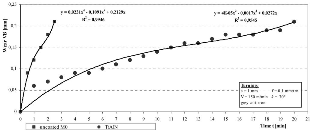
Fig. 8. Comparison of the approximated values of the VB wear of the cermet sample: uncoated and coated with the (Ti,Al)N coating, depending on machining time
