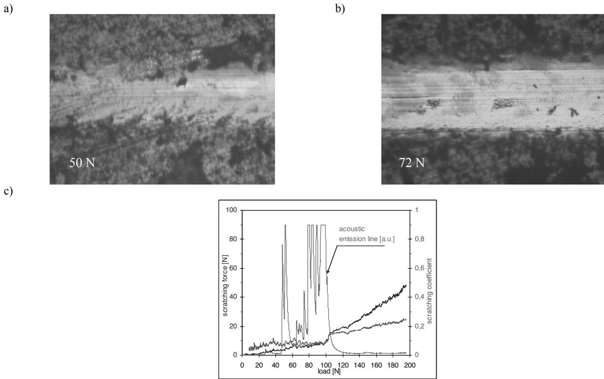
Fig. 3. a), b): Indenter trace with the optical  $L_c$  load, c) scratch test results of the (Ti,Al,Si)N coating surface deposited on cemented carbide substrate
