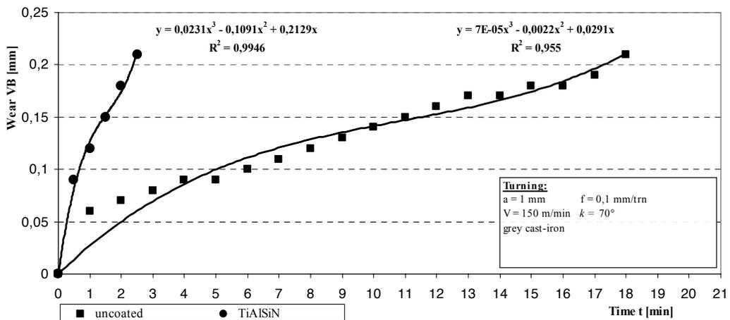
Fig. 7. Comparison of the approximated values of the VB wear of the cemented carbide sample: uncoated and coated with the (Ti,Al,Si)N coating, depending on machining time
