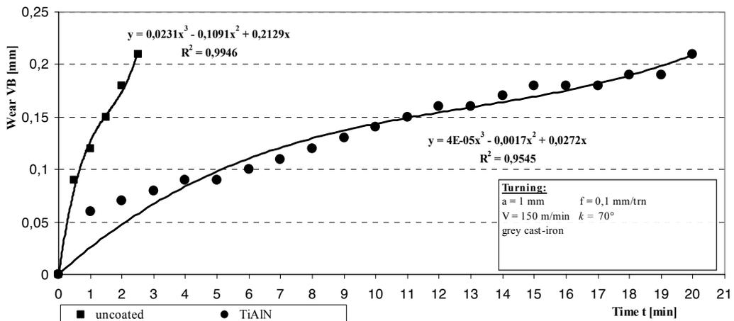
Fig. 5. Comparison of the approximated values of the VB wear of the cemented carbide sample: uncoated and coated with the (Ti,Al)N coating, depending on machining time
