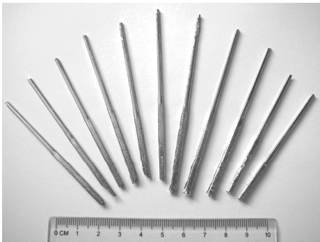
Fig. 1. Outer morphology of cast glassy \text{Fe}_{72}\text{B}_{20}\text{Si}_4\text{Nb}_4 alloy rods with diameters of 1.5 and 2 mm [8]
