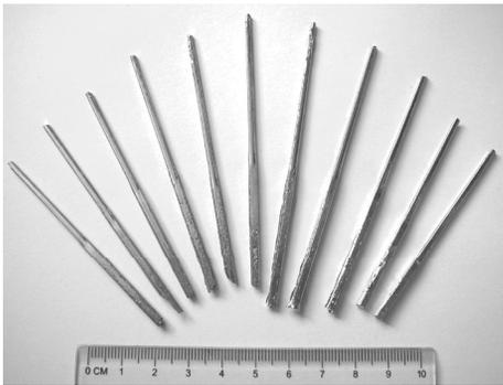
Fig. 1. Outer morphology of cast glassy  $\text{Fe}_{72}\text{B}_{20}\text{Si}_4\text{Nb}_4$  alloy rods with diameters of 1.5 and 2 mm [8]
