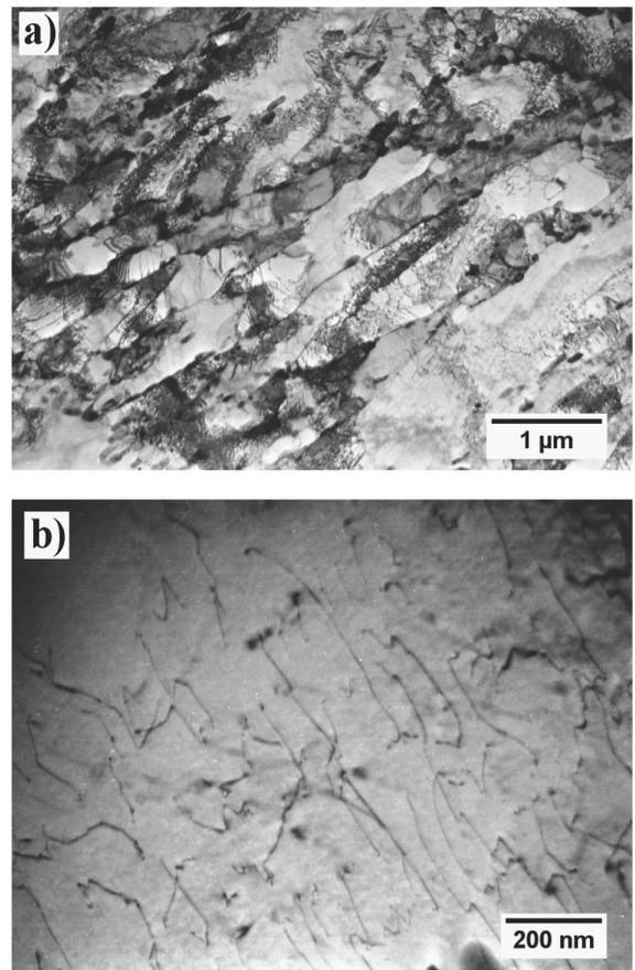
Fig. 3. TEM micrographs of the VM12 steel austenitised at 1100 °C: a) sub-grains and  $M_{23}C_6$  precipitates, b) MX precipitates
