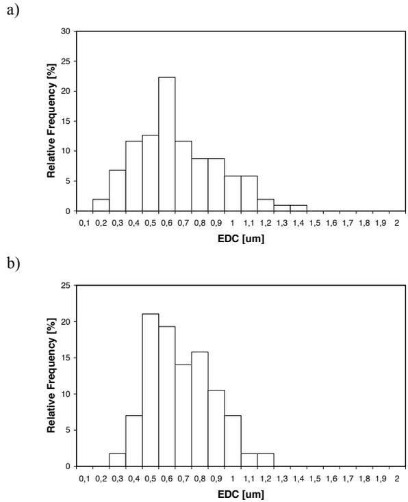
Fig. 5. Sub-grain size distribution in the specimen: a) austenitised at 1060 °C, b) austenitised at 1100 °C
