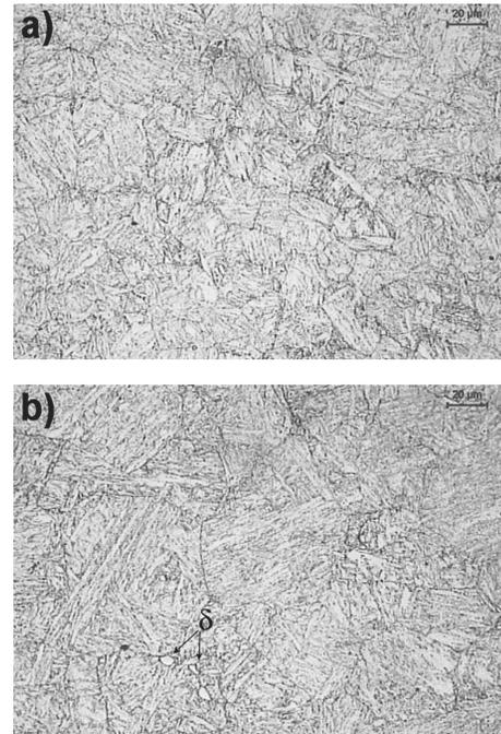
Fig. 1. Microstructure of the VM12 steel after austenitisation at a) 1060 °C, b) 1100 °C as seen by LM
