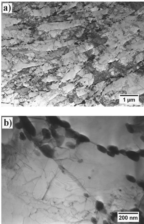
Fig. 2. TEM micrographs of the VM12 steel austenitised at 1060 °C: a) sub-grains and  $M_{23}C_6$  precipitates, b) MX precipitates
