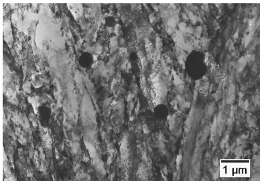
Fig. 7. Large primary particles of  $M_{23}(C, B)_6$  borocarbides
