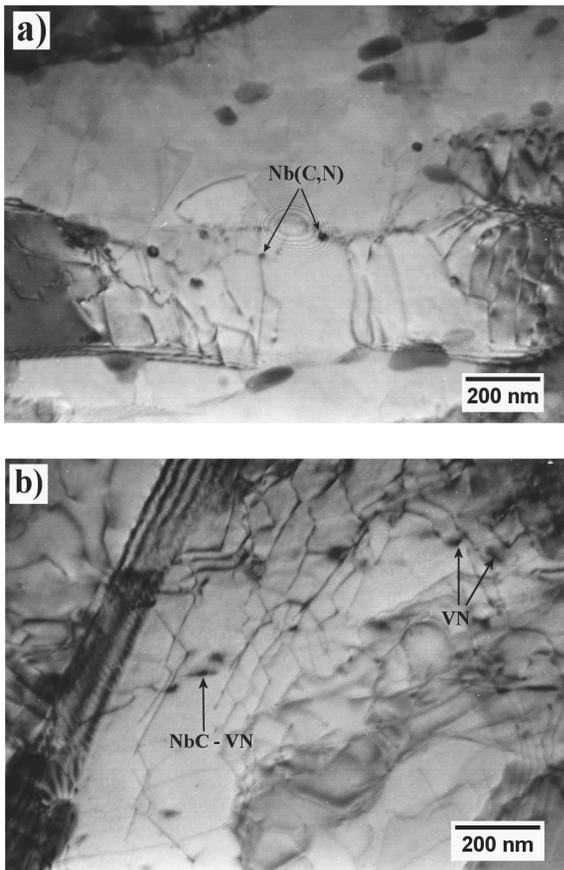
Fig. 4. MX precipitates observed in the VM12 steel
