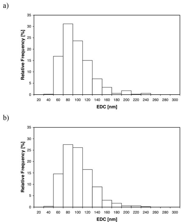
Fig. 6. Particle size distribution of  $M_{23}C_6$  precipitates in the VM12: a) austenitised at 1060 °C, b) austenitised at 1100 °C
