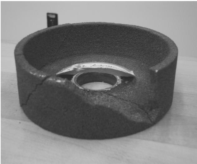
Fig. 21. Exploded View of Cup Shaped Vitrified Grinding Wheel After Recovery From the Burst Chamber
