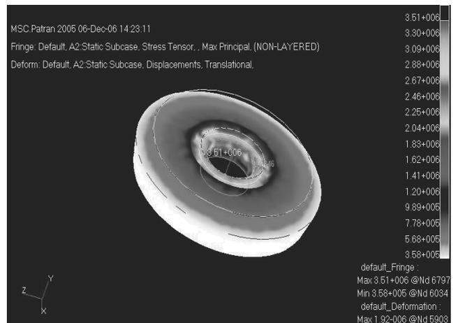
Fig. 14. Fringe Plot of Small Cup Shaped Grinding Wheel spinning at 45 m/s ( $P=100$   $F=10$ )
