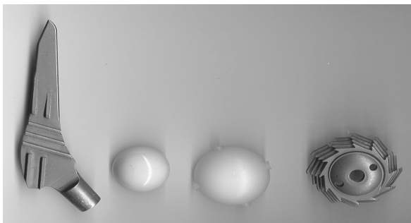
Fig. 2. The 1 st version of total hip replacement - canine model - potential - ZMR, after some modification was created model as in Fig. 3
