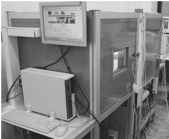
Fig. 5. The verification of modeling on two climatic chambers combined through a solar wall model in the laboratory [11]
