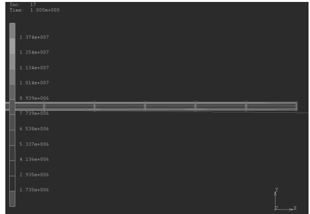
Fig. 12. Von Misses stress (N/m 2 ) in a sheet after CAF loading
