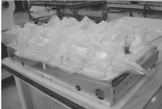
Fig. 14. Vacuum bag technique applied in CAF test [2]
