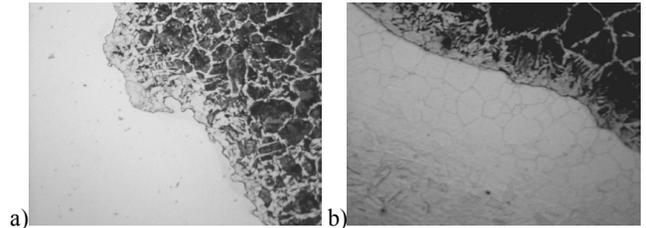
Fig. 4. The microstructure in the joint region of a bimetallic bar after explosive welding: a) - the core, zoom 100x, etched with Nital; b) - clad layer, zoom 100x, etched with 45ml H<sub>2</sub>O, 30ml HNO<sub>3</sub>, 15ml HCl, 10ml HF
