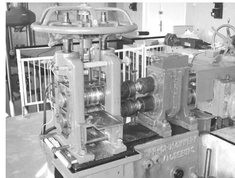
Fig. 12. Laboratory rolls Ø150 mm - general view
