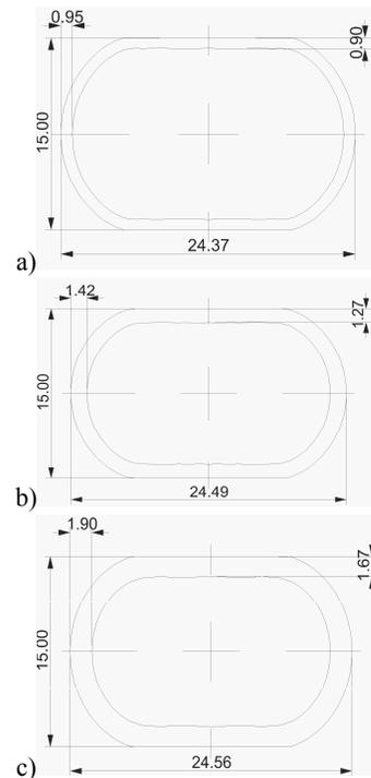
Fig. 9. The shape and dimensions of bimetallic preformed strip obtained from the theoretical examination of the process of rolling in the flat oval pass with the clad layer thickness fraction of the bimetallic stock equal to, respectively: a) 17.4%, b) 25.7%, c) 33.2%
