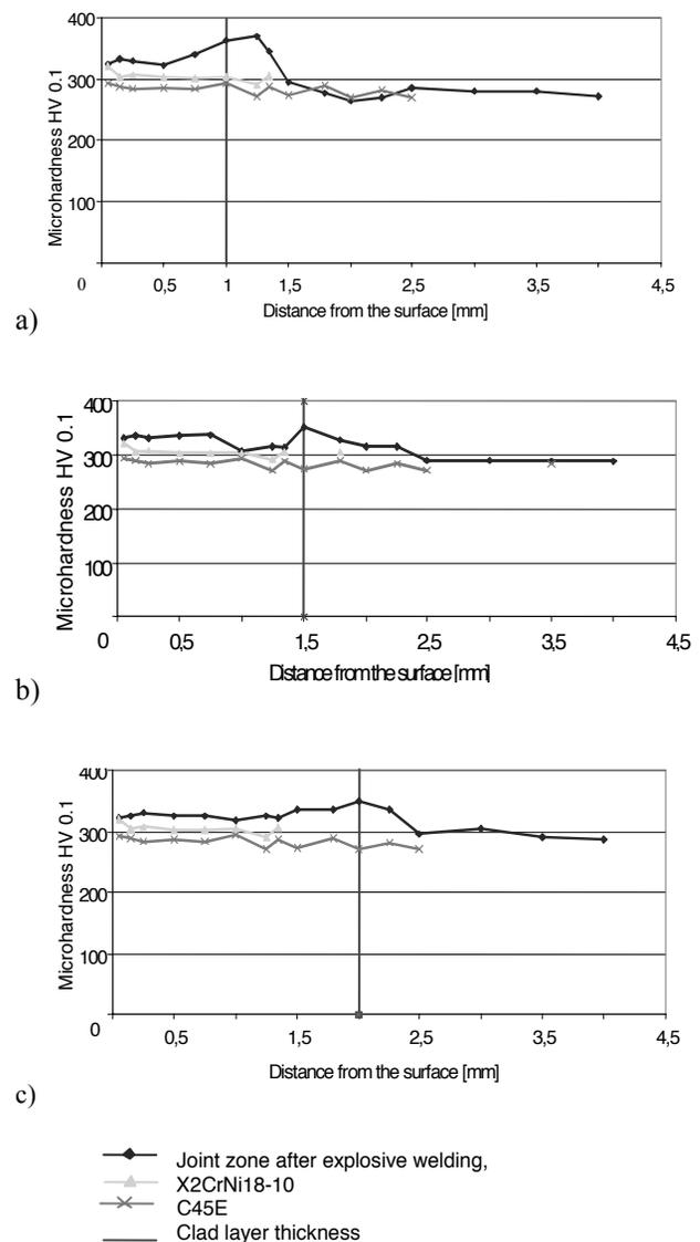
Fig.7. The distribution of microhardness for stock materials and in bimetallic bars after explosive welding; with a clad layer thickness of: a) - 1,0 mm; b) - 1,5 mm; c) - 2,0 mm
