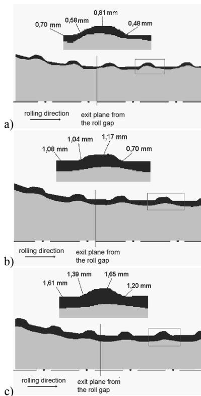
Fig. 10. Distribution of layer surface thickness on the longitudinal cross in deformation zone during bimetallic bar rolling using flat oval pass with the platter layer containing: a) 17.3 %; b) 25.5 %; c) 33.1 %
