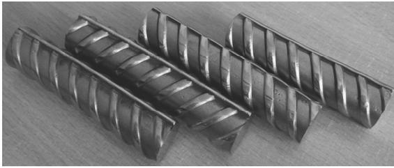
Fig. 14. Bimetallic ribbed round bars
