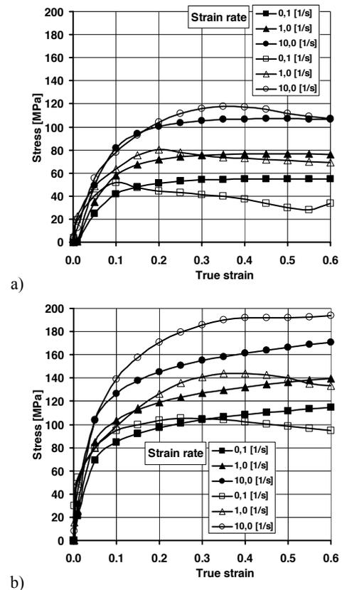
Fig. 1. Example flow curves for: a) steel C45E and b) for steel X2CrNi18-10, for a temperature of  $1100^\circ\text{C}$ , (the curves denoted with filled signs represent experimental results, the remaining curves are approximated based on experimental tests)
