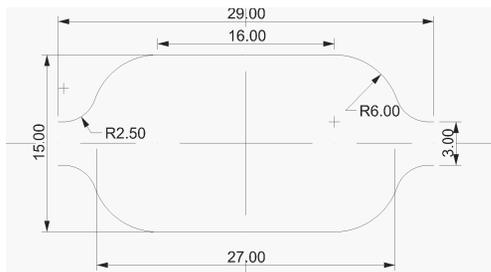
Fig. 8. The shape and dimensions of the preforming pass used in rolling
