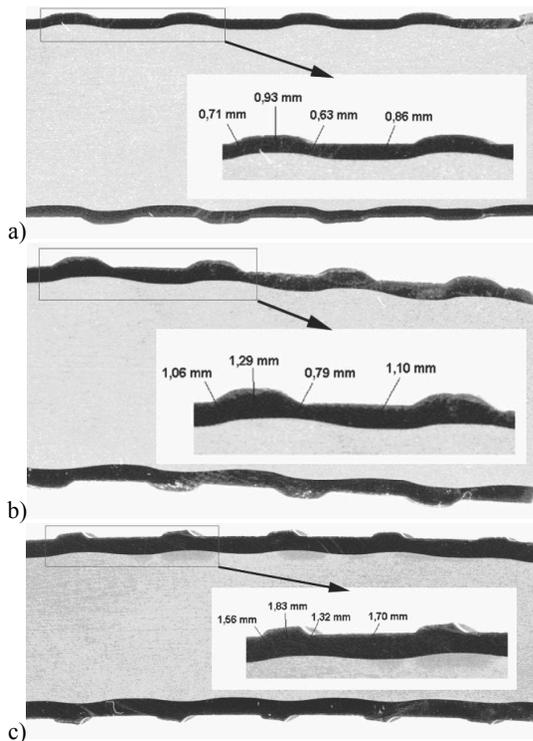
Fig. 15. Distribution of layer surface thickness on the longitudinal cross in deformation zone during bimetallic bar rolling using flat oval pass with the platter layer containing: a) 17.3 %; b) 25.5 %; c) 33.1 %
