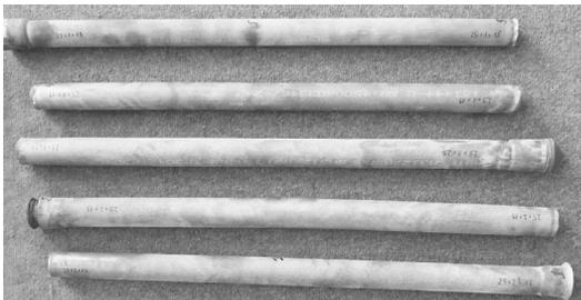
Fig. 3. Bimetallic bars after explosive welding
