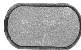
Fig. 13. View of a sample preformed oval strip designed for rolling 18 mm-diameter ribbed bars
