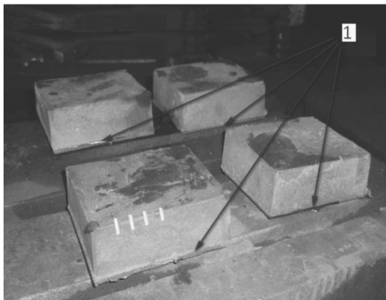
Fig. 5. View of cast iron test-castings with the surface enriched by alloy steel plate – 1
