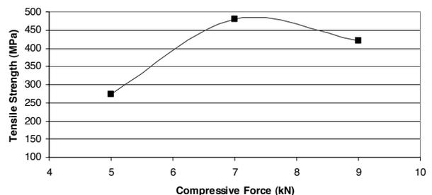
Fig. 4. Influence of the compressive tool force on the tensile strength with FSW joints having  $n=1180$  rpm,  $v_t=60$  mm/min,  $\alpha=1.5^\circ$
