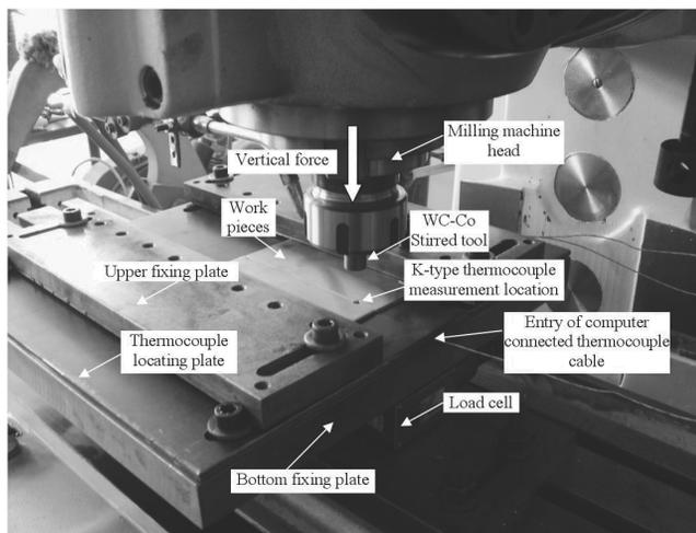
Fig. 1. Experimental setup using for friction stir welding
