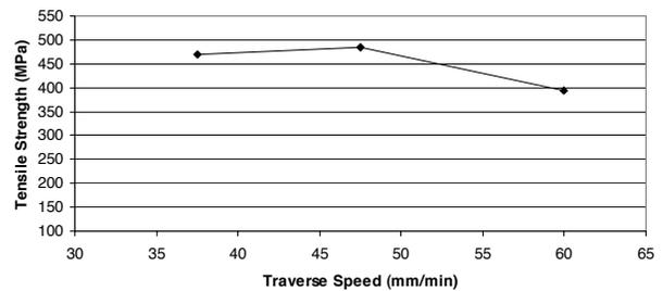
Fig. 3. Influence of the traverse speed on the tensile strength with FSW joints having  $n=750$  rpm,  $F=9$  kN,  $\alpha=1.5^\circ$
