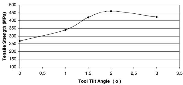
Fig. 5. Influence of the tool tilt angle on the tensile strength with FSW joints having  $n=1180$  rpm,  $vt=60$  mm/min,  $F=9$  kN
