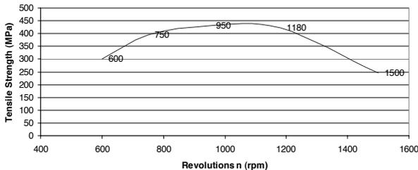
Fig. 2. The effect of the rotational tool speed on tensile strength of AISI 304 stainless steel processed by FSW with process parameters:  $v_t=60$  mm/min,  $F=9$  kN,  $\alpha=1.5^\circ$
