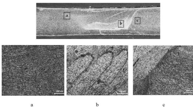
Fig. 6. Macrograph of the heat affected zone (HAZ) (a), weld zone (b) and base material (c), optical micrographs showing the microstructures of the stir welded zone processed with  $F=9$  kN,  $vt=60$  mm/min,  $n=950$  rpm,  $\alpha=1.5^\circ$
