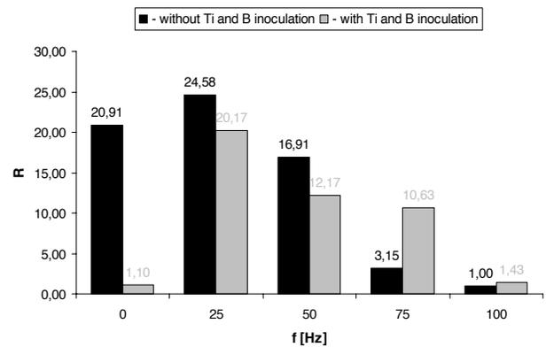
Fig.6. Value of refinement factor (R) for different versions of inoculation
