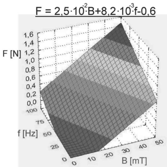
Fig. 3. Influence of frequency of supply current (f) and magnetic induction (B) on value of force (F), which generating the movement of liquid metal in mould with diameter 25mm
