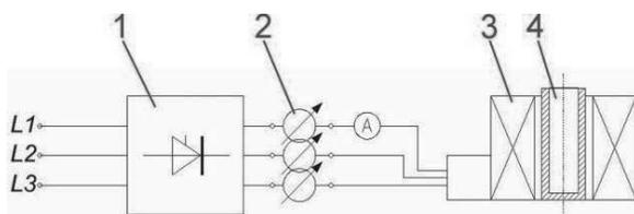
Fig. 2. Scheme of test stand: 1 - inverter, 2 - autotransformer, 3 - induction coil, 4 - mould containing liquid metal, A - ammeter
