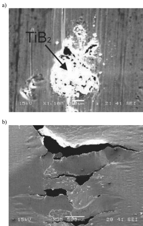
Fig. 1. Phase  $TiB_2$  in structure of pure Al (a) and produced in result from its present crack in sheet (foil) during rolling [12]
