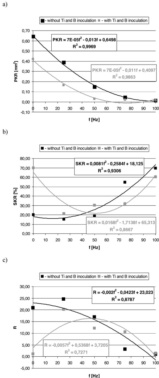
Fig. 5. Influence of frequency (f) of supply current feeding induction coil, which generates electromagnetic field on selected refinement parameters of structure of pure Al ingot
