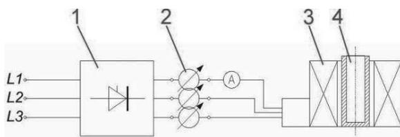
Fig. 2. Scheme of test stand: 1 - inverter, 2 - autotransformer, 3 - induction coil, 4 - mould containing liquid metal, A - ammeter
