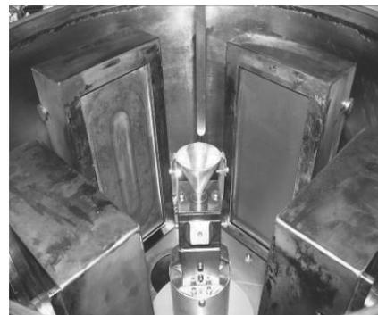
Fig. 1. Internal equipment of a vacuum chamber with four rectangular magnetrons forming a closed magnetic field configuration for magnetron sputtering (CFUBMSIP system) around a rotary heater with specimens
