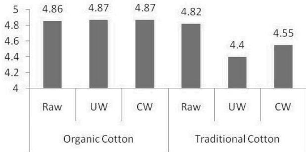
Fig. 4. Raw, ultrasonic and conventional washed yarns elongation properties [%]
