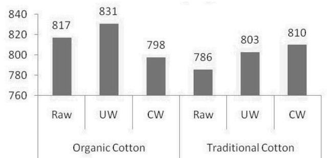
Fig. 2. Raw, ultrasonic and conventional washed yarns twists [T/m]
