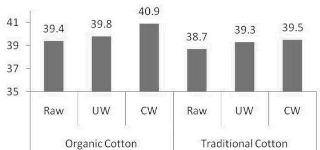
Fig. 1. Raw, ultrasonic and conventional washed yarns counts [Ne]
