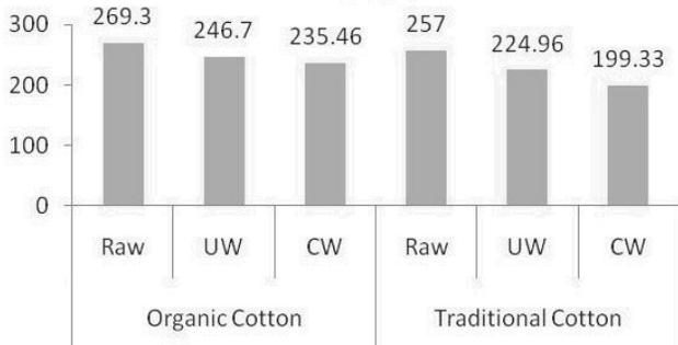
Fig. 3. Raw, ultrasonic and conventional washed yarns tensile strength properties [gf]
