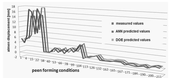
Fig. 5. Measured and predicted maximum displacements
