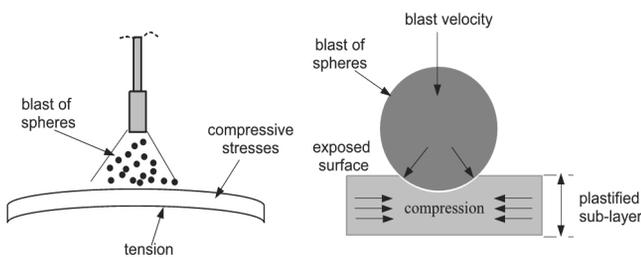
Fig. 1. Peen forming general schema
