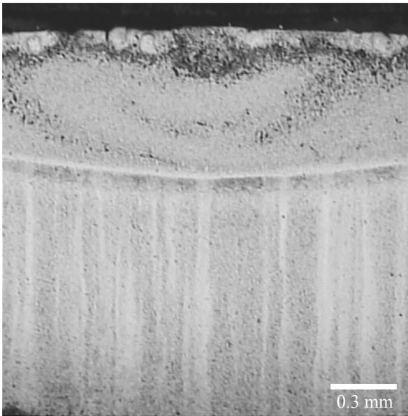
Fig. 27. Melted zone limit of the steel surface layer after alloying with vanadium carbide, laser power of 1.6 kW
