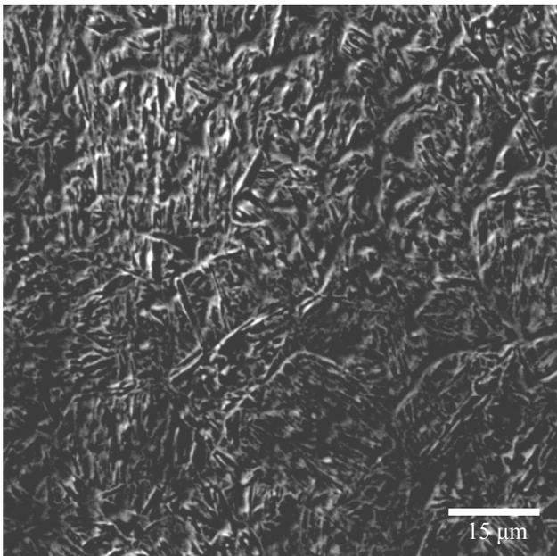
Fig. 31. Surface layer of steel after alloying with vanadium carbide VC powder, the laser beam power of 2.3 kW (SEM)
