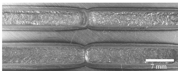
Fig. 18. Face view after laser alloying with vanadium carbide, 32CrMoV12-28 steel, laser power of 1.2-2.3 kW
