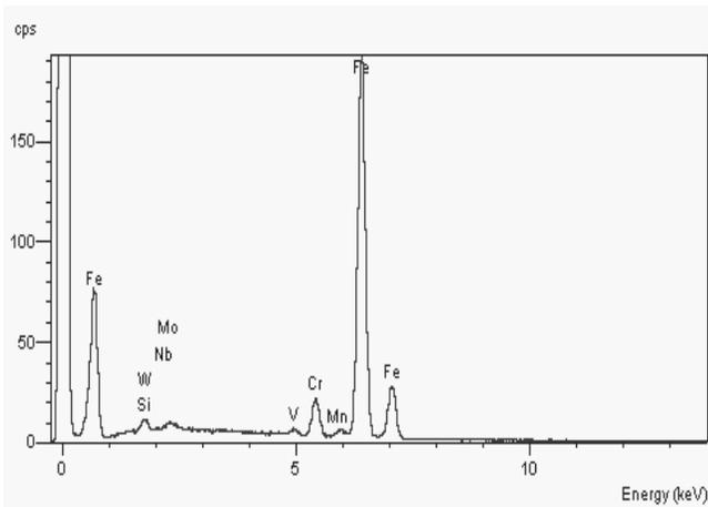
Fig. 36. Diagram of concentration according to scattered X-ray radiation energy for a X40CrMoV5-1 steel sample after cladding with laser, the laser beam power of 1.2 kW
