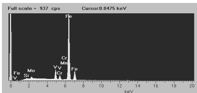
Fig. 32. Diagram of concentration according to energy for the dispersed X-ray radiation for the sample of 32CrMoV12-28 steel after laser alloying with VC vanadium powder
