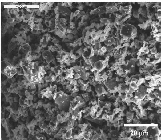
Fig. 4. Topography of titanium carbide powder (TiC) used for the tests (SEM)
