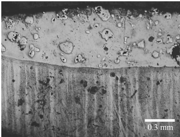
Fig. 21. View of surface layer section after laser alloying of X40CrMoV5-1 steel, tungsten carbide powder, laser power of 2.3 kW
