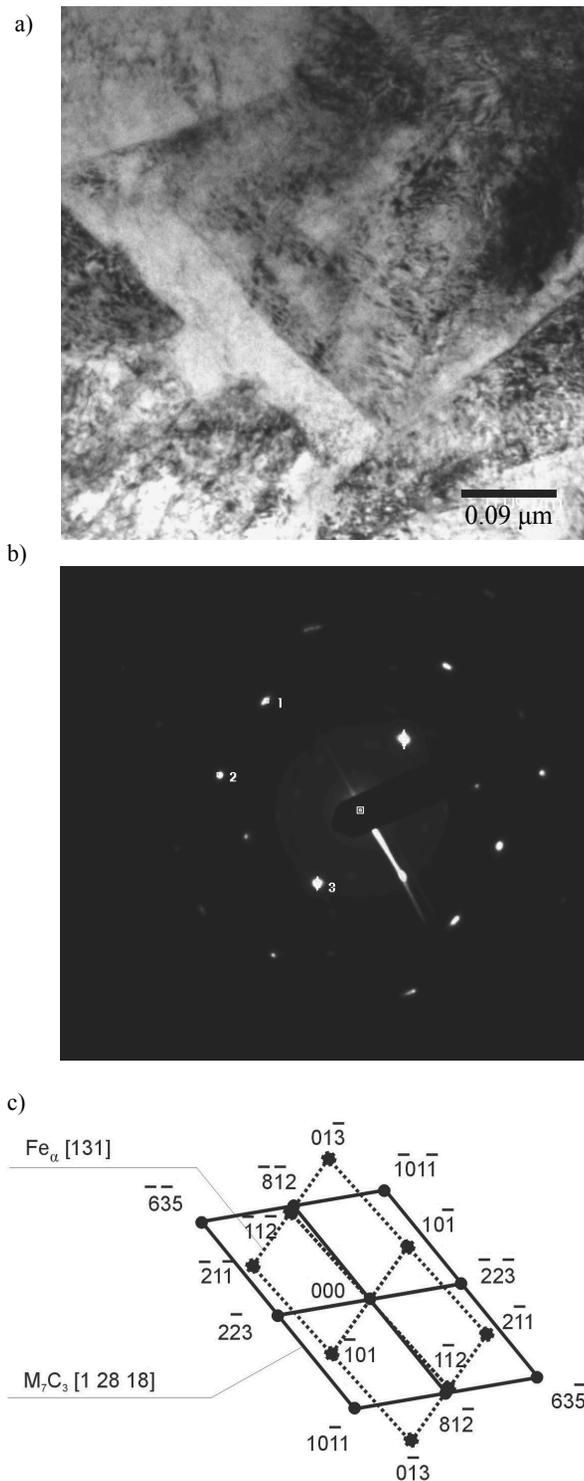
Fig. 38. Structure of thin foil made of X40CrMoV5-1 steel after alloying with NbC niobium carbide, laser beam power of 2.0 kW, a) image in light field, b) diffraction pattern from the area as in figure a), c) diffraction pattern solution for figure b)
