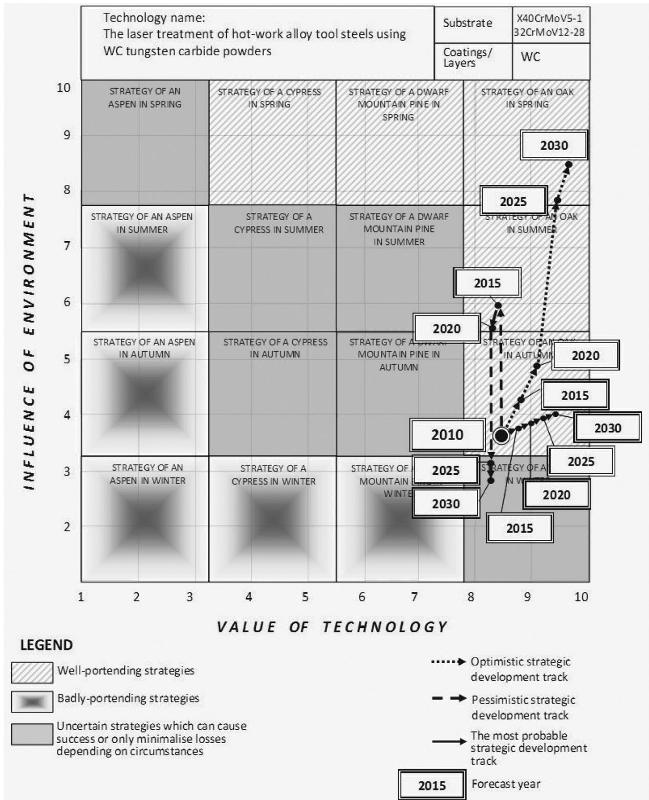
Fig. 8. The strategic development tracks for the (E) demonstration technology called the laser treatment of hot-work alloy tool steels using WC tungsten carbide powders
