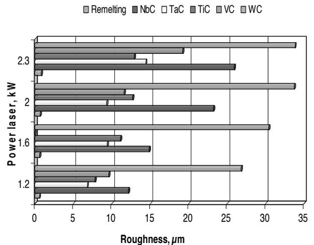
Fig. 20. Average roughness of surface layer for 32CrMoV12-28 remelted with laser or alloyed with carbide powders with a 1.2-2.3 kW laser
