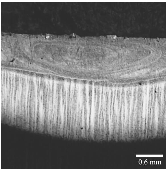
Fig. 28. Melted zone limit of the steel surface layer after alloying with titanium carbide, laser power of 2.0 kW
