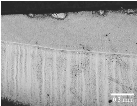
Fig. 22. View of surface layer section after laser alloying, X40CrMoV5-1 steel, vanadium carbide powder, laser power of 2.0 kW
