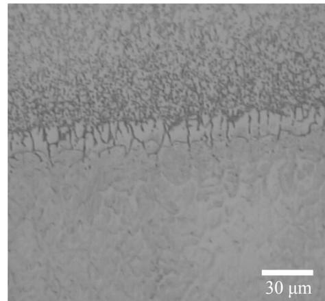
Fig. 25. Melted zone limit of X40CrMoV5-1 steel surface layer, after alloying with titanium carbide, laser power of 2.3 kW
