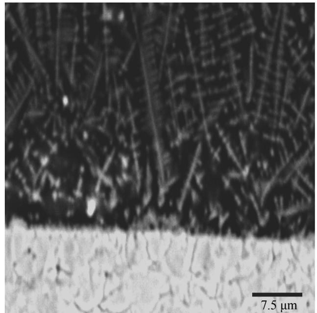
Fig. 33. Surface layer of 32CrMoV12-28 steel after alloying with VC powder, the laser beam power of 2.3 kW
