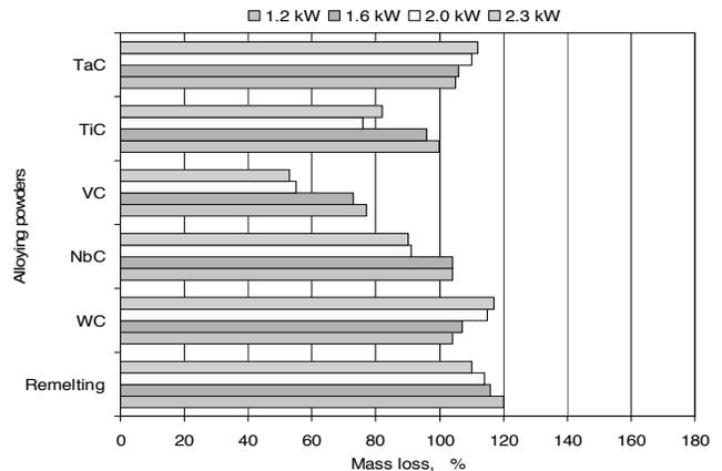
Fig. 44. The relative mass loss measured when testing wear resistance for 32CrMoV12-28 steel (100% – the mass loss of the heat-treated sample, not subjected to laser cladding or alloying with carbide powders)
