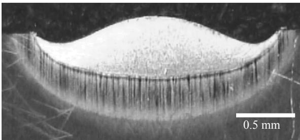
Fig. 11. Surface layer of X40CrMoV5-1 steel after laser alloying with tantalum carbide, laser power of 2.3 kW
