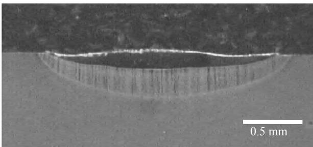
Fig. 12. Surface layer of 32CrMoV12-28 steel after laser alloying with tungsten carbide, laser power of 2.0 kW
