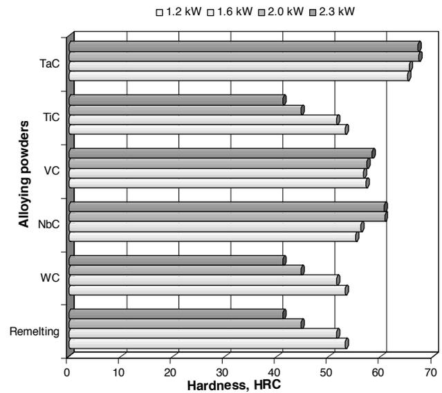
Fig. 40. Variation in surface layer hardness of 32CrMoV12-28 steel remelted or alloyed with the laser power range of 1.2-2.3 kW
