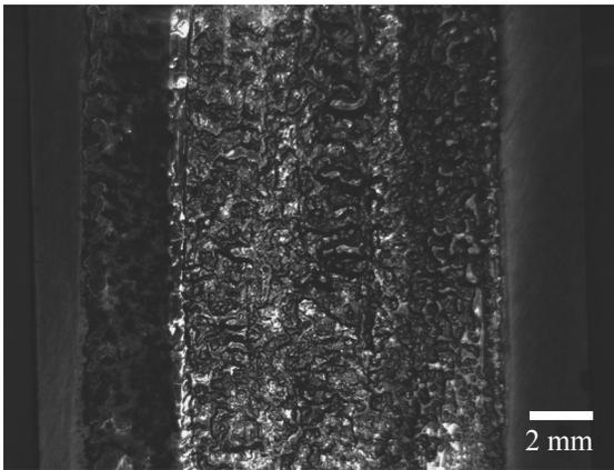
Fig. 41. Wear trace of the surface layer after an abrasion test acc. to ASTM G65 for X40CrMoV5-1 steel alloyed with WC tungsten powder, the laser power of 1.2 kW
