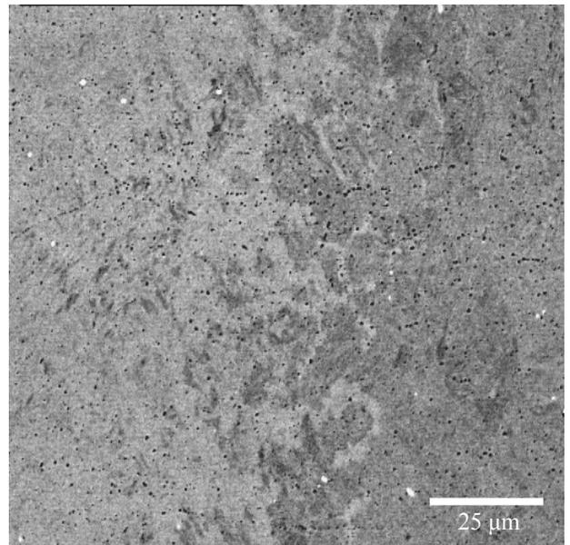
Fig. 30. Zonal structure of the surface layer of X40CrMo5-1 steel remelted with laser, the laser beam power of 1.2 kW
