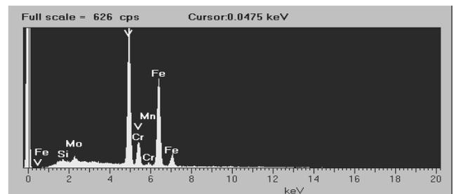
Fig. 34. Diagram of concentration according to scattered X-ray radiation energy for a 32CrMoV12-28 steel sample after laser alloying with VC vanadium powder
