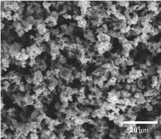
Fig. 3. Topography of vanadium carbide powder (VC) used for the tests (SEM)
