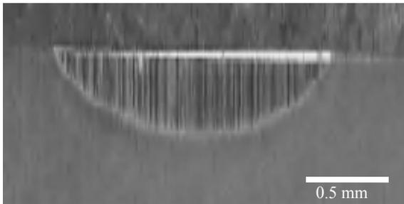
Fig. 10. Surface layer of 32CrMoV12-28 steel after laser cladding, laser power of 1.2 kW
