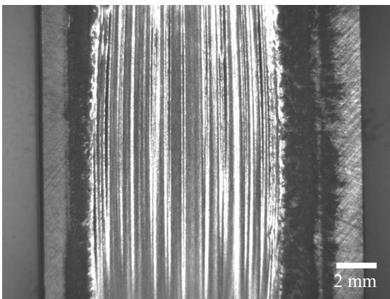
Fig. 42. Wear trace of the surface layer after an abrasion test acc. to ASTM G65 for 32CrMoV12-28 steel alloyed with TiC titanium powder, the laser power of 2.0 kW
