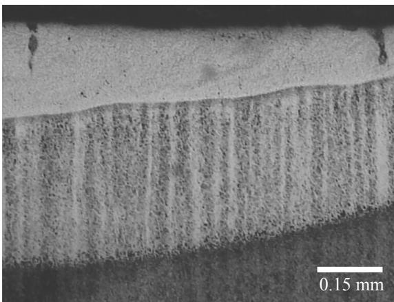
Fig. 23. View of surface layer section after laser alloying, 32CrMoV12-28 steel, vanadium carbide powder, laser power of 1.2 kW
