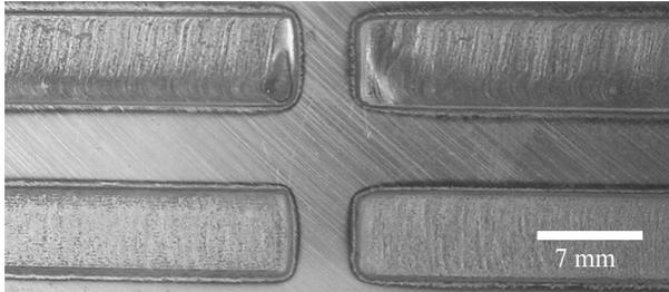
Fig. 15. Face view after laser cladding, X40CrMoV5-1 steel, laser power of 1.2-2.3 kW
