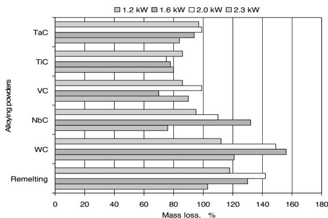
Fig. 43. The relative mass loss measured when testing wear resistance for X40CrMoV5-1 steel (100% – the mass loss of the heat-treated sample, not subjected to laser cladding or alloying with carbide powders)
