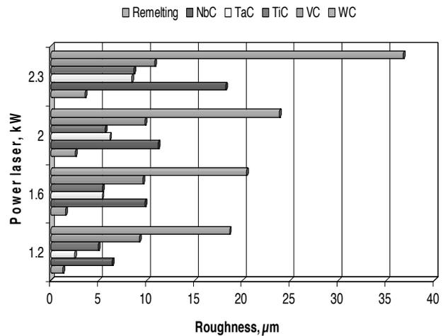
Fig. 19. Average roughness of surface layer for X40CrMoV5-1 steel remelted with laser or alloyed with carbide powders with a 1.2-2.3 kW laser
