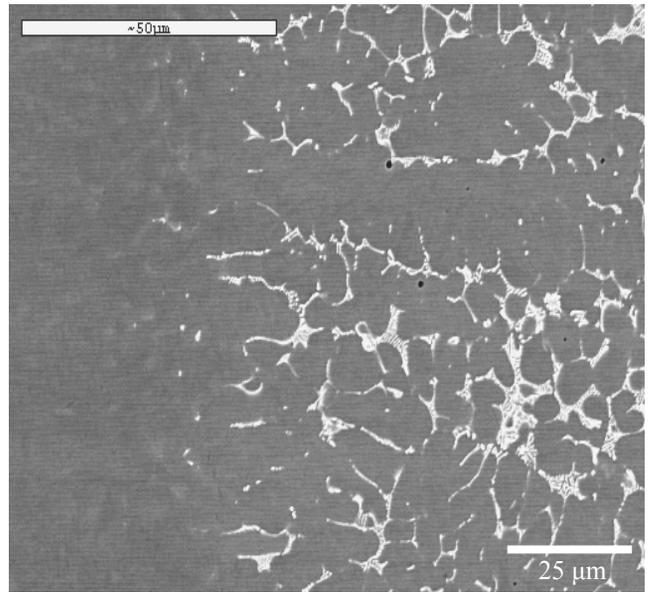
Fig. 29. Zonal structure of the surface layer of X40CrMo5-1 steel alloyed with TaC powder, the laser beam power of 1.6 kW
