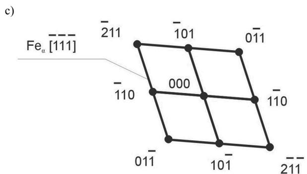
Fig. 37. Structure of thin foil made of 32CrMoV12-28 steel after alloying with VC vanadium carbide with the following parameters: scanning speed – 0.5 m/min, beam power – 2.0 kW, a) image in light field, b) diffraction pattern from the area as in figure a), c) diffraction pattern solution for figure b)
