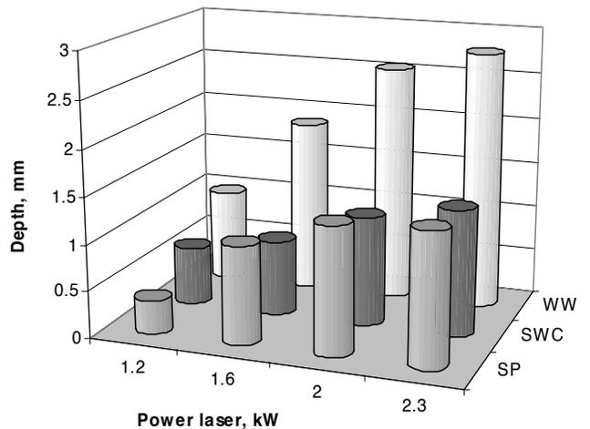
Fig. 14. The effect of laser power on the thickness of RZ and HAZ of 32CrMoV12-28 steel after laser alloying with TaC within the laser power of 1.2-2.3 kW
