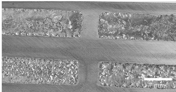
Fig. 16. Face view after laser alloying with tungsten carbide, X40CrMoV5-1 steel, laser power of 1.2-2.3 kW
