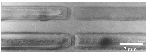
Fig. 17. Face view after laser cladding, 32CrMoV12-28 steel, laser power of 1.2-2.3 kW
