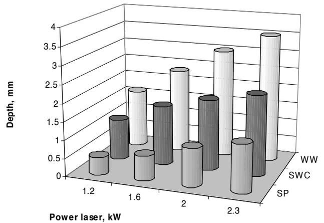
Fig. 13. The effect of laser power on the thickness of RZ and HAZ of X40CrMoV5-1 steel after laser alloying with TaC within the laser power of 1.2-2.3 kW
