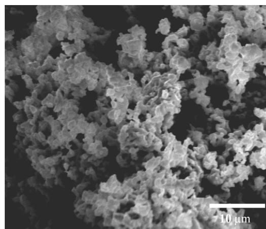
Fig. 2. Topography of niobium carbide powder (NbC) used for the tests (SEM)
