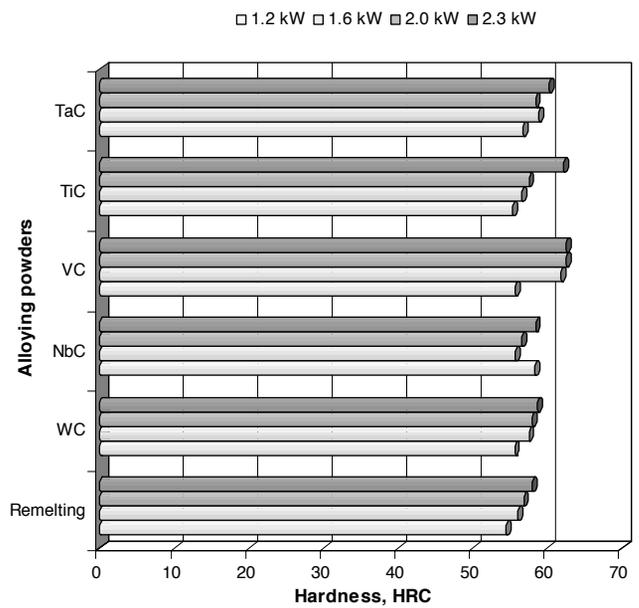
Fig. 39. Variation in surface layer hardness of X40CrMoV5-1 steel remelted or alloyed with the laser power range of 1.2-2.3 kW
