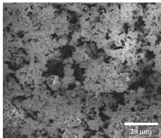
Fig. 1. Topography of tantalum carbide powder (TaC) used for the tests (SEM)
