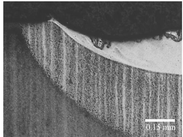
Fig. 24. View of surface layer section after laser alloying, 32CrMoV12-28 steel, vanadium carbide powder, laser power of 2.3 kW
