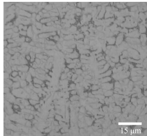
Fig. 26. Central zone of remelted surface layer of X40CrMoV5-1 steel after remelting, laser power of 2.3 kW
