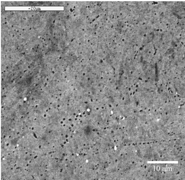
Fig. 35. Central zone of cladding the surface layer of X40CrMoV5-1 steel sample after cladding with laser, the laser beam power of 1.2 kW
