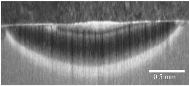
Fig. 9. Surface layer of X40CrMoV5-1 steel after laser cladding, laser power of 1.2 kW
