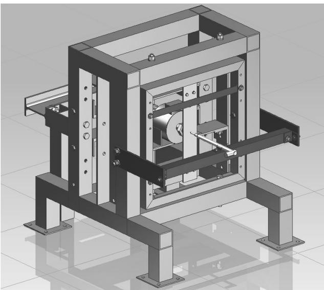
Fig. 5. Three - point bending position
