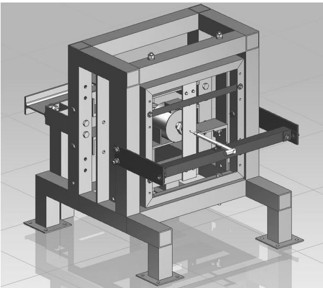
Fig. 5. Three - point bending position
