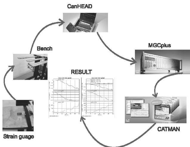
Fig. 2. Measurement chain
