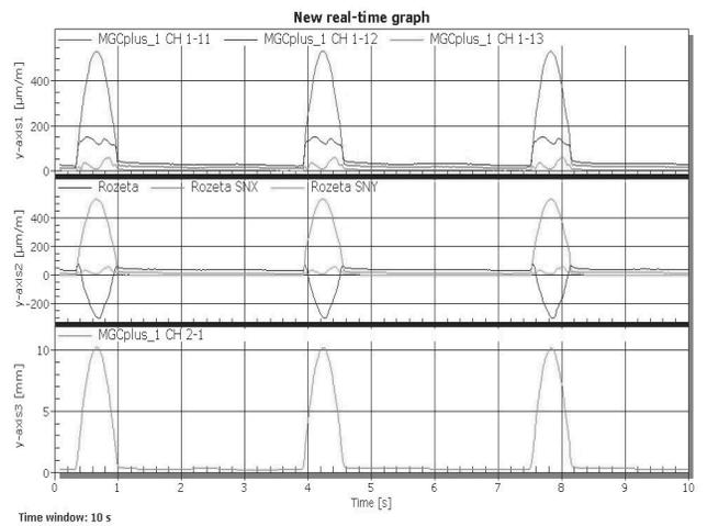
Fig. 16. The graph shows the deformation of a composite sample of glass fiber, plain weave, which was founded 10 mm displacement and 18 rpm
