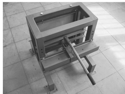
Fig. 7. Research position for axial loading laminate panels
