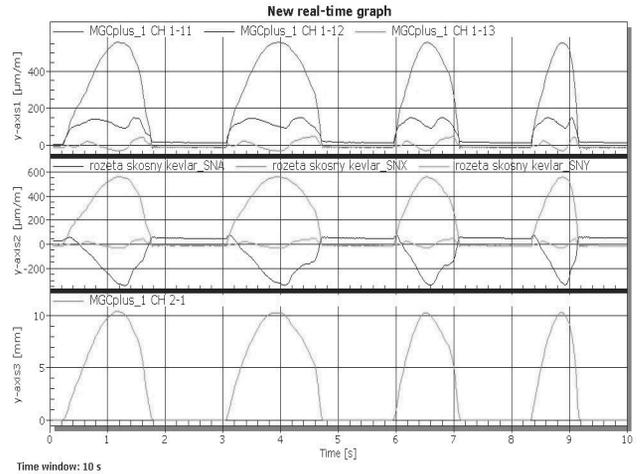
Fig. 15. The graph shows the deformation of a composite sample of glass fiber, plain weave, founded 10 mm displacement
