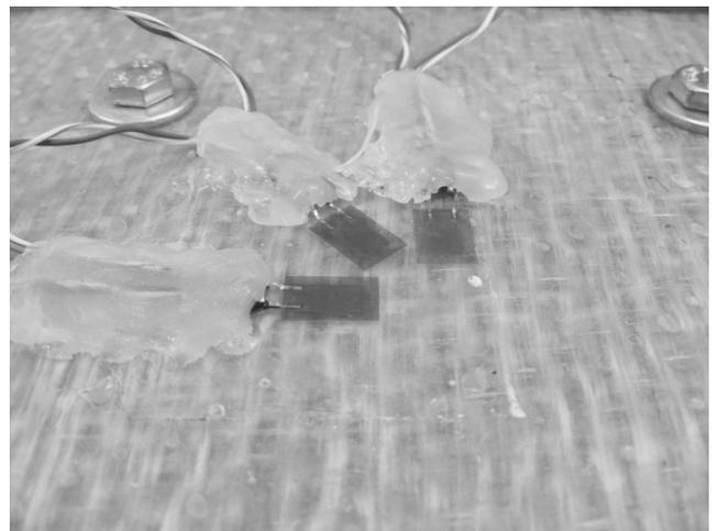
Fig. 3. Strain gauges on a surface
