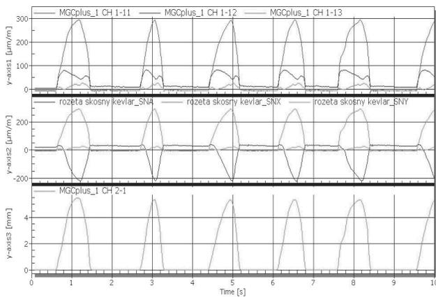
Fig. 14. The graph shows the deformation of a composite sample of glass fiber, plain weave, founded 5 mm displacement
