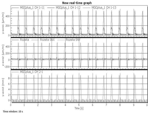
Fig. 17. The graph shows the deformation of a composite sample of glass fiber, plain weave, which was founded 10 mm displacement and 102 rpm
