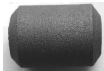
Fig. 6. A view of the NiAl(Cr) – Al<sub>2</sub>O<sub>3</sub> coating surface, magn. 2x
