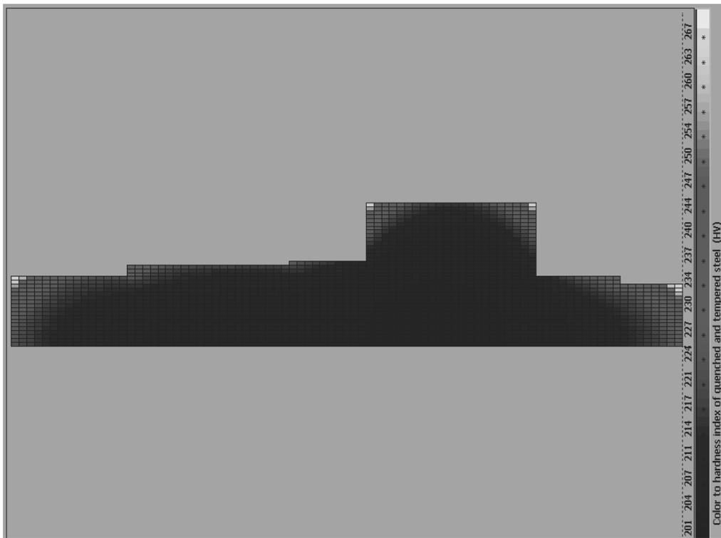
Fig. 4. Distributions of hardness of quenched and tempered workpiece
