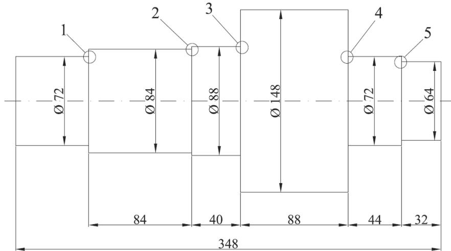
Fig. 1. Geometry of steel shaft
