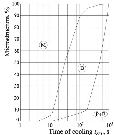
Fig. 2. Microstructure compositions vs. time  $t_{8/5}$ ; (P+F) - Pearlite + Ferrite; B - Bainite; M - Martensite
