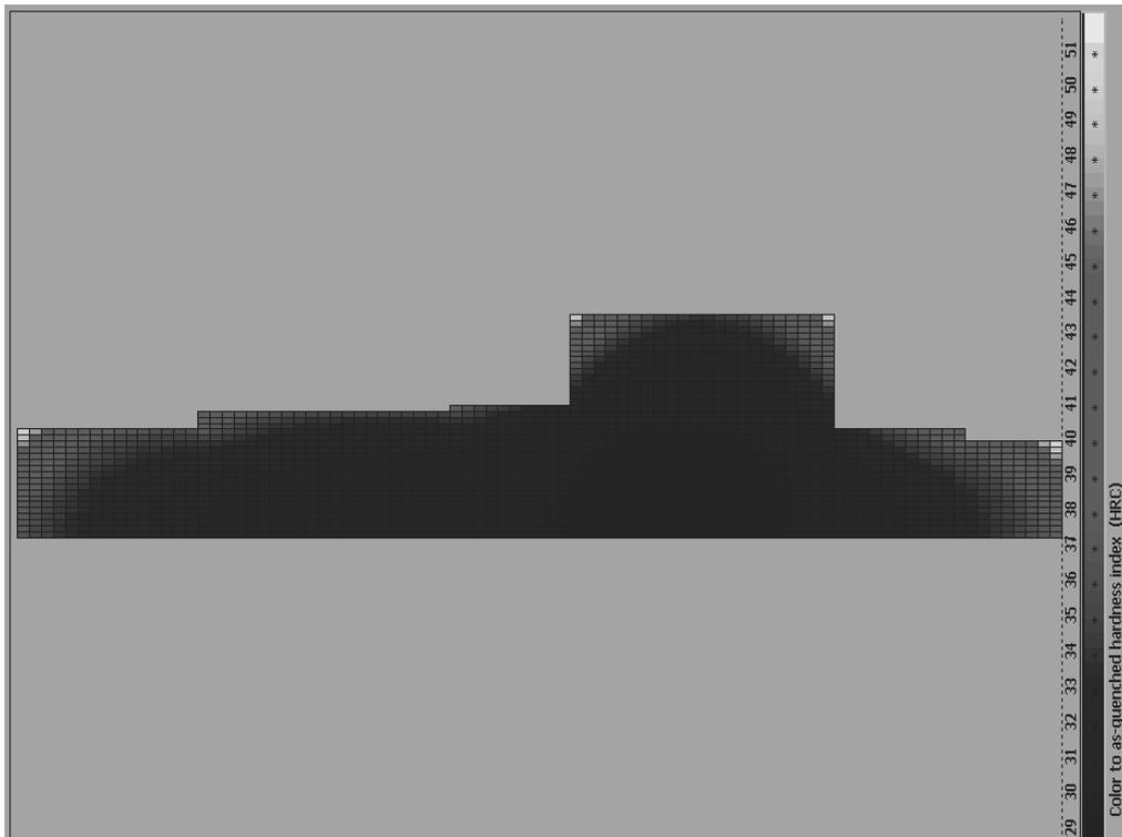
Fig. 3. Distributions of hardness of as-quenched workpiece
