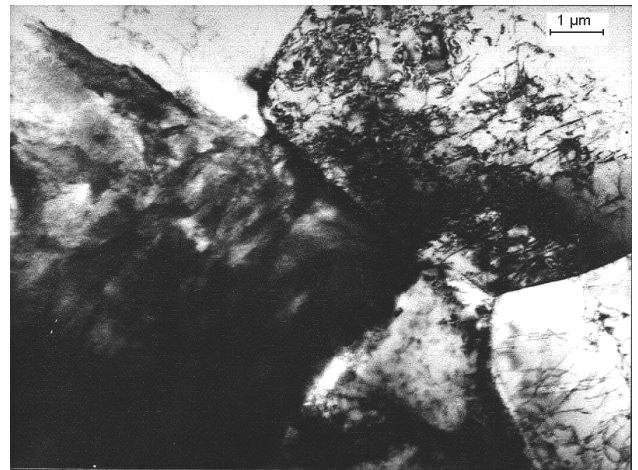
Fig. 47. Martensitic island on the boundaries of three ferrite grains of high dislocation density
